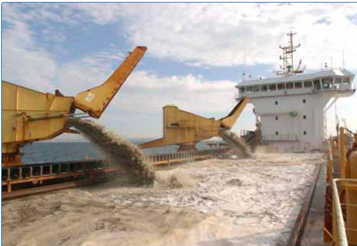
**Offshore aggregate gravel extraction**
