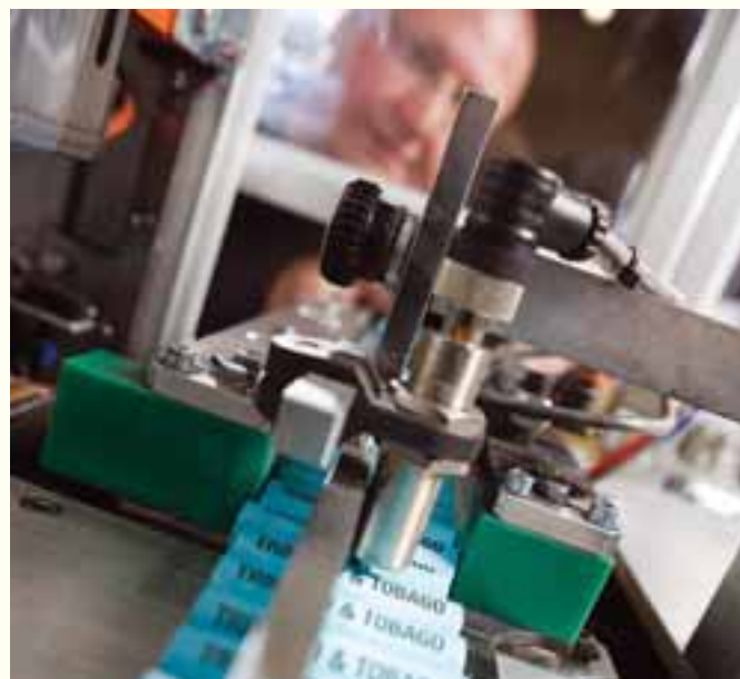
For despatch, a number of countries prefer their coins to be wrapped in paper tubes and the Royal Mint has invested in a dedicated machine to pack coins according to this requirement.
