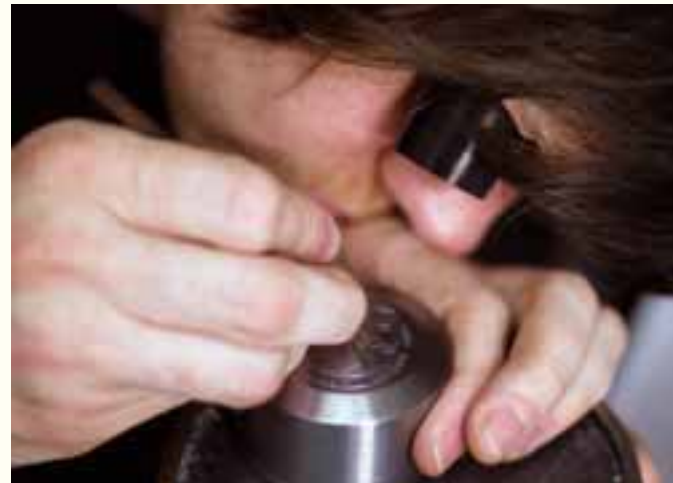
Traditional skills, such as engraving direct into steel, remain fundamental to the preparation of high-quality modern coins and medals.
