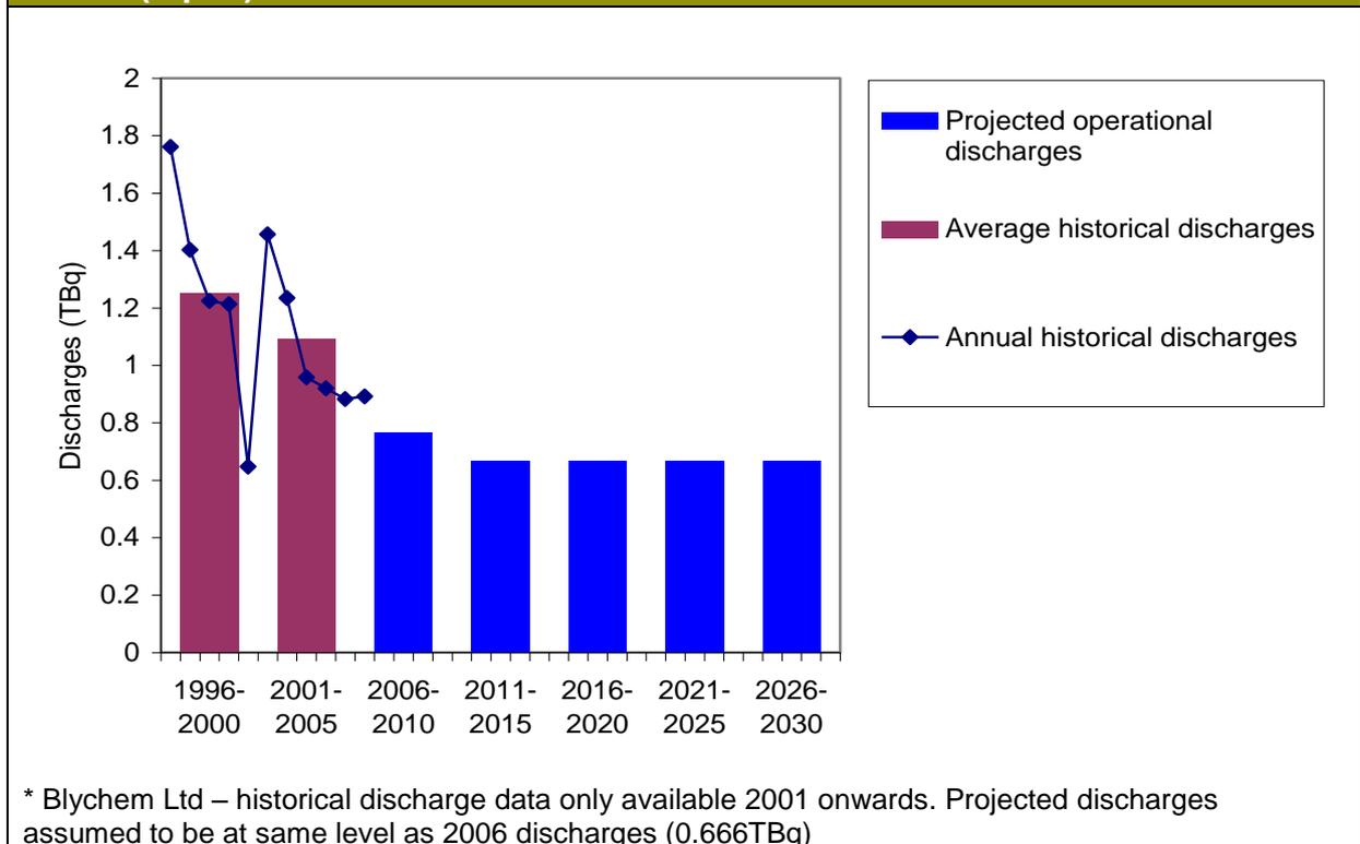
**Figure 12.3: H-3 discharges from isotope production & radio-labelling sector (liquid)**
