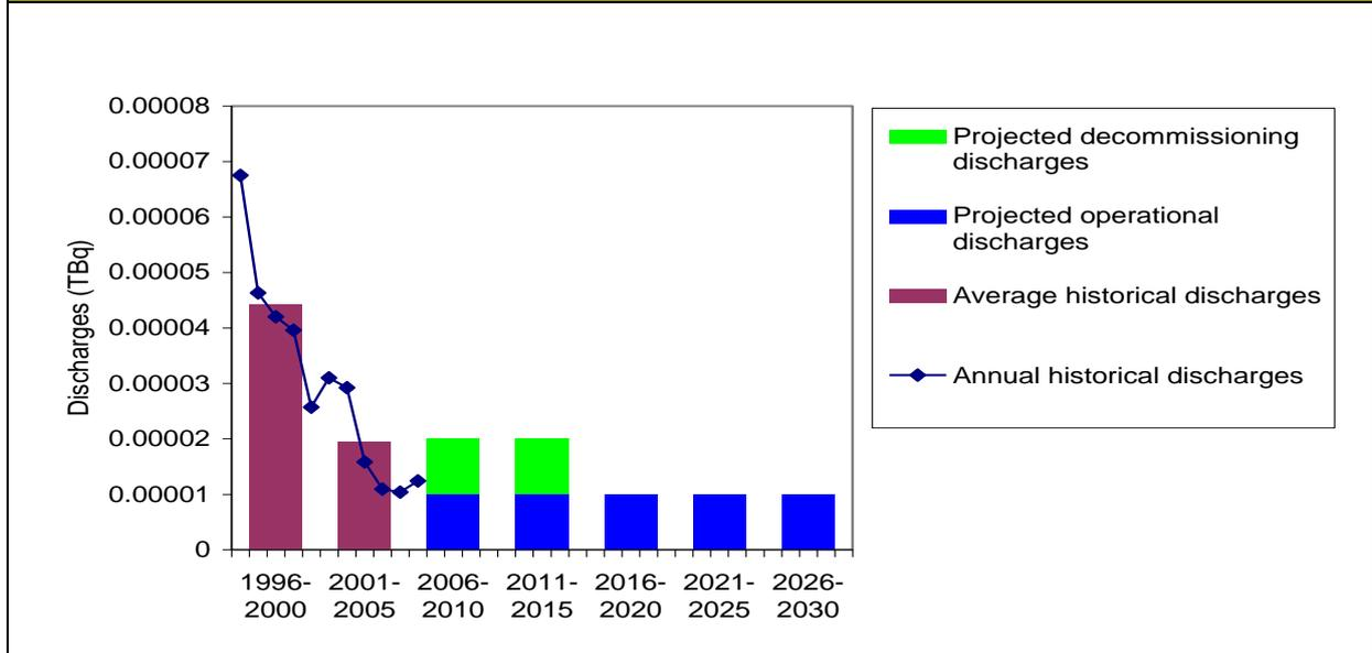
**Figure 12.2: Total beta discharges from isotope production & radio-labelling sector (liquid)**
