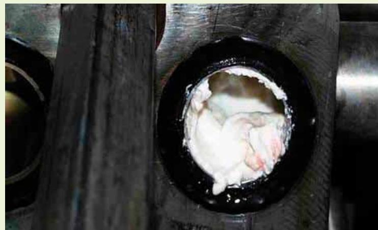
A fouled plate heat exchanger, showing a port clogged with protein deposit.
