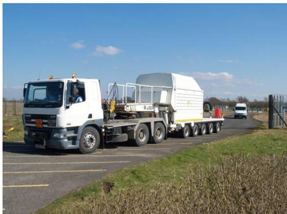
Following significant modifications to the Chapelcross defuelling system, the site is now able to fill and despatch fuel flasks at a rate of up to three flasks per week (pictured – flask in
