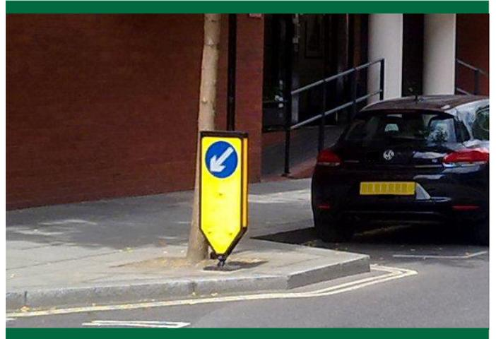
*Figure 14: Incorrect use of a keep left sign*
