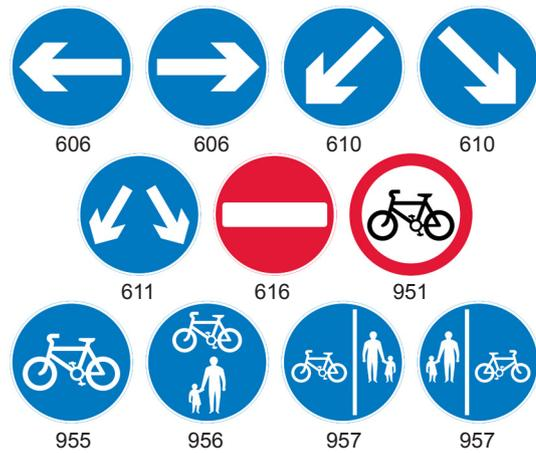
Figure 2 Signs permitted on a traffic bollard
