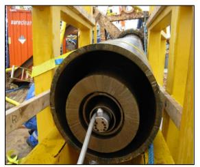
Fig 4- Internal Multi String Cutting Tool
