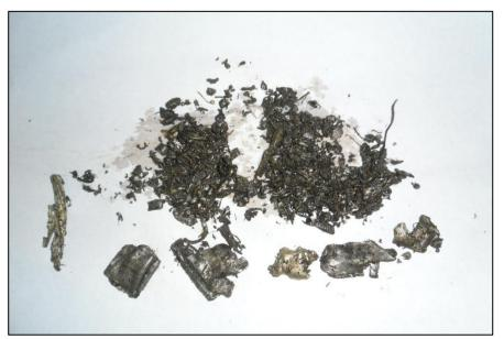
Fig 15- Swarf sample recovered to the vessel
