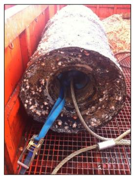
Fig 19- Recovered Wellhead on deck
