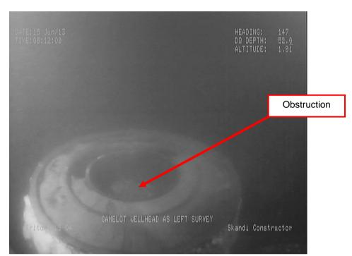
Fig 20- Obstruction in 13 3/8" Casing
