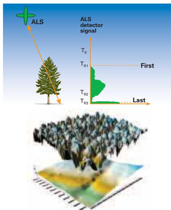
**Figure 1** Interactions between the commercial airborne laser systems (ALS) and the vegetation. First return signal is used to derive canopy models, whereas the last return signal generates high resolution terrain models. Vegetation height is estimated as the difference between the first and the last laser returns (NTCM – normalised tree canopy model).
