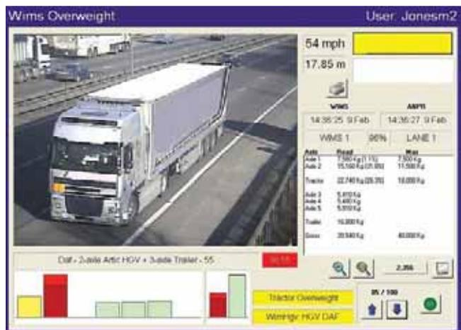
The trial also concluded that combined ANPR and WIMS installations can provide highly focused enforcement targeting.
