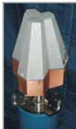
An AGATA detector unit of three germanium crystals
