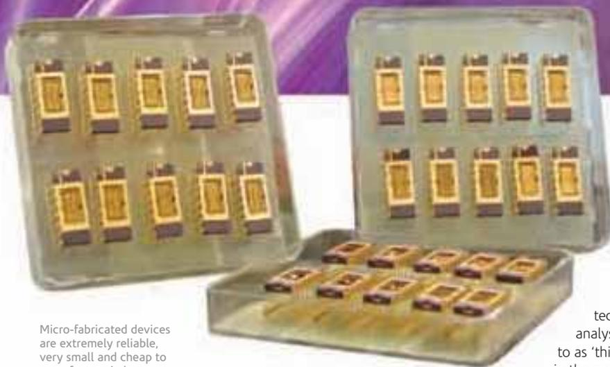
Micro-fabricated devices are extremely reliable, very small and cheap to manufacture in large quantities
