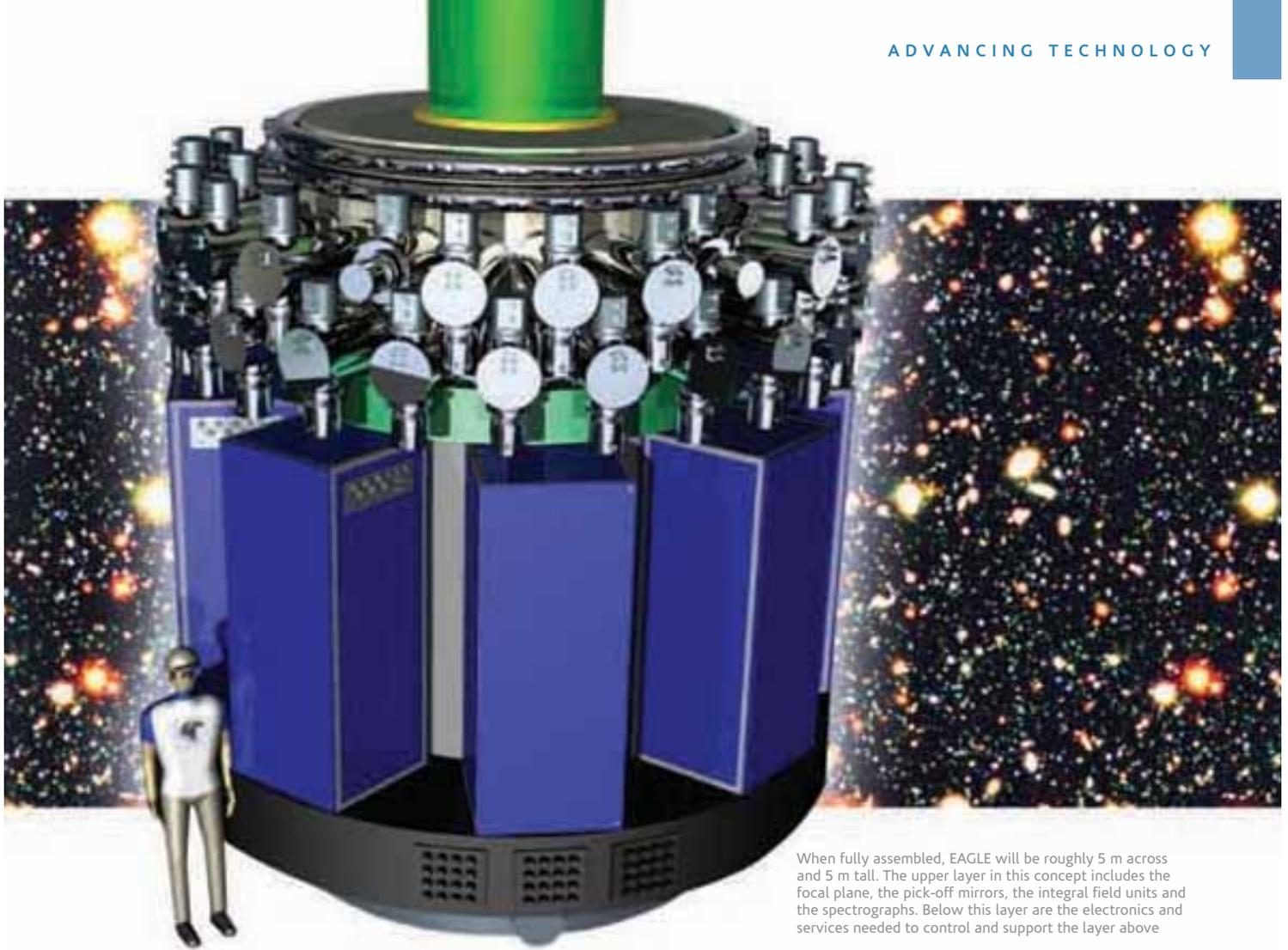
When fully assembled, EAGLE will be roughly 5 m across and 5 m tall. The upper layer in this concept includes the focal plane, the pick-off mirrors, the integral field units and the spectrographs. Below this layer are the electronics and services needed to control and support the layer above
