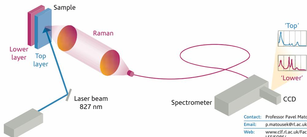
The SORS method is based on a simple concept. Instead of collecting Raman light from the regions of a sample illuminated by the laser beam where the maximum signal is present, the scattered light is collected from regions that are laterally offset. This offset signal contains much lower relative Raman and fluorescence contributions from the surface layer allowing the signals of individual layers to be identified and separated from each other.
