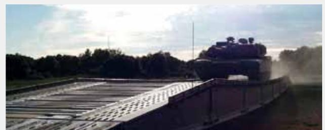
Designed for military operations, the pioneering DSB can span gaps of up to 46 metres in less than 90 minutes and has a maximum load capacity of 120 tonnes.
