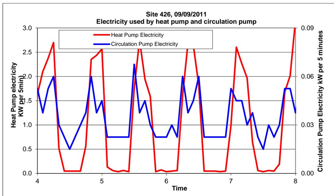
**Figure 53: Electricity consumption of the heat pump and circulation pump at site 426 during a mild day in Phase II**
