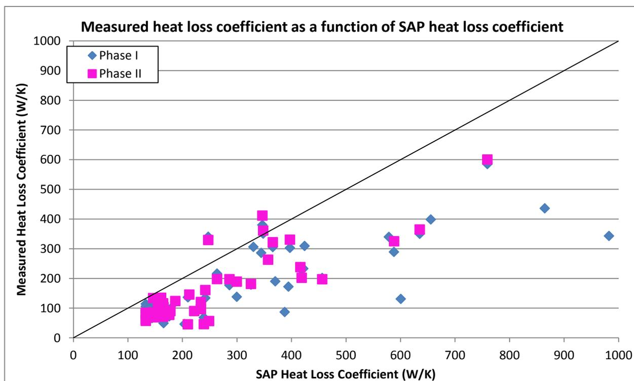
Figure 79: Comparison of measured heat loss coefficients and SAP heat loss coefficients
