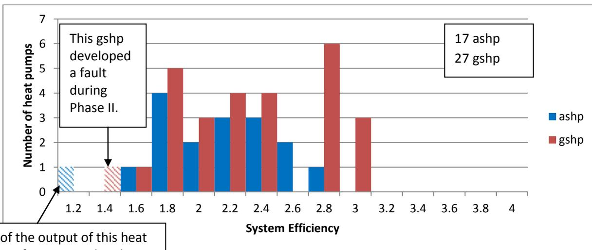
90% of the output of this heat pump is for DHW and tank is poorly insulated.
