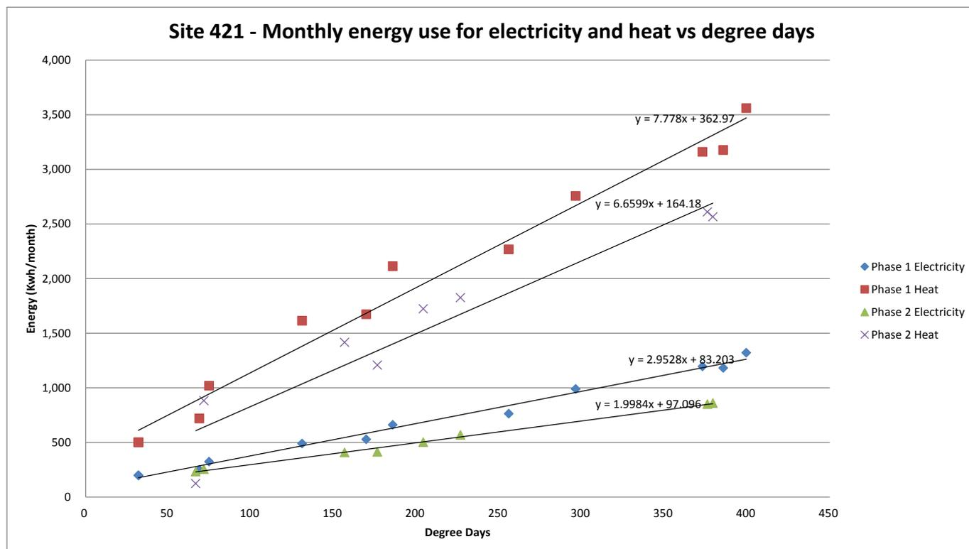
Figure 78: Monthly electricity and heat use plotted against monthly degree days for site 421.
