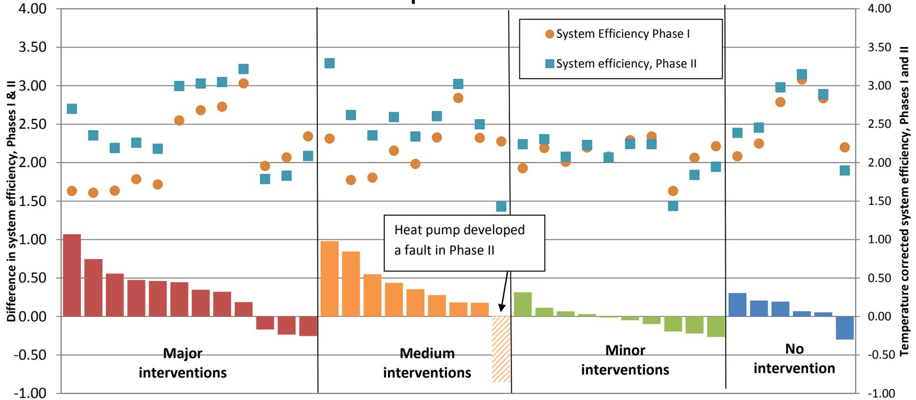
**Figure 9: Change in temperature-corrected system efficiency from Phase I to Phase II (37 sites, one site with faulty heat meter in Phase I removed from minor intervention category)**
