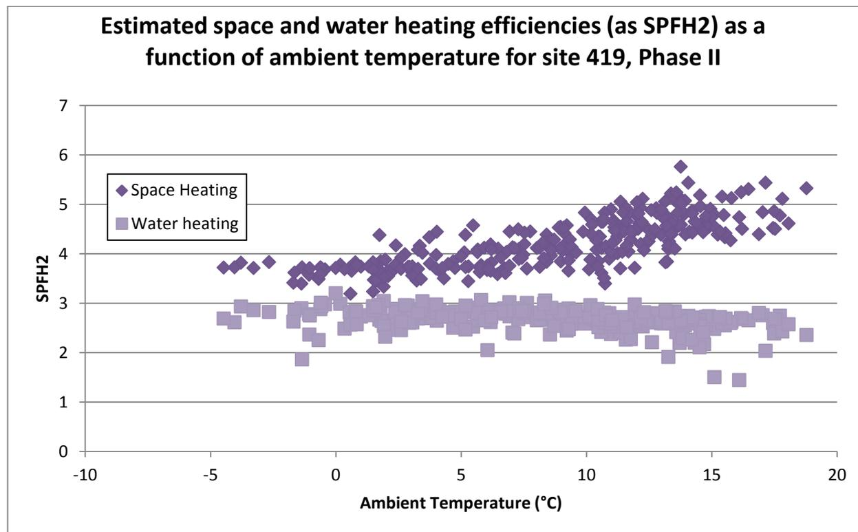
**Figure 38: Estimated space and water heating efficiencies (as  $SPF_{H2}$ ) as a function of ambient temperature for site 419, Phase II**
