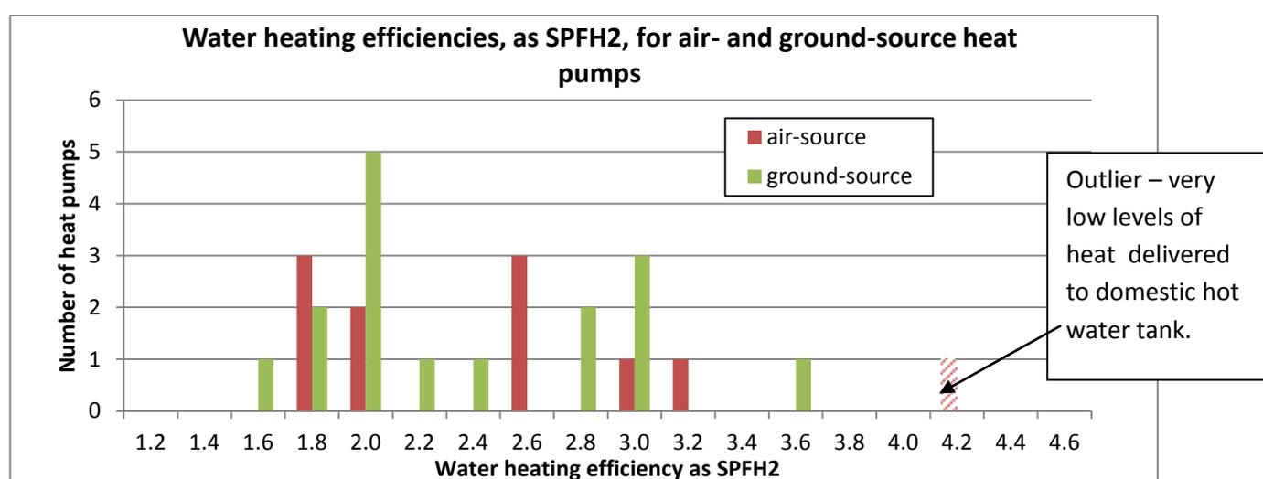
**Figure 19: Water heating efficiencies for 11 air- and 16 ground source heat pumps (as  $SPF_{H2}$ )**
