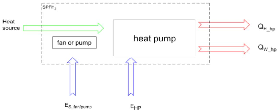
**Figure 3: System boundary for  $SPF_{H2}$ , as defined in the SEPAMO project.**
