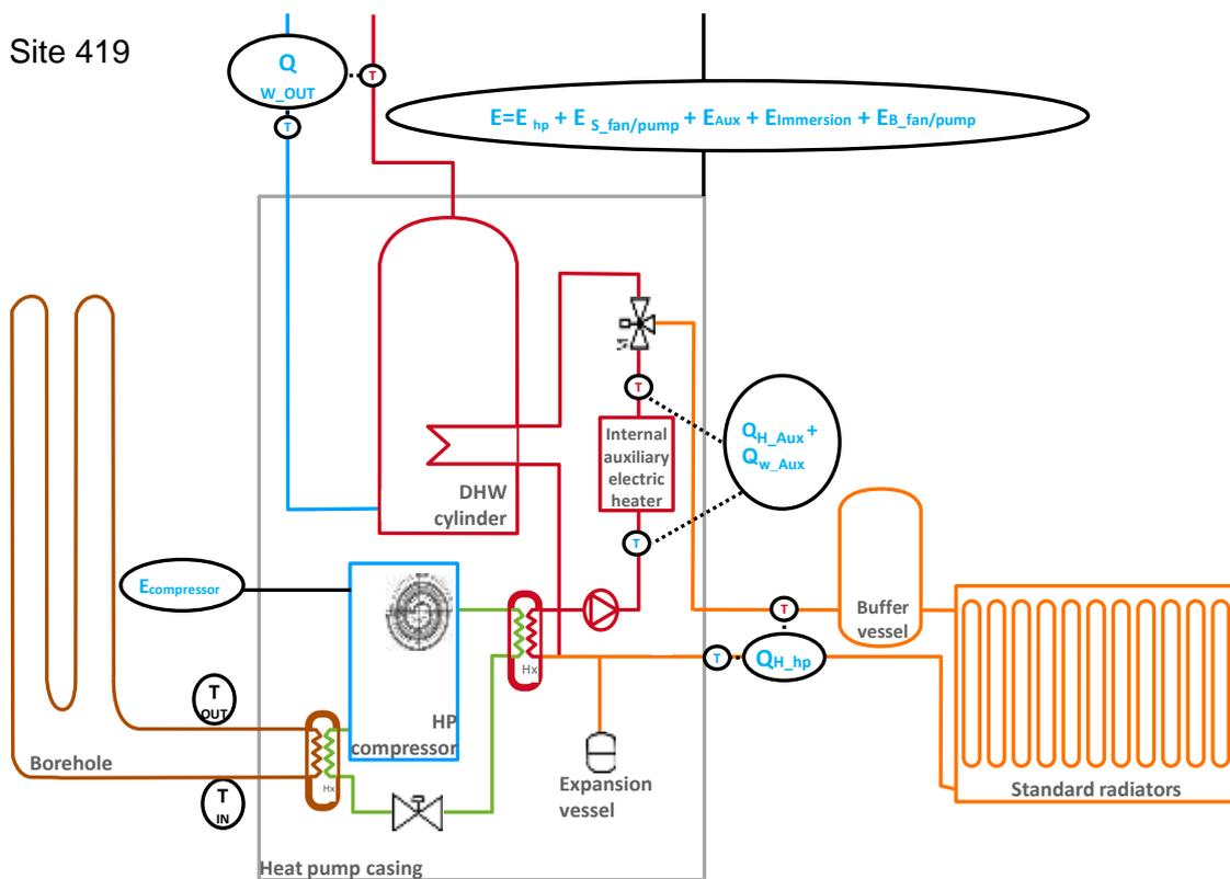
Figure 35: Schematic for site 419, Phase II
