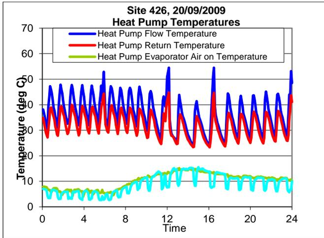
**Figure 45: Heat pump temperatures on 20/09/2009 at site 426 (Phase I)**
