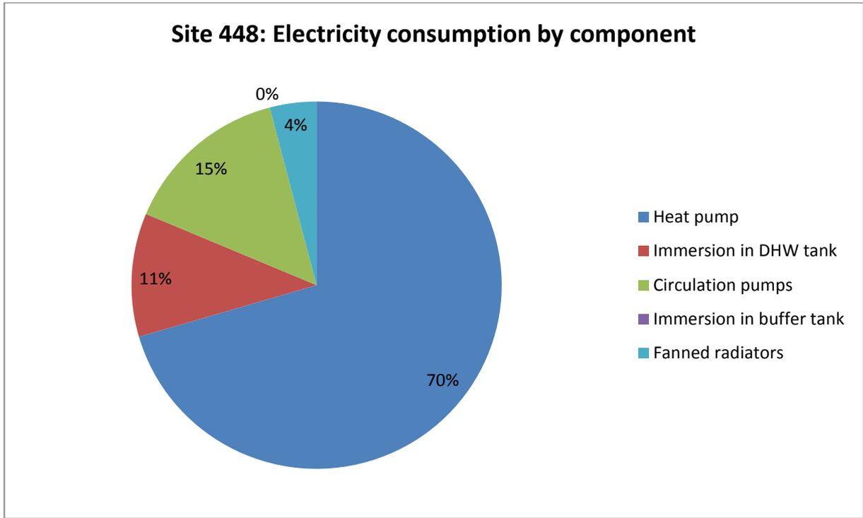
**Figure 71: Electricity consumption by different components for site 448, Phase II**
