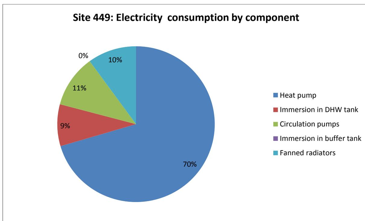
Figure 74: Electricity consumption by different components, site 449, Phase II
