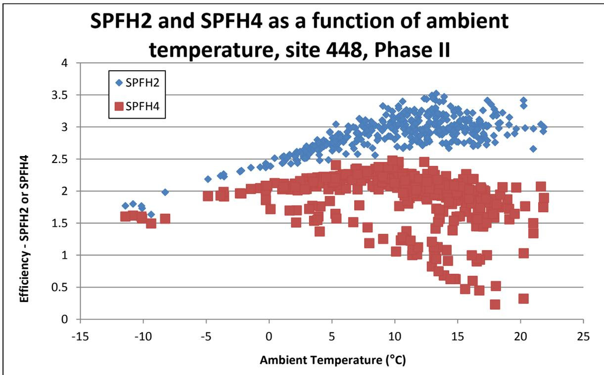
**Figure 72:  $SPF_{H2}$  and  $SPF_{H4}$  as a function of ambient temperature for site 448, Phase II**
