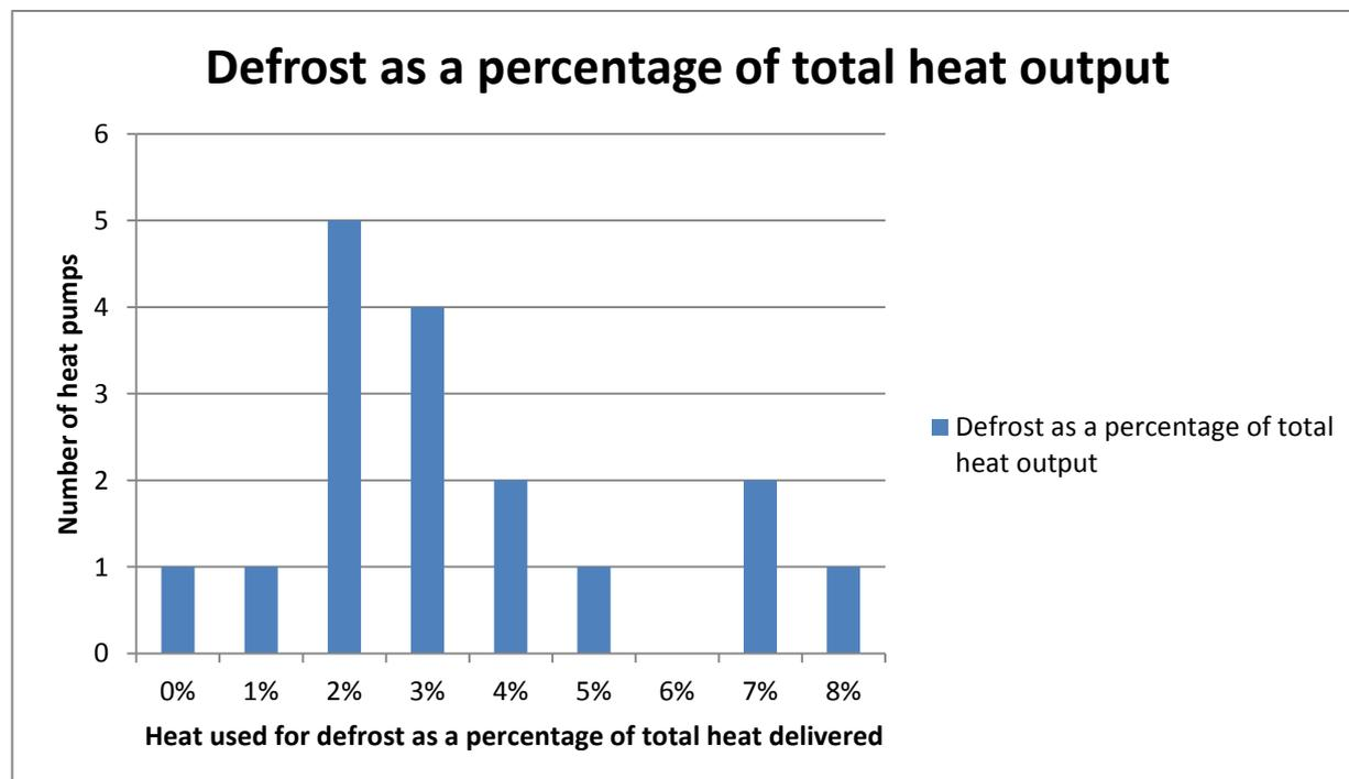
**Figure 12: Defrost as a percentage of total heat output for the air-source heat pumps in the field trial**
