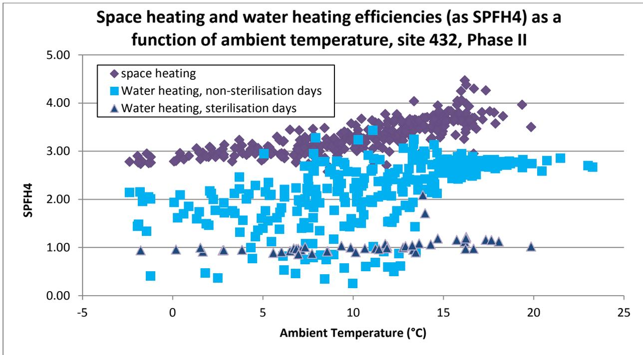
**Figure 62: Space and water heating efficiencies (as  $SPF_{H4}$ ) as a function of ambient temperature, showing effect of sterilisation, site 432, Phase II**
