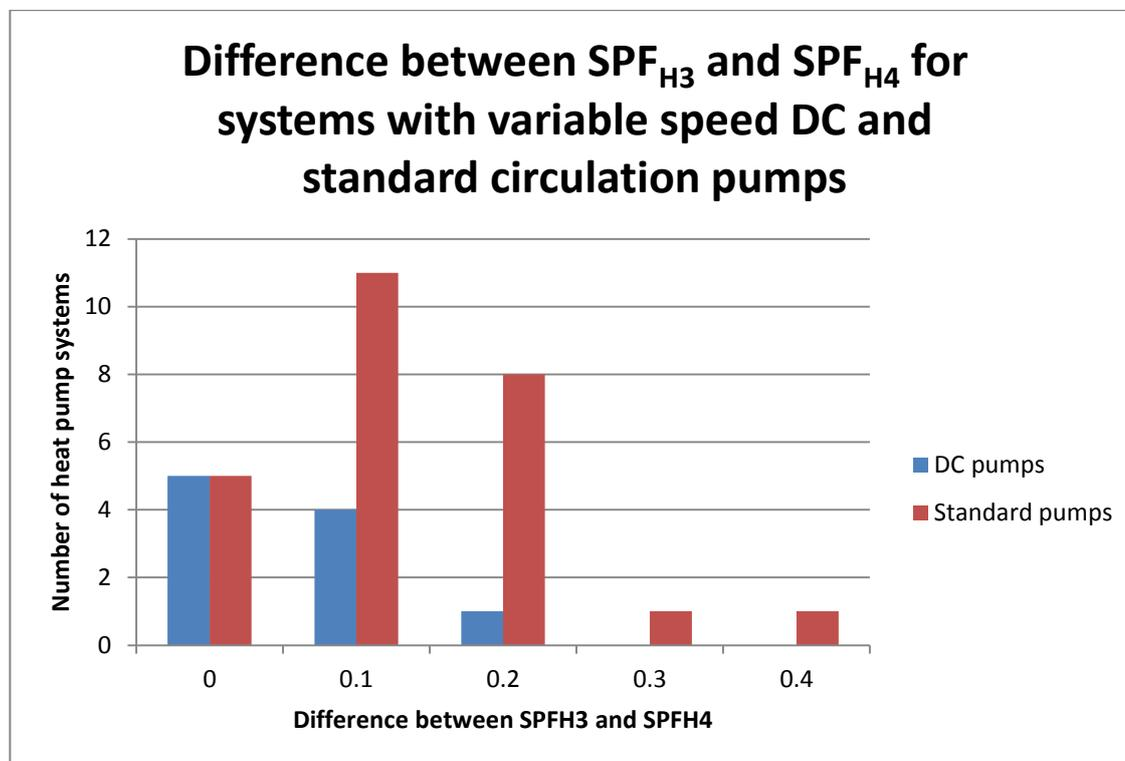
**Figure 10: Difference between  $SPF_{H3}$  and  $SPF_{H4}$  for systems with variable speed DC and standard circulation pumps**
