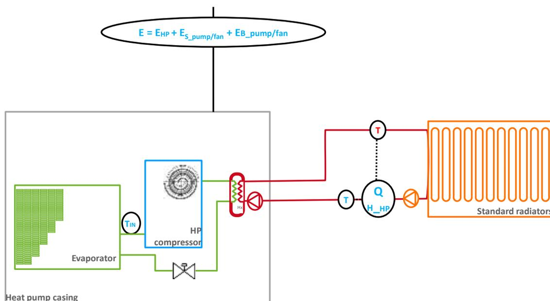
**Figure 66: Schematic for site 443, Phase II**
