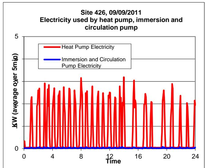
**Figure 52: Electricity consumption, site 426, 09/09/2011, Phase II**
