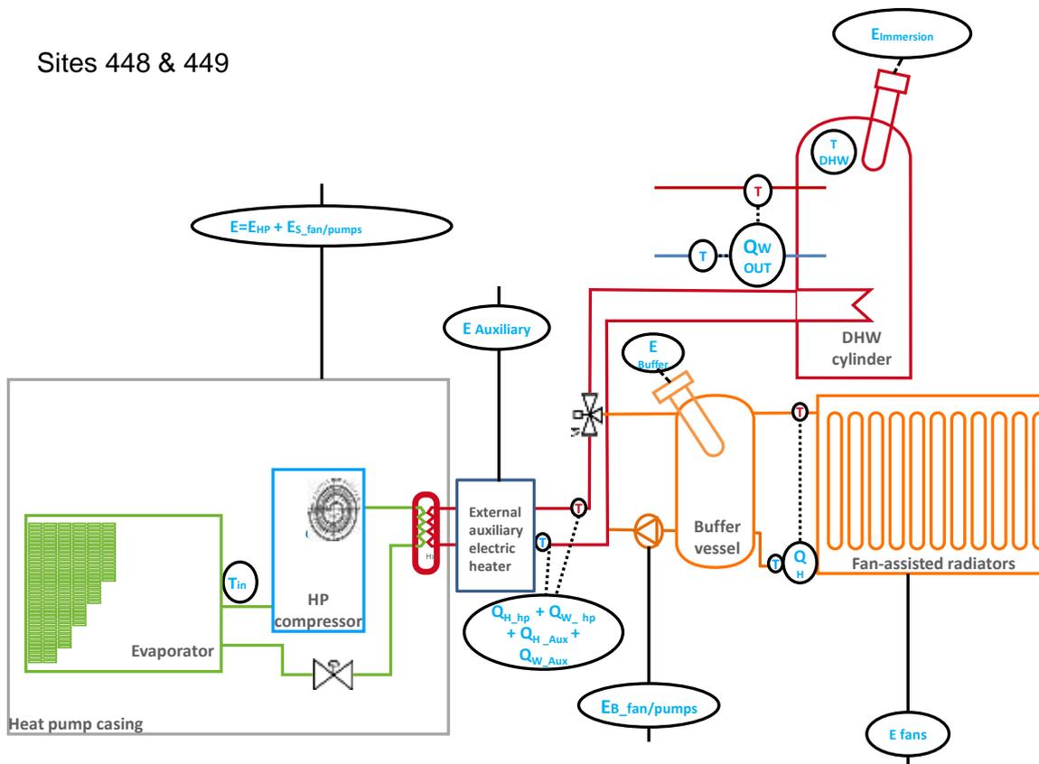
Figure 68: Schematic for site 448, Phase II
