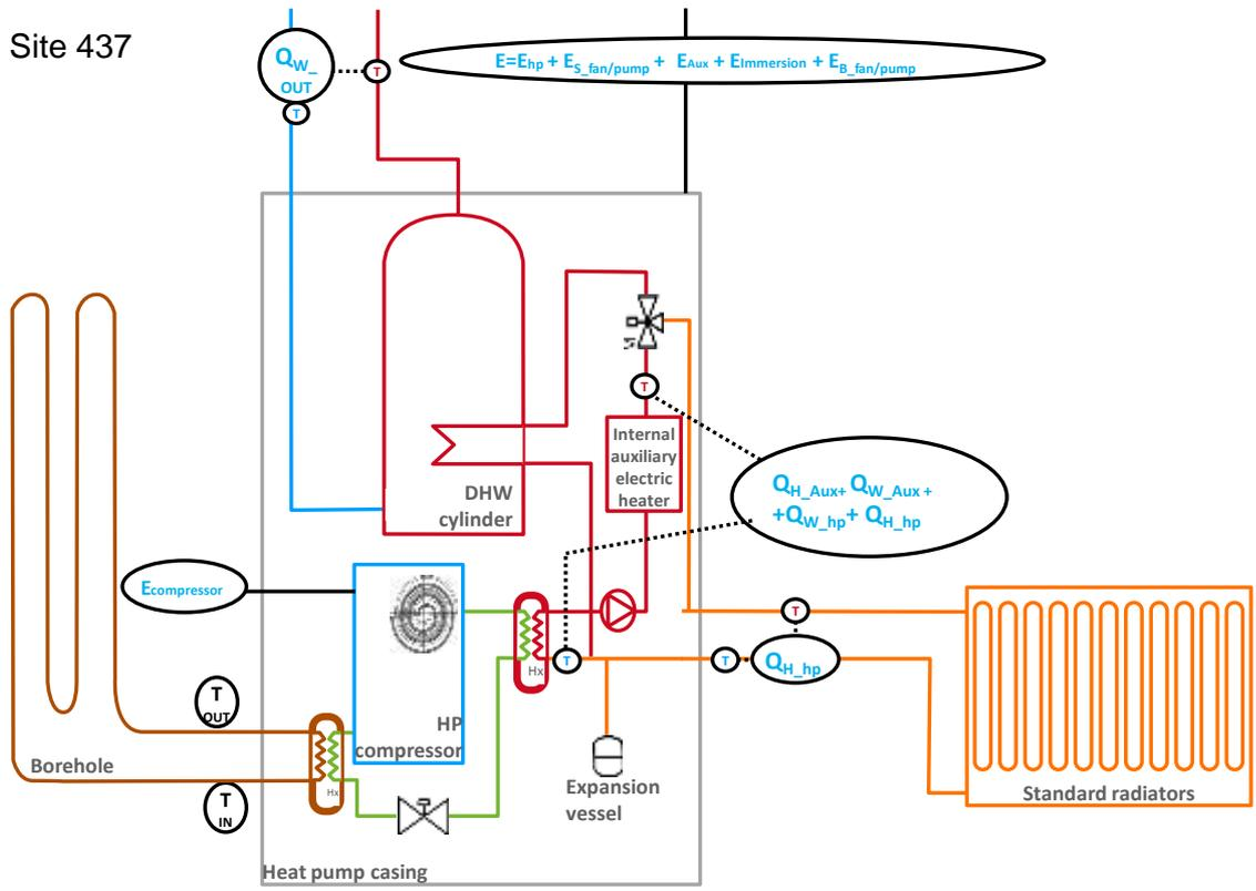
Figure 56 shows the schematic.
