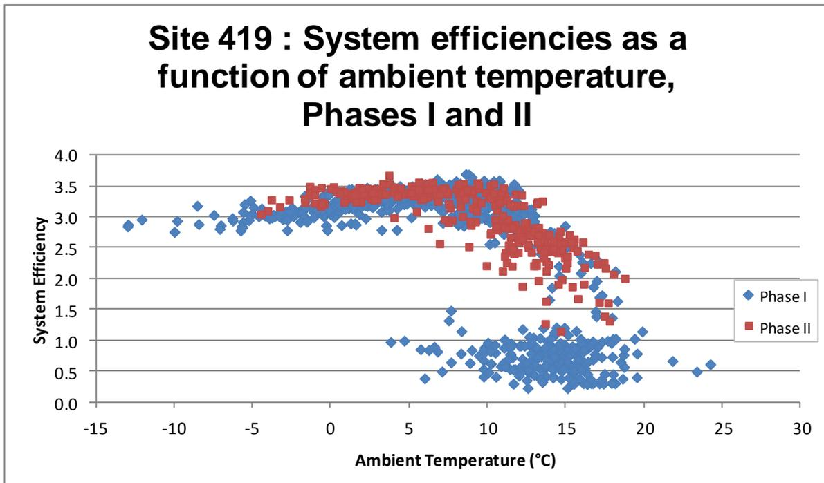
**Figure 37: System efficiencies as a function of ambient temperature for site 419, Phases I & II**
