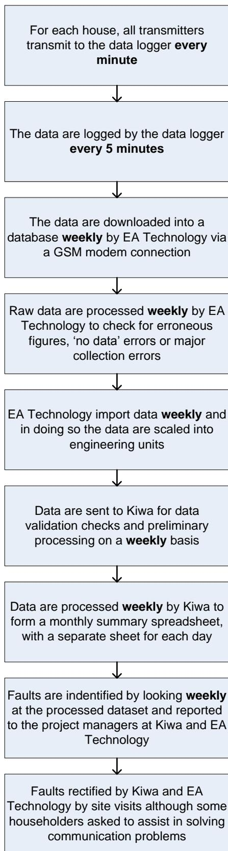
Figure 77: Flow chart showing procedures for data checking
