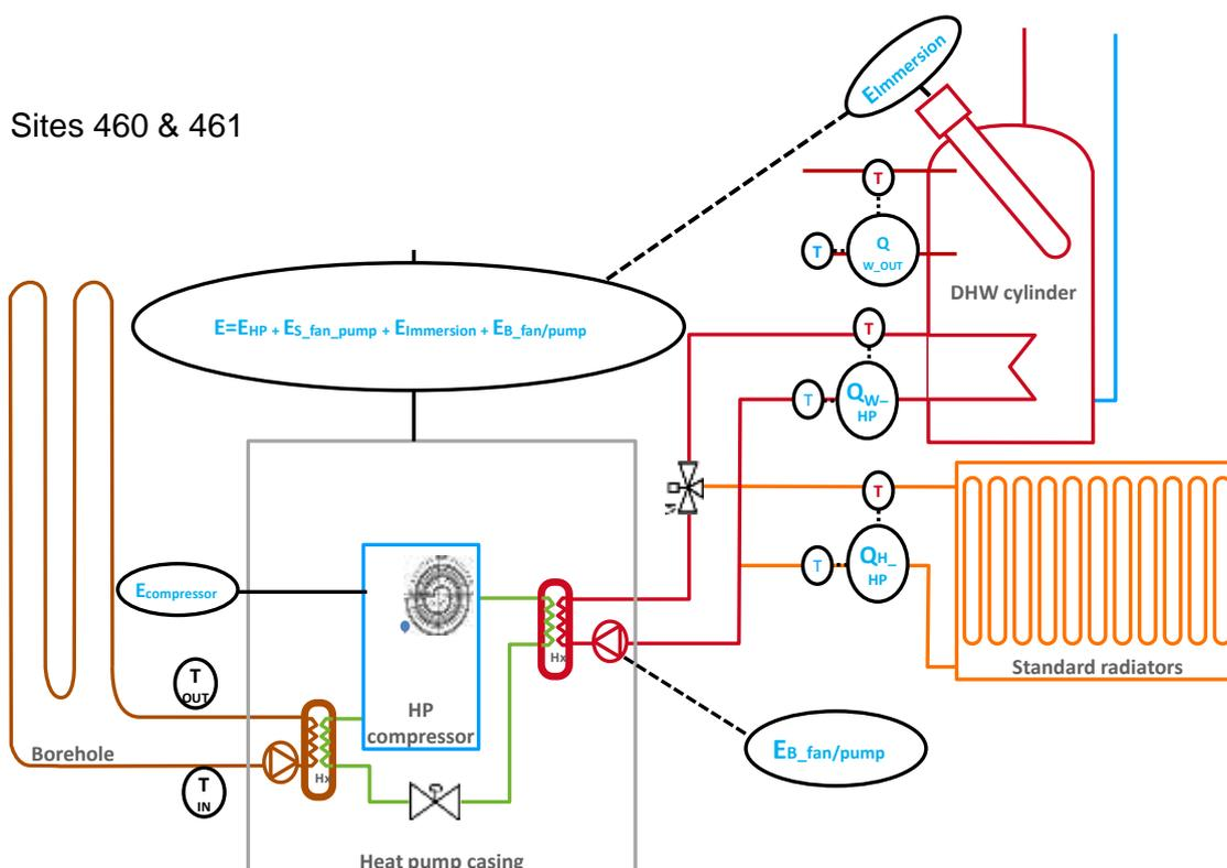
Figure 64: Schematic for site 460, Phase II
