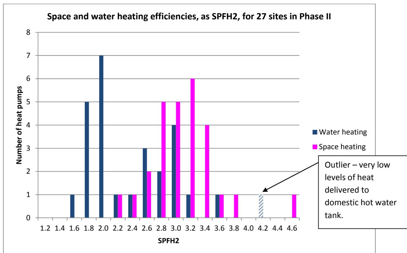
Figure 15: Space and water heating efficiencies as  $SPF_{H2}$  for 27 heat pumps, Phase II
