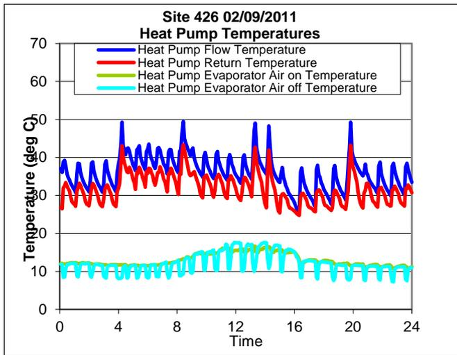
**Figure 47: Heat pump temperatures on 02/09/2011 at site 426 (Phase II)**
