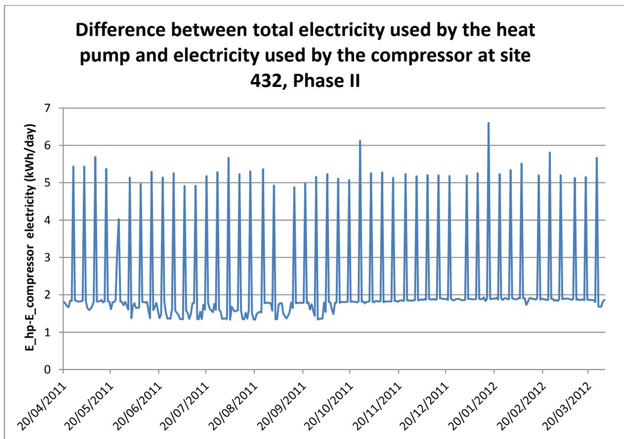
**Figure 61: Difference between total electricity used by the heat pump and electricity used by the compressor at site 432, Phase II**
