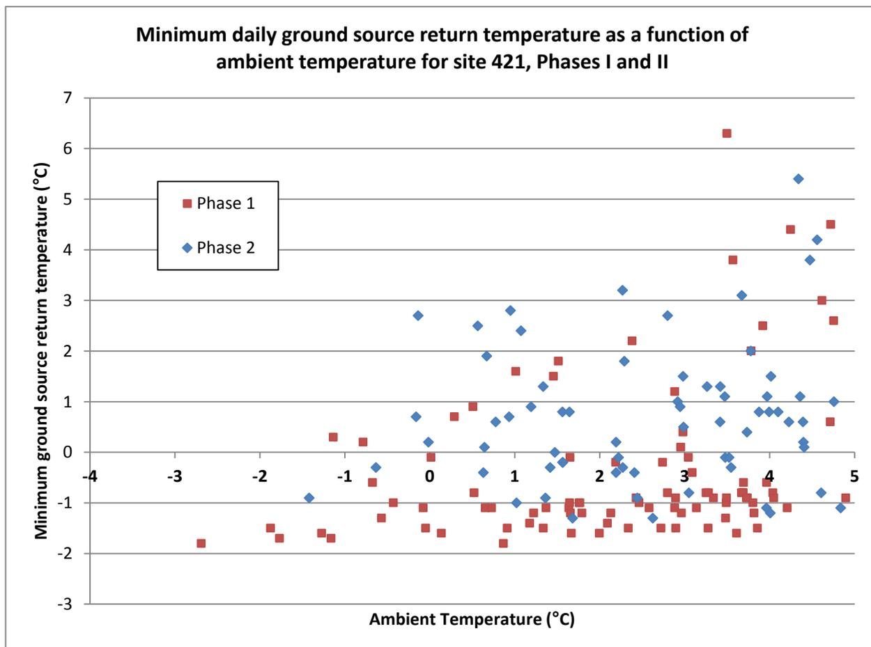
Figure 42: Minimum daily ground source return temperature as a function of ambient temperature for site 421, Phases I & II
