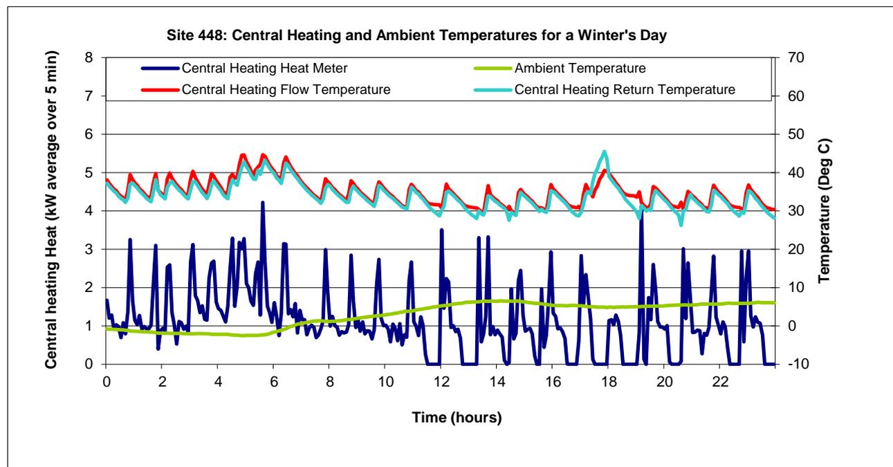
**Figure 70: Central heating flow and return temperatures and ambient temperatures on a typical winter's day for site 448, Phase II**
