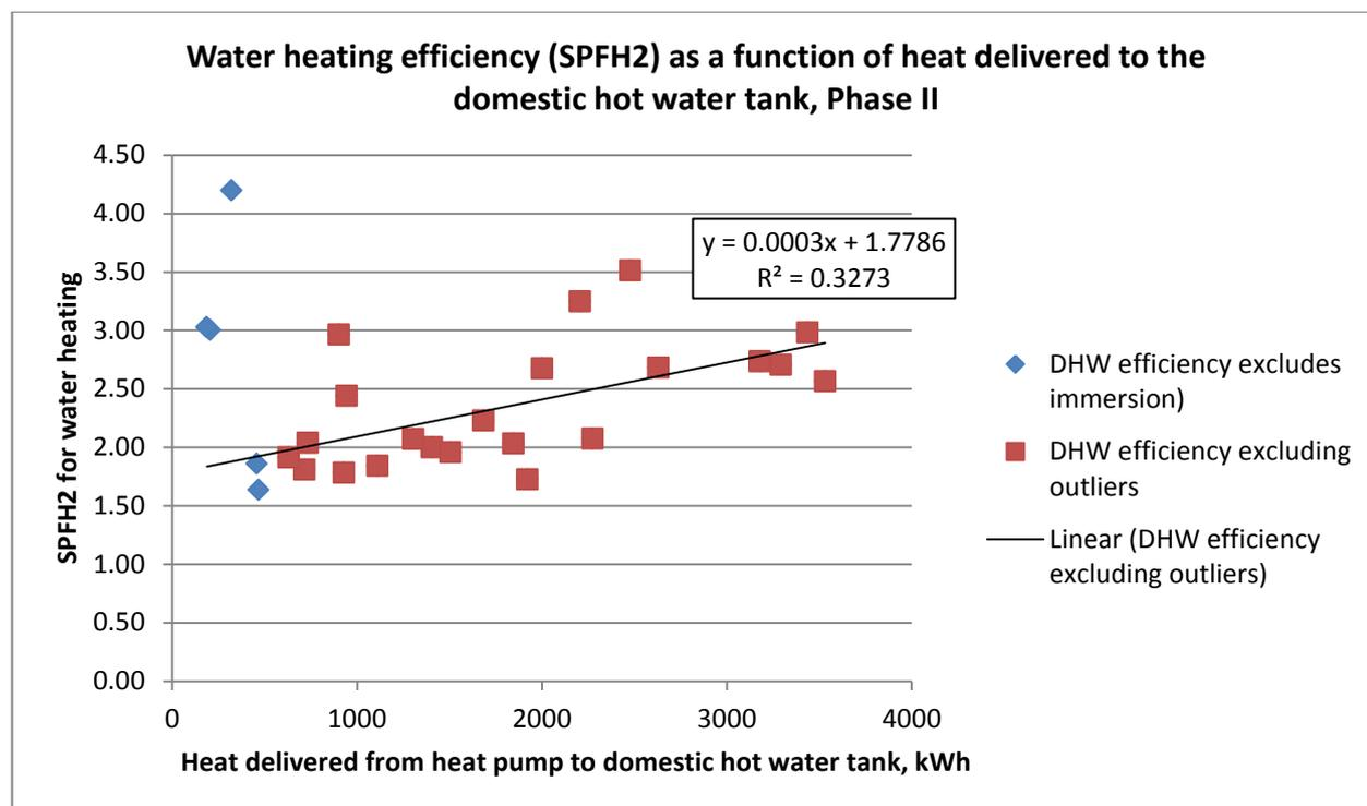
**Figure 20: Water heating efficiency (as  $SPFH_2$ ) as a function of heat delivered from the heat pump to the domestic hot water tank**
