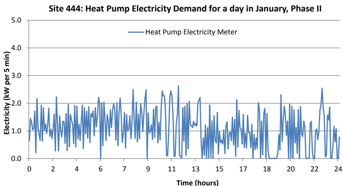
Figure 27: Electricity demand by heat pump 444 for a day in January 2012 (Phase II)
