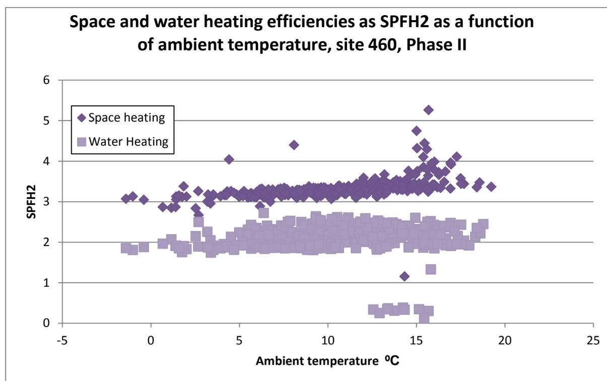
**Figure 65: Space and water heating efficiencies (as  $SPFH2$ ) as a function of ambient temperature at site 460, Phase II**
