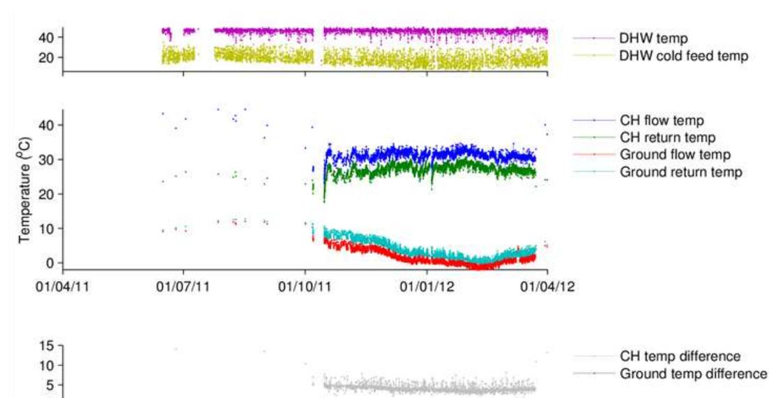
Figure 55: Central heating, domestic hot water and ground flow and return temperatures, site 416
