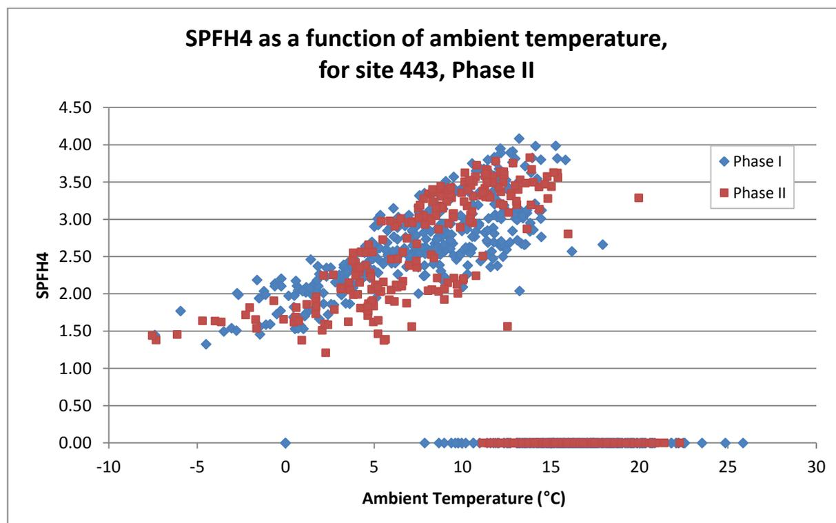
**Figure 67:  $SPF_{H4}$  as a function of ambient temperature for site 443, Phases I & II**
