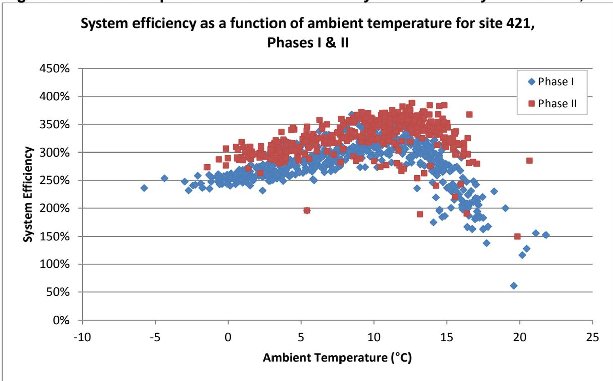
Figure 41: System efficiency as a function of ambient temperature for site 421, Phases I & II
