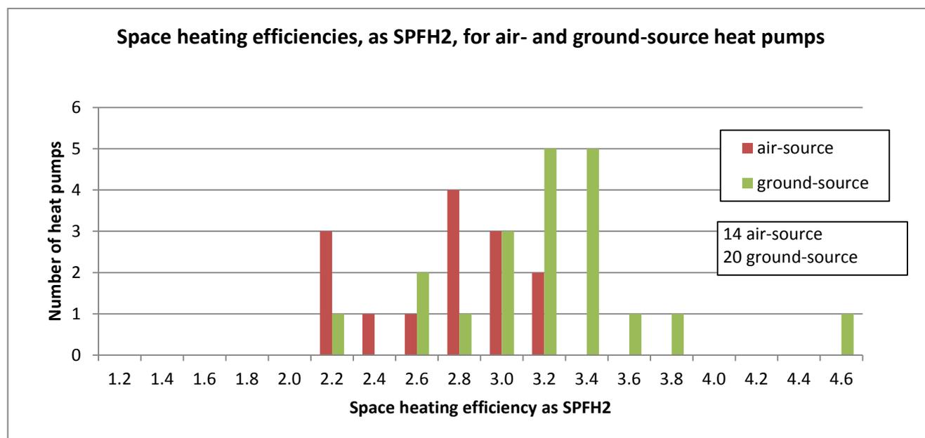
**Figure 16: Space heating efficiencies for 14 air- and 20 ground-source heat pumps (as  $SPF_{H2}$ )**
