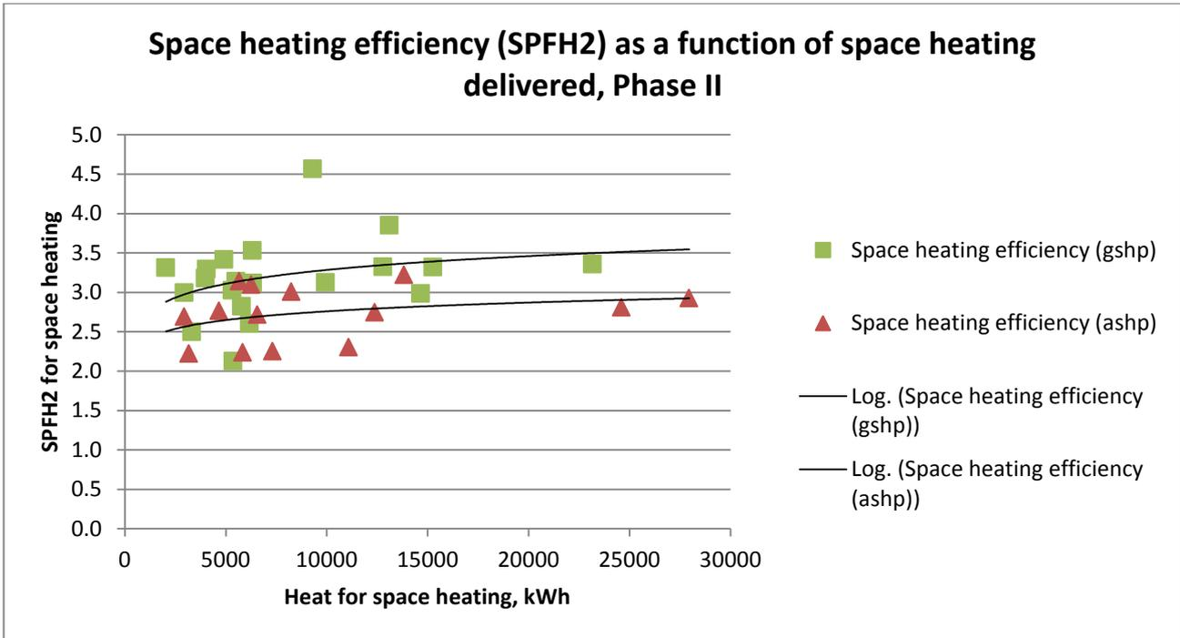
**Figure 17: Space heating efficiency as a function of space heating delivered for Phase II sites**
