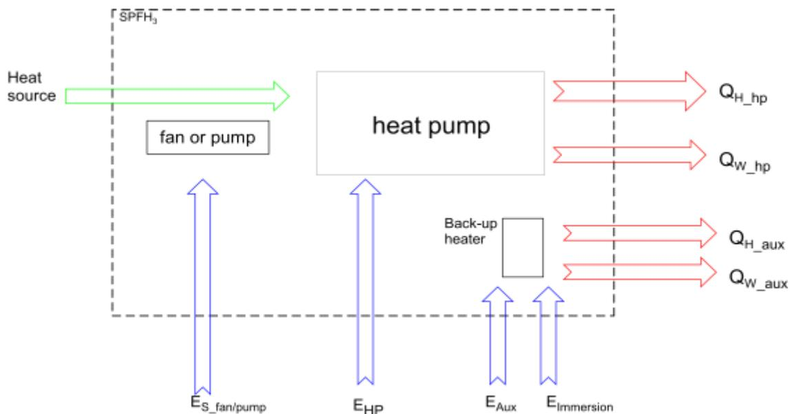
**Figure 4: System boundary for  $SPF_{H3}$ , as defined in the SEPAMO project**
