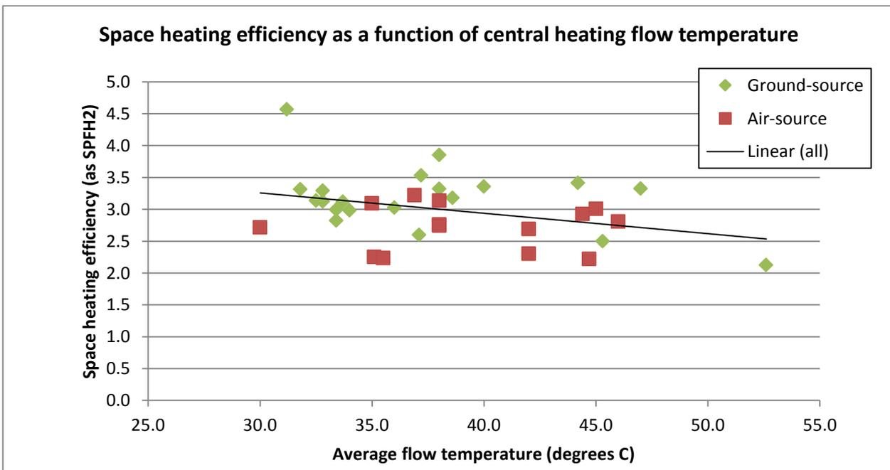
Figure 18 shows the average space heating efficiency (as  $SPF_{H2}$ ) as a function of the mode of the central heating flow temperature. There is a great deal of scatter, but, overall, the chart shows the expected decrease in space heating efficiency as central heating flow temperatures increase.
