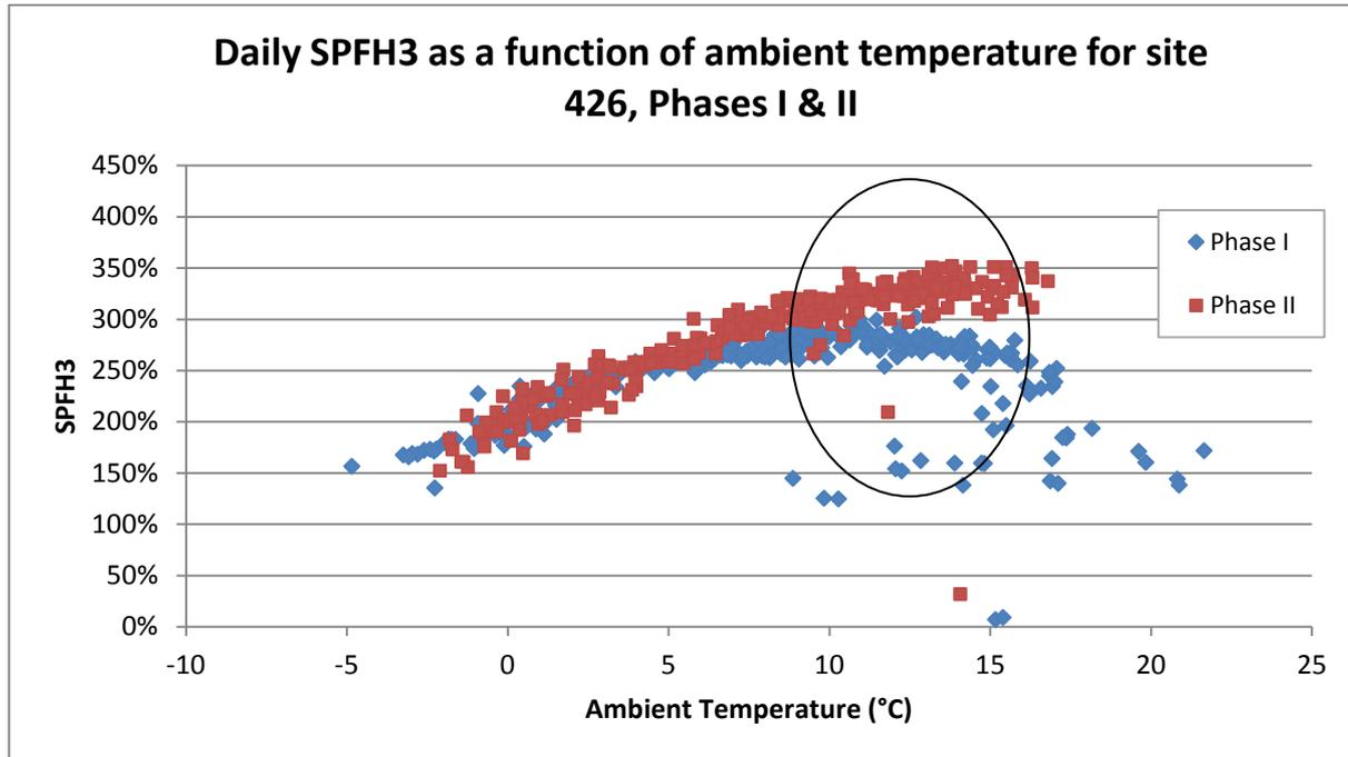
**Figure 44: Daily  $SPF_{H3}$  as a function of ambient temperature for site 426, Phases I & II**
