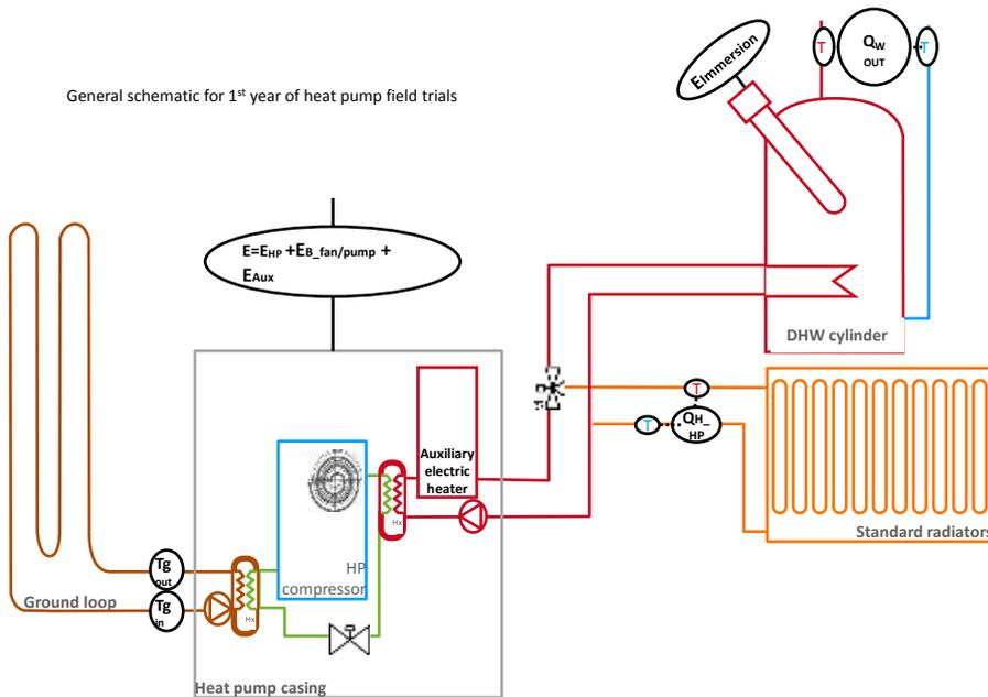
**Figure 7: Schematic of monitoring protocol for Phase I of the Energy Saving Trust heat pump field trials**
