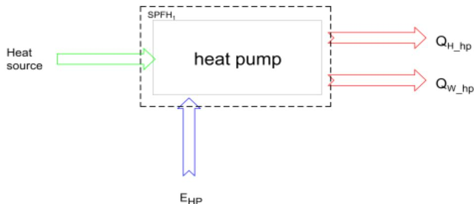
**Figure 2: System boundary for  $SPF_{H1}$ , as defined in the SEPEMO project**
