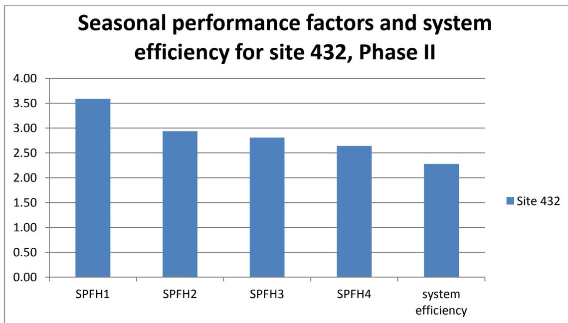
**Figure 60: Seasonal performance factors and system efficiency for site 432, Phase II**
