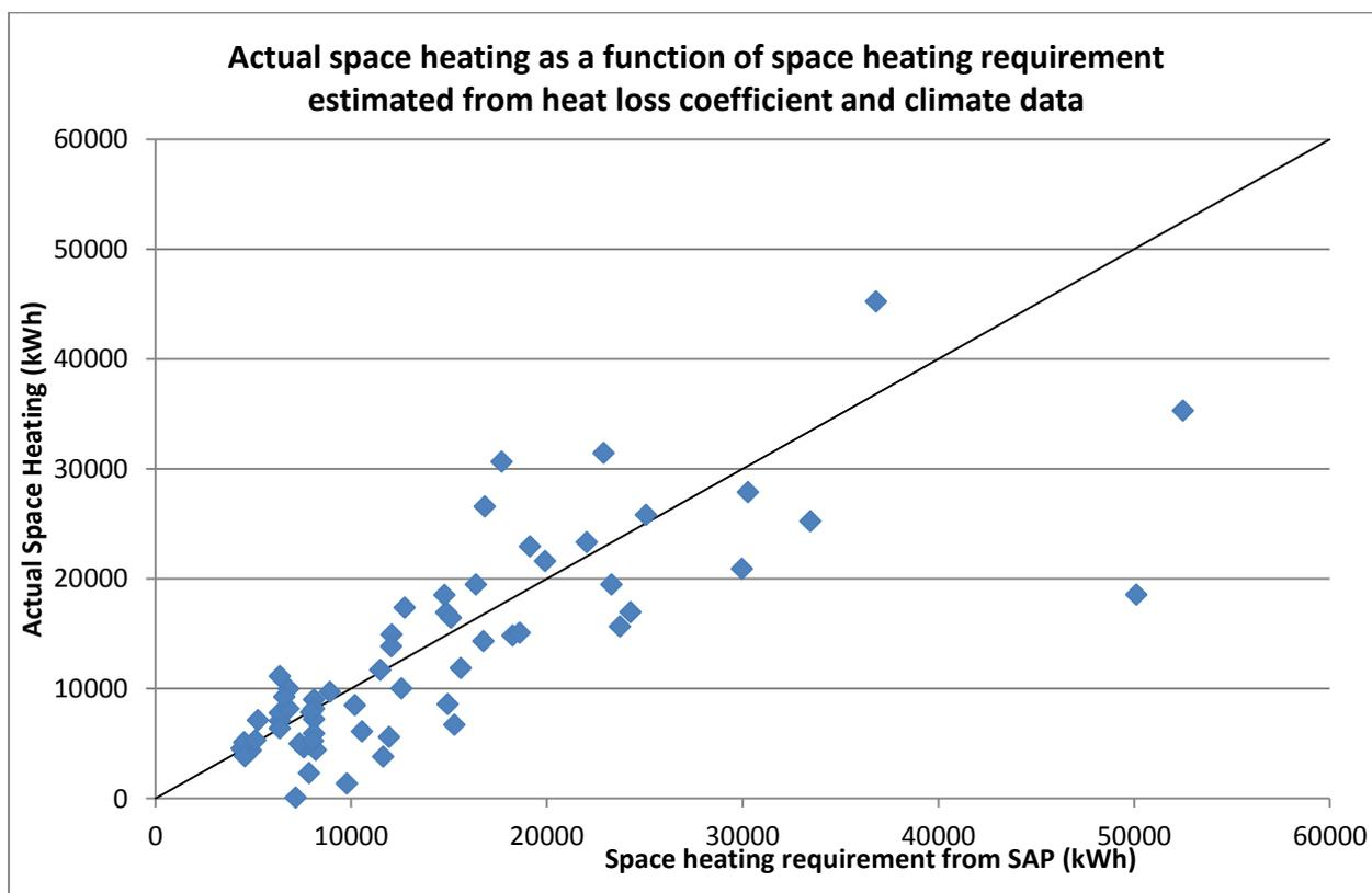
**Figure 80: Comparison of measured annual space heating demand with SAP estimates for Phase II sites**
