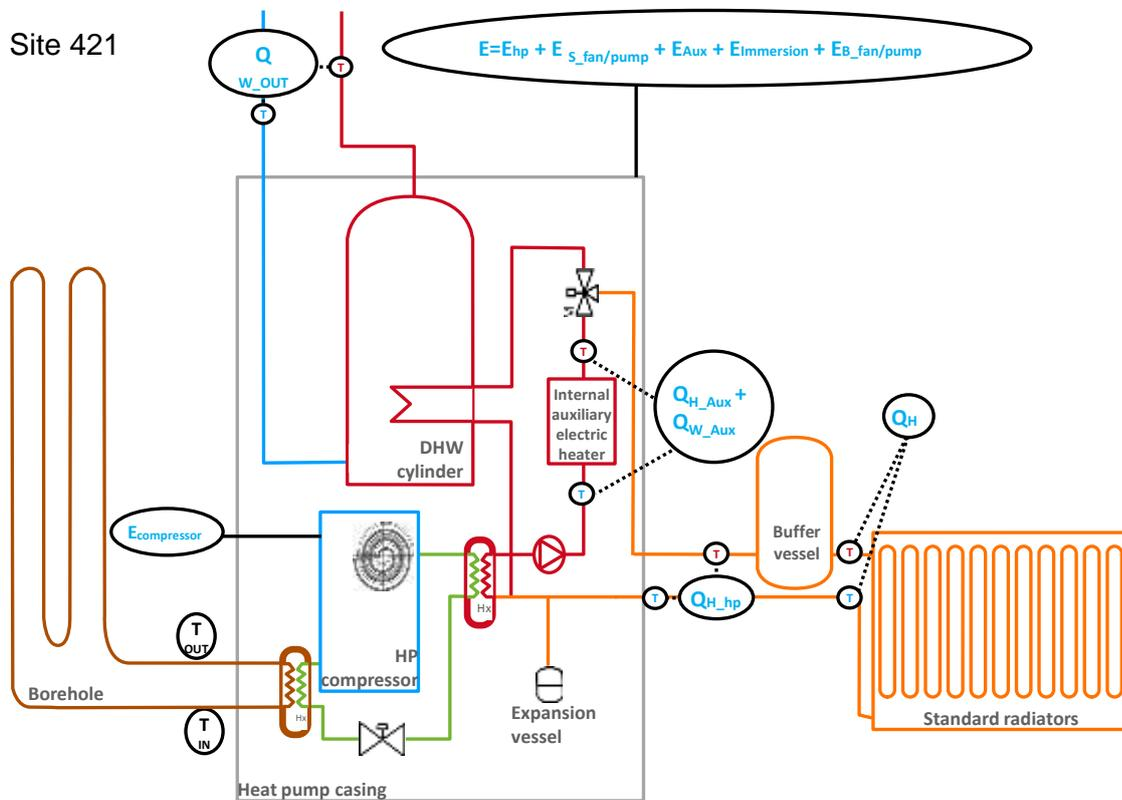
**Figure 39: Schematic for site 421, Phase II**
