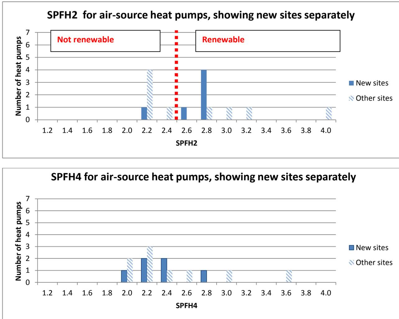
Figure 14: Comparison of  $SPF_{H2}$  and  $SPF_{H4}$  for the new air-source heat pumps in Phase II of the trial
