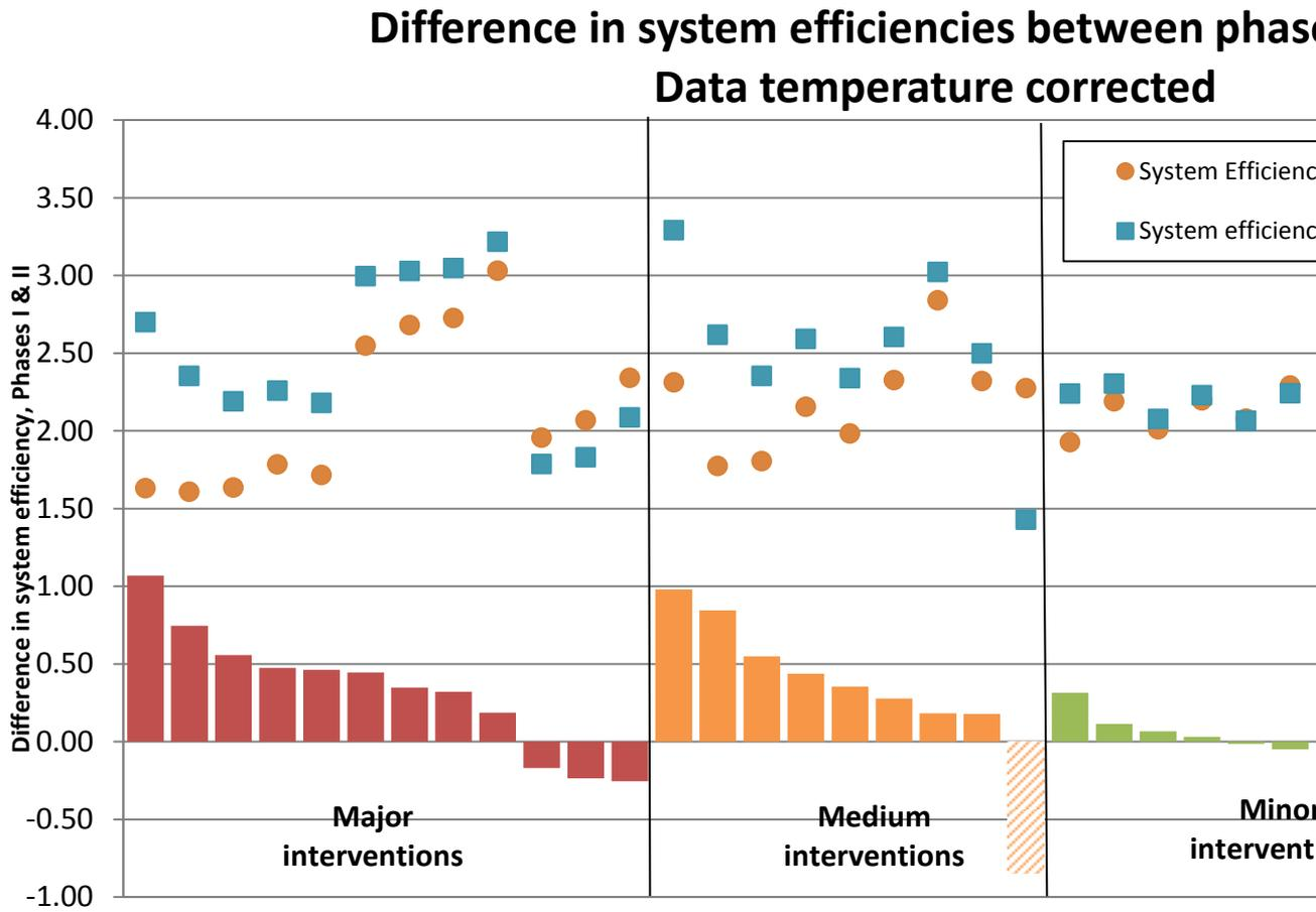
Figure 9 presents the difference in temperature-corrected system efficiency between Phases I and II. The orange points show the Phase I system efficiency, while the blue ones show the system efficiency for Phase II.
