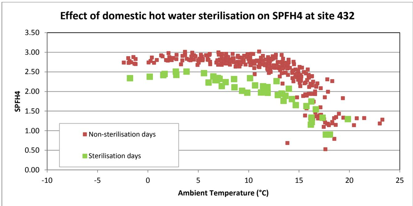
**Figure 63: Effect of domestic hot water sterilisation on  $SPF_{H4}$  at site 432**
