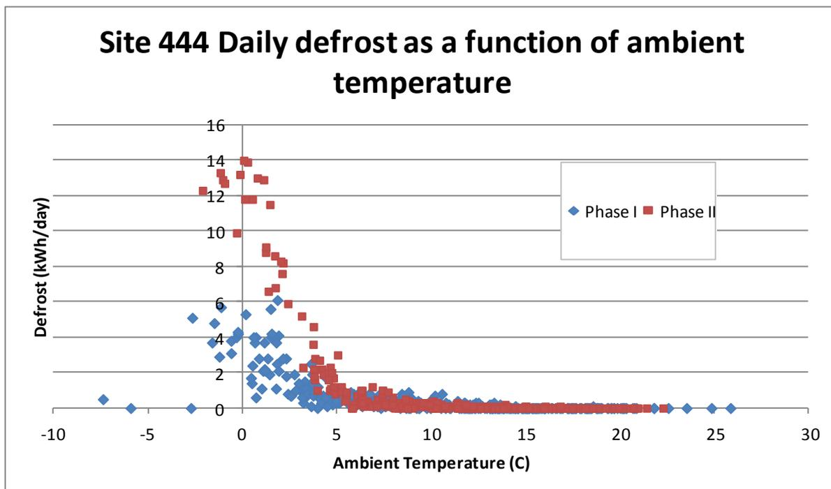
Figure 29: Daily defrost as a function of ambient temperature at Site 444, Phases I & II
