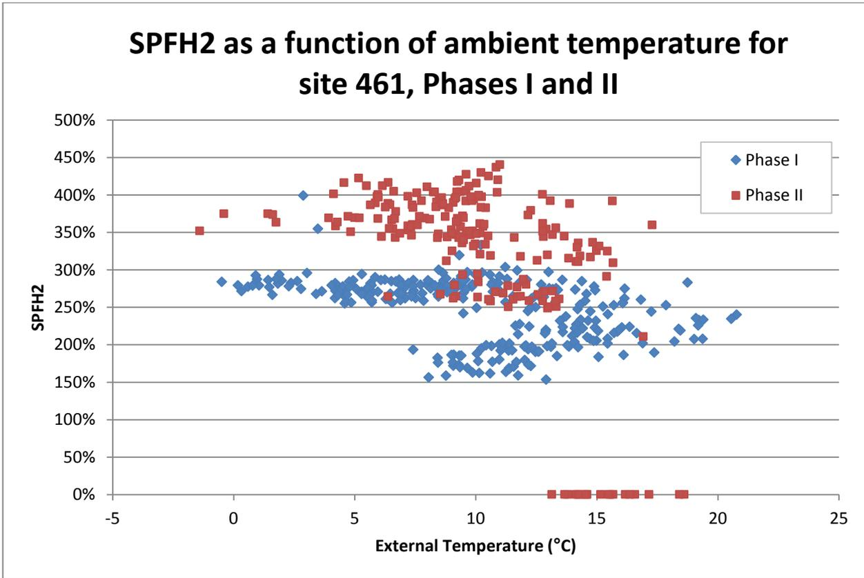
Figure 31: SPFH2 as a function of ambient temperature, site 461, Phases I & II
