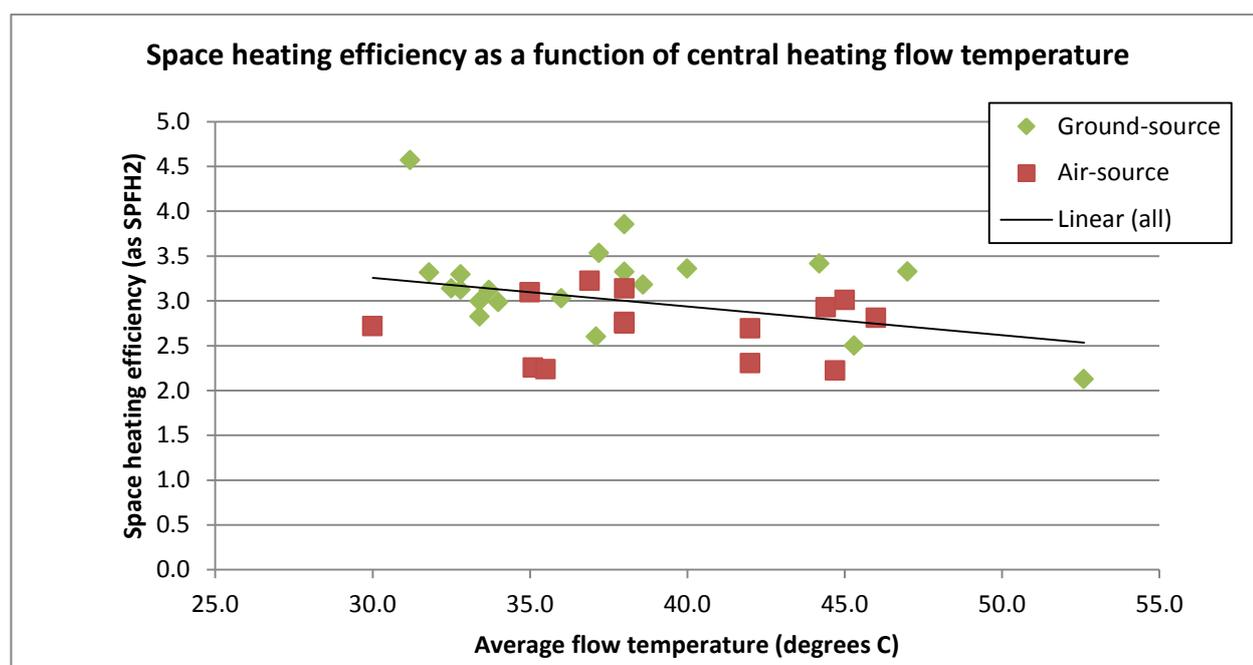
**Figure 18: Space heating efficiency as a function of central heating flow temperature for Phase II sites**
