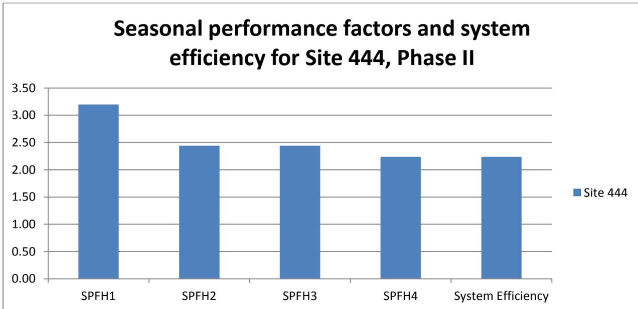
**Figure 22: Seasonal performance factors and system efficiency for site 444, Phase II**
