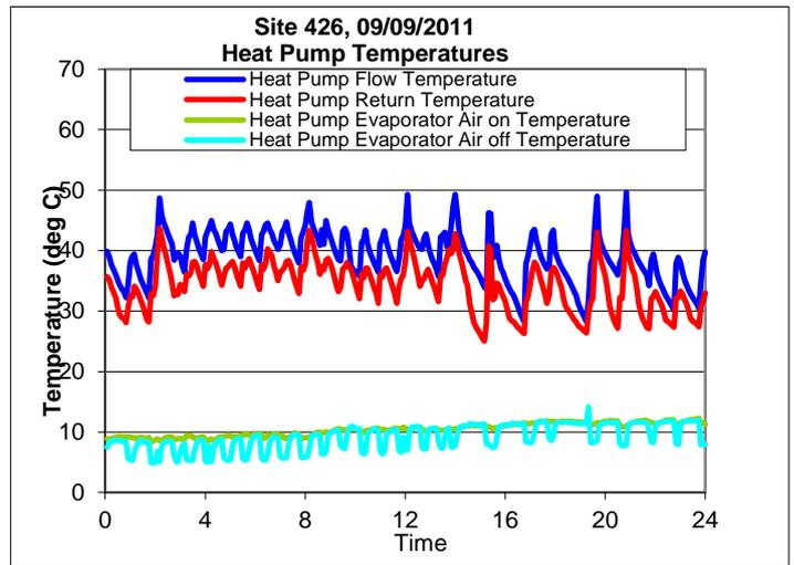
**Figure 48: Heat pump temperatures on 09/09/2011 at site 426 (Phase II)**
