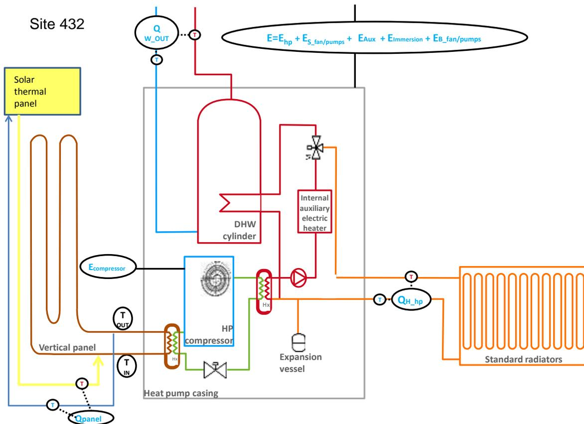
**Figure 59: Schematic for site 432, Phase II**
