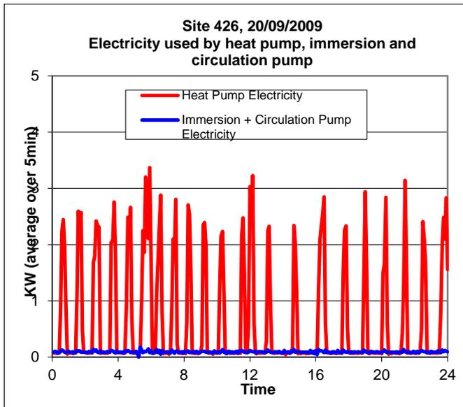
**Figure 49: Electricity consumption, site 426, 20/09/2009 (Phase I)**
