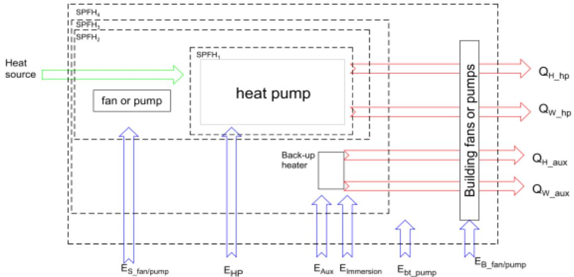
**Figure 1: System boundaries for space and water heating circuits, as defined in the SEPEMO project**
