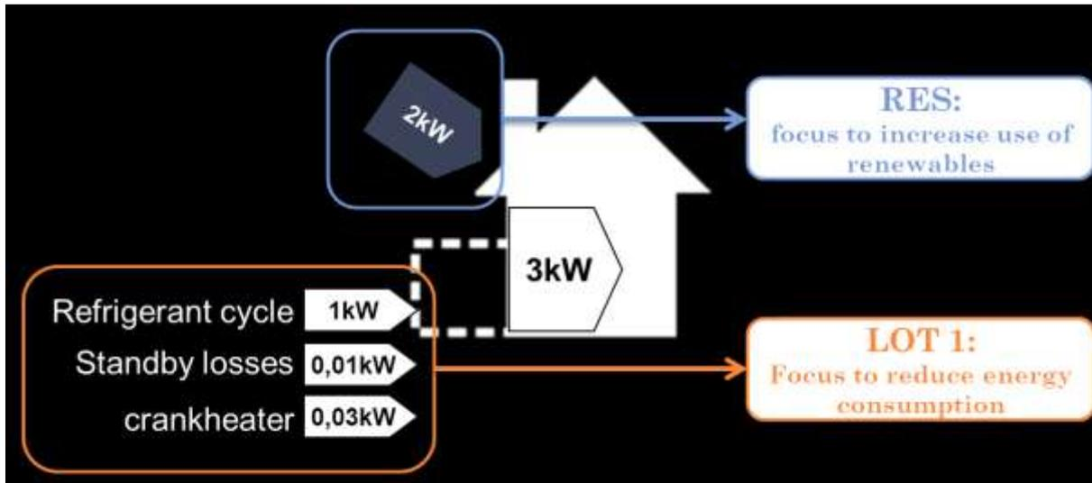
**Figure 6: Schematic to demonstrate the focus of the EU Eco-design Directive and that of the EU Renewable Sources Directive, as applied to heat pumps**
