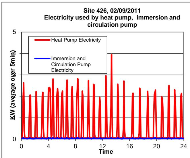
**Figure 51: Electricity consumption, site 426, 02/09/2011, Phase II**
