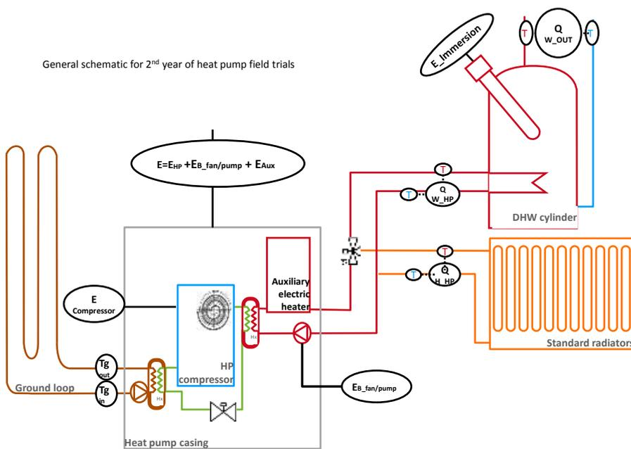
**Figure 8: Schematic of monitoring protocol for Phase II of the Energy Saving Trust heat pump field trials**
