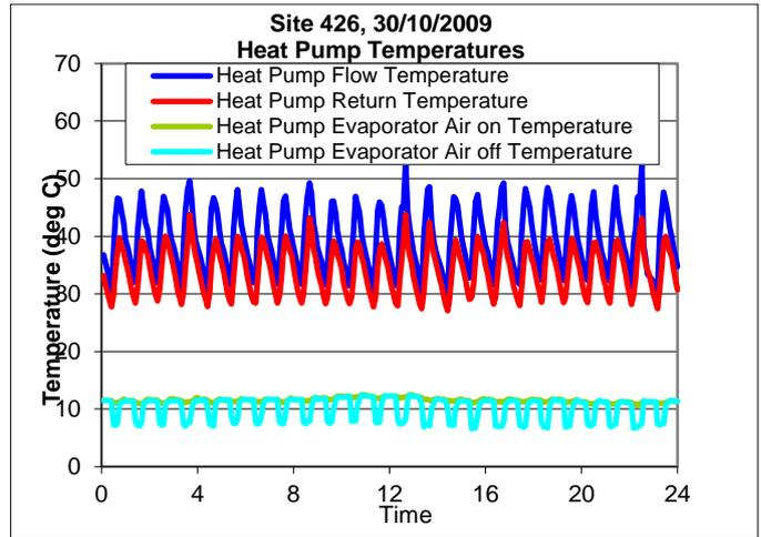
**Figure 46: Heat pump temperatures on 30/10/2009 at site 426 (Phase I)**
