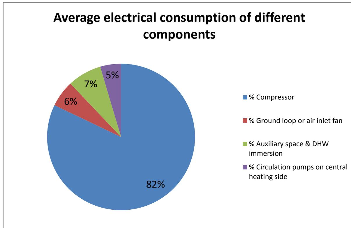
**Figure 11: Average electrical consumption of different components of heat pumps in the trial**
