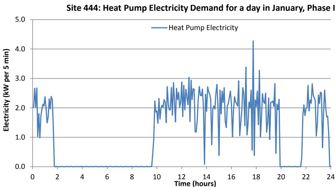
Figure 26: Electricity demand by heat pump 444 for a day in January 2010 (Phase I)
