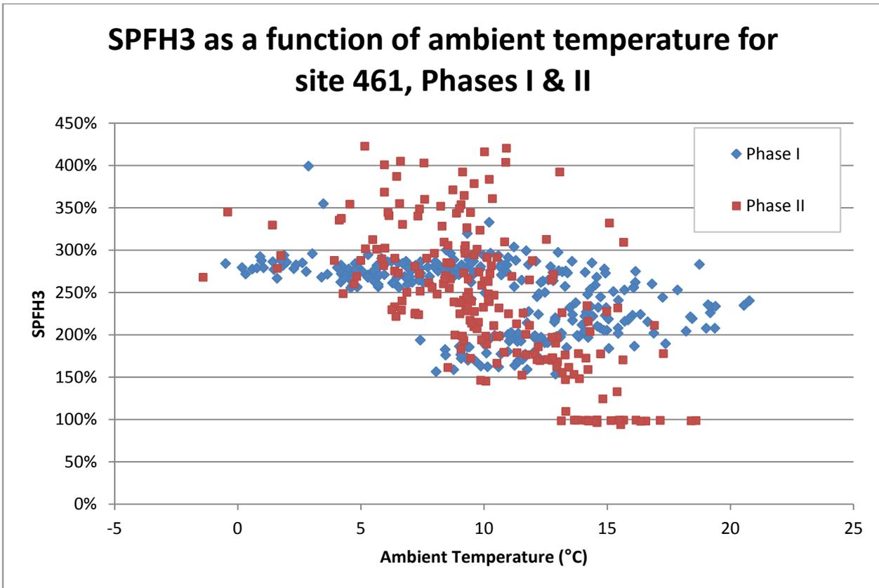
Figure 32: SPFH<sub>H3</sub> as a function of ambient temperature for site 461, Phases I & II
