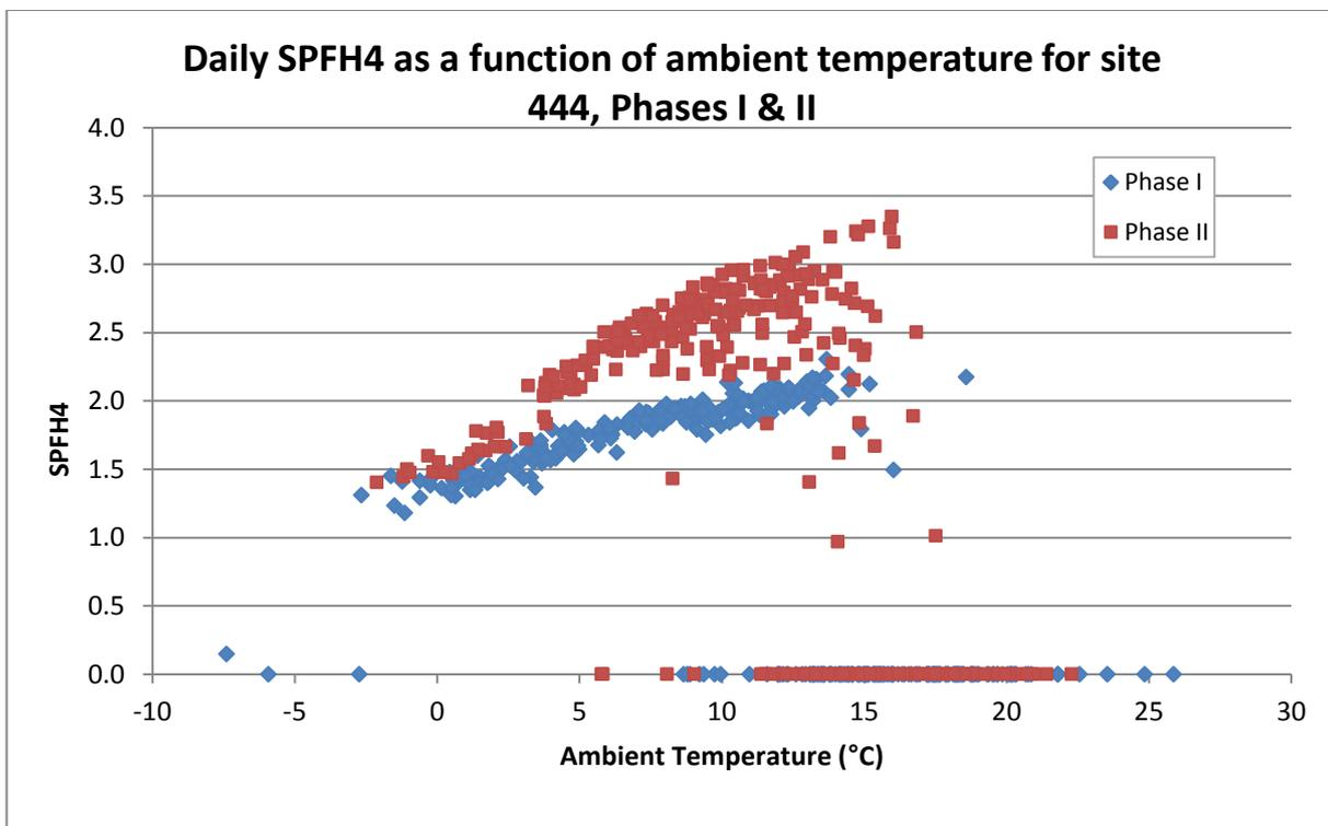
**Figure 23: Daily  $SPF_{H4}$  as a function of daily average ambient temperature for site 444, Phases I & II**
