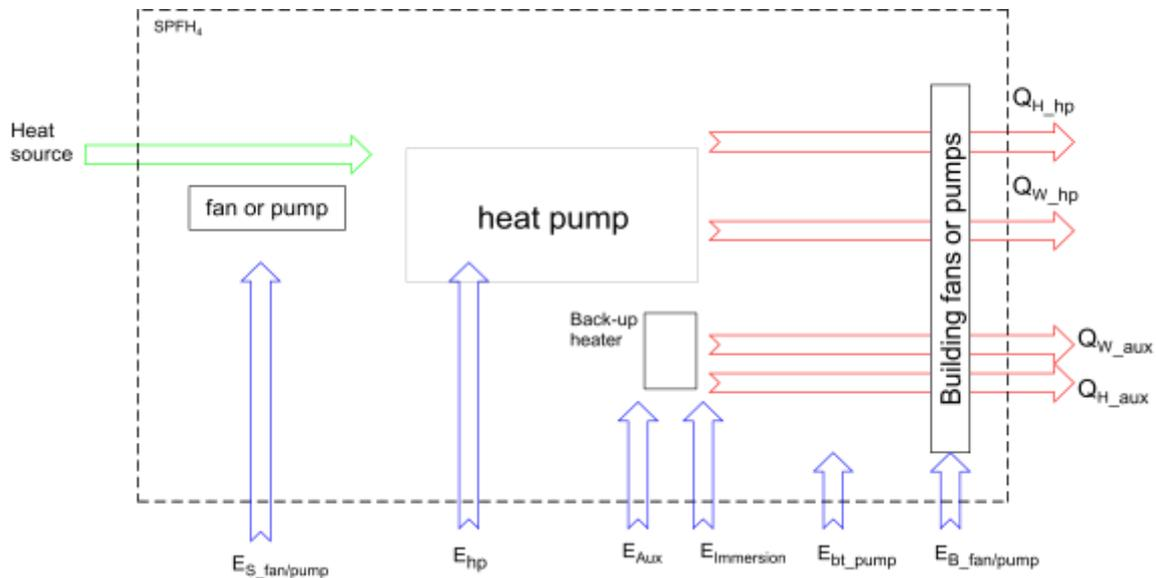
**Figure 5: System boundary for  $SPF_{H4}$ , as defined in the SEPEMO project**
