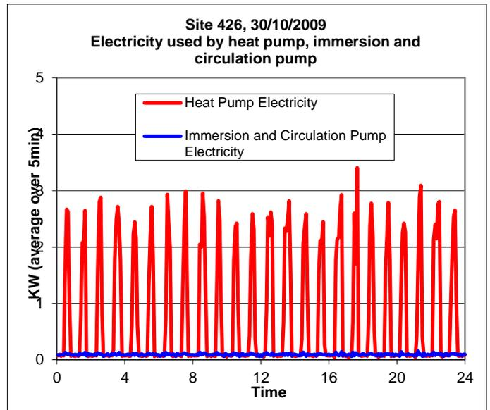
**Figure 50: Electricity consumption, site 426, 30/10/2009 (Phase I)**
