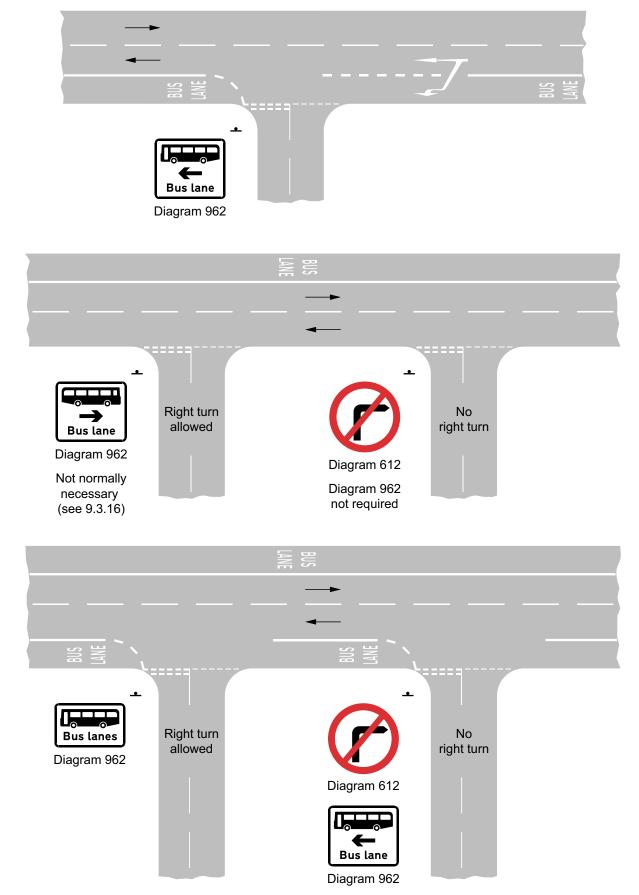
Figure 9-10 Examples of the use of the sign to diagram 962 to indicate with-flow bus lanes
