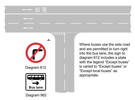
**Figure 9-18** Examples of the use of the signs to diagrams 962 and 962.2 to indicate contraflow bus lanes
