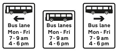
**Figure 9-9** Diagram 962 (variant) (S11-2-34) Bus lane on road at junction ahead with indication of times of operation (Alternative types)
