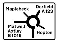
Two signs: These can provide a more compact arrangement. The sign to diagram 818.4 should be sited upstream of the advance direction sign for the junction
