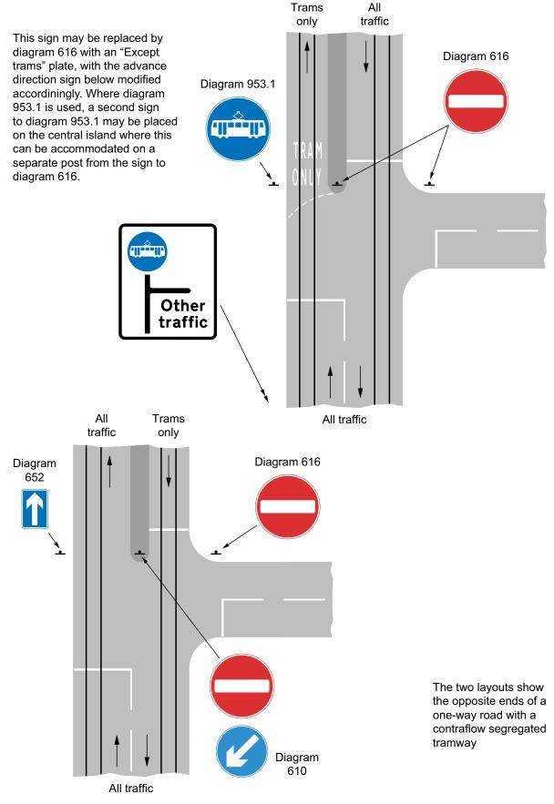
**Figure 10-8** Example of a one-way road used by all traffic with a contraflow segregated tramway
