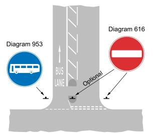
**Figure 9-14** Start of contraflow bus-only lane indicated by a sign to diagram 953
