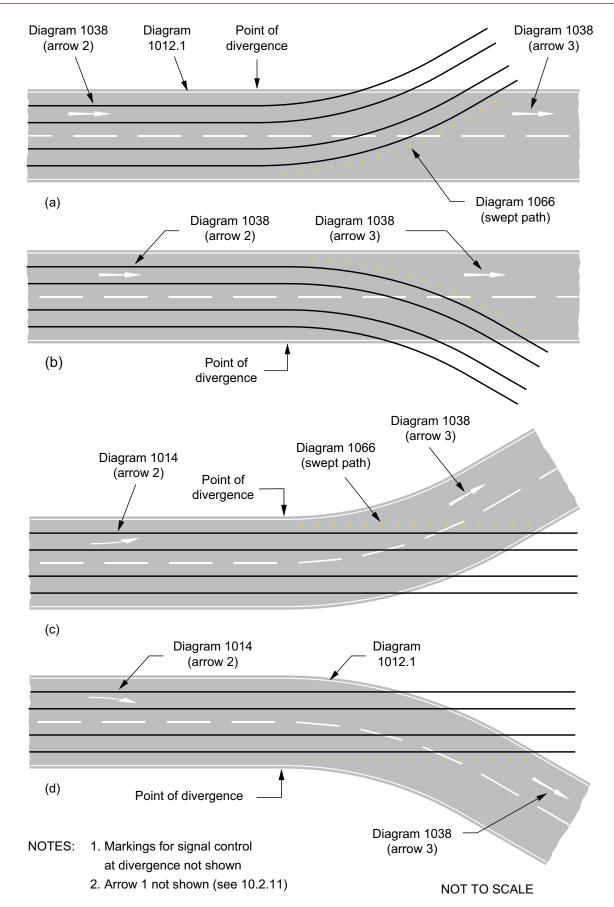
**Figure 10-10** Examples of a tramway leading from a public highway to an off-street route showing appropriate road marking guidance arrows
