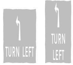
Figure 4-10 Diagram 1036.1 (S9-6-19) Vehicular traffic must turn left (Alternative types)
