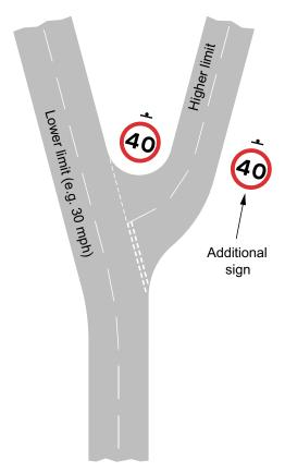
**Figure 8-4** Road junction where the side road makes an acute angle with the main road (Signs for drivers entering the side road)
