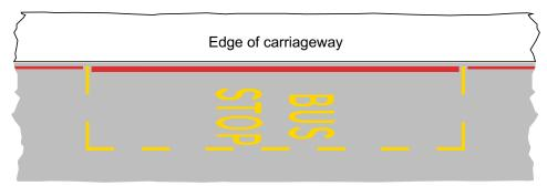
**Figure 16-7** Permitted variant of diagram 1025.1 for a bus stop clearway on red route where stopping by taxis is prohibited
