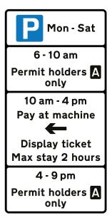
Figure 13-49 Example of a sign that is reserved for permit holders for only part of the day; at other times the parking conditions apply to all users including permit holders
