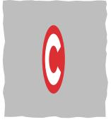
**Figure 12-2** Diagram 1068 (S8-4-7) Road marking indicating the commencement of a congestion charging zone
