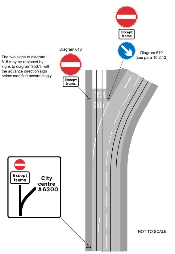
**Figure 10-9** Example of a tramway leading from a public highway to an off-street route showing appropriate upright signs
