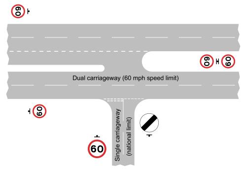
**Figure 8-7** Example of terminal signs at a road junction where the main road is a dual carriageway with a speed limit of 60 mph and the side road is a single carriageway subject to the national speed limit of 60 mph
