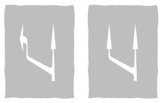
**Figure 9-6** Diagram 1050 (S9-6-12) Indication of traffic movements at end of nearside bus lane or intermediate junction (Alternative types)
