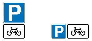
Figure 11-31 Diagrams 968 and 968.1 (S11-2-47) Parking place for pedal cycles
