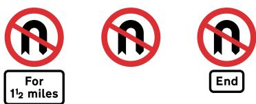
Figure 4-34 Diagram 614 (S3-2-6) No U-turns for vehicular traffic (Alternative types)
