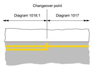
Figure 13-8 Changeover point from diagram 1018.1 to diagram 1017
