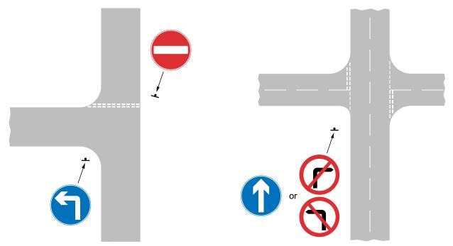
**Figure 4-16** Signing arrangement at unsignalled junction where ahead manoeuvre is prohibited
