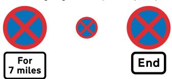
Figure 7-1 Diagram 642 (S3-2-4) No stopping on main carriageway (Alternative types)
