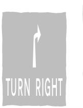
Figure 4-11 Diagram 1037.1 (S8-6-21) Vehicular traffic must turn right (Alternative types)
