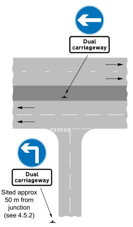
**Figure 4-5** Signing arrangement at unsignalled junction where side road meets dual carriageway
