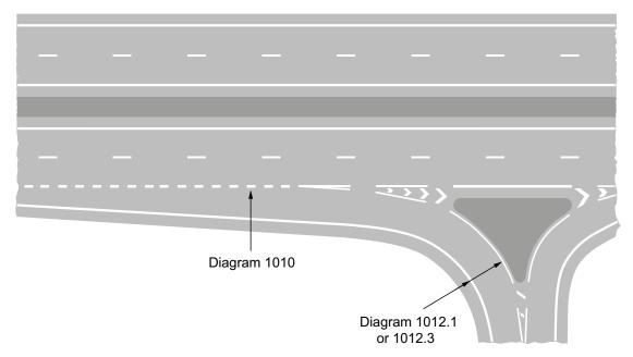
Figure 3-7 Markings for acceleration lane on high speed dual carriageway
