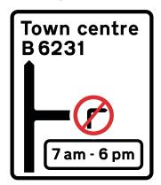
**Figure 4-23** Map-type direction sign incorporating "no right turn" roundel and supplementary time plate
