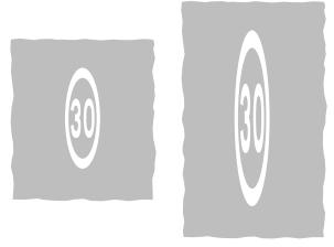
Figure 8-22 Diagram 1065 (S10-2-9) Road marking indicating maximum speed limit (Alternative sizes)
