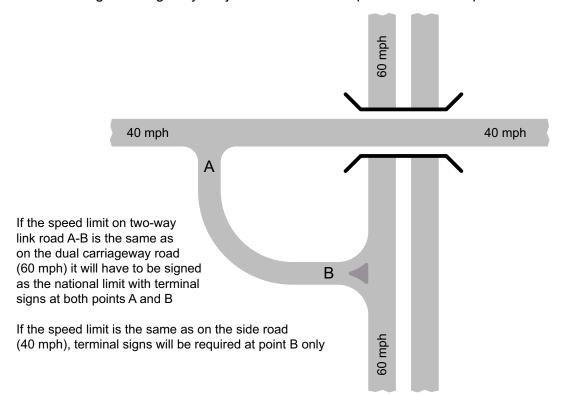
**Figure 8-8** Speed limit on two-way link road between a dual carriageway road with a speed limit of 60 mph and a side road with a speed limit of 40 mph
