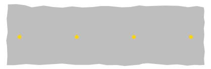
**Figure 10-14** Diagram 1066 (S11-4-36) Edge of part of road used by tramcars (Longitudinal marking)
