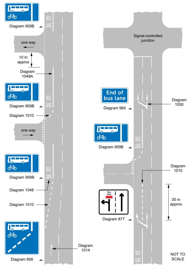
Figure 9-1 Typical layout for a with-flow bus lane
