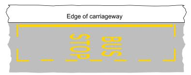
Figure 13-71 Diagram 1025.1 (S7-4-9) Bus stop clearway road marking
