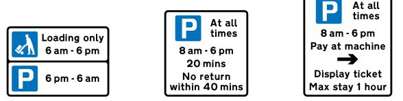
**Figure 15-3** Examples of upright signs indicating loading and parking bays where controls do not apply throughout the operational period of the restricted parking zone
