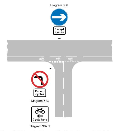
**Figure 11-12** Example of the use of the sign to diagram 962.1 to indicate a mandatory contraflow cycle lane
