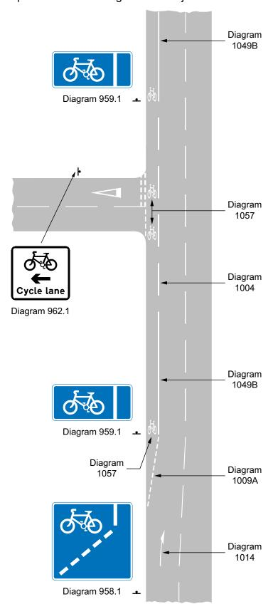
Figure 11-2 Example of a mandatory with-flow cycle lane
