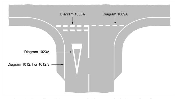
Figure 3-6 Layout used where a 1 m hard strip is provided on the main carriageway
