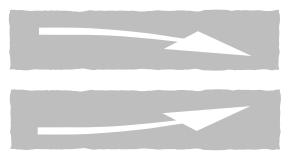
**Figure 10-11** Diagram 1014 (S11-4-14) Deflection arrow (Longitudinal marking) (Alternative types)
