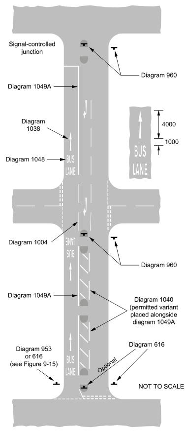
Figure 9-12 Typical layout for a contraflow bus lane
