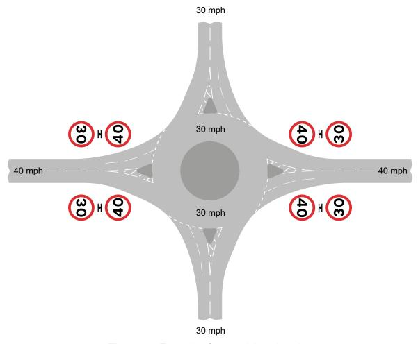
Figure 8-5 Example of a roundabout junction
