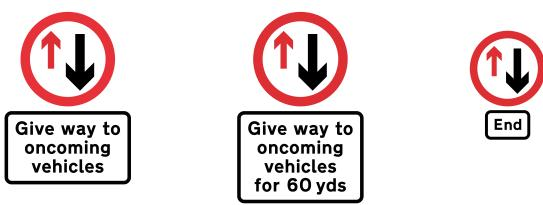
**Figure 4-27** Diagram 615 (S3-2-9) Priority must be given to vehicles from the opposite direction (Alternative types)
