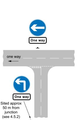
Figure 4-4 Signing arrangement at unsignalled junction where side road meets one-way road
