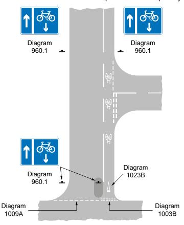
**Figure 11-8** Example of signs indicating a mandatory contraflow cycle lane to other drivers and road markings at end of cycle lane
