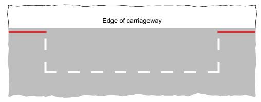
**Figure 16-5** Road marking to diagram 1028.4 where a parking or loading bay is always available for a specified class of user during the period of operation of a red route
