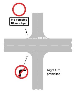
**Figure 4-20** Signing arrangement at crossroads where ahead manoeuvre is prohibited 10 am - 4 pm and right turn is prohibited
