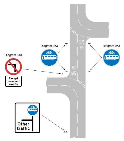
Figure 9-26 Example of a two-way bus gate
