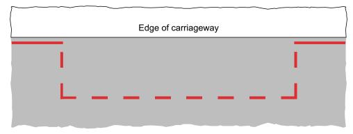
**Figure 16-6** Permitted variant of diagram 1028.4 where a parking or loading bay is available for a specified class of user during part of the period of operation of a red route with no stopping at other times, or where the bay operates only outside the period of operation
