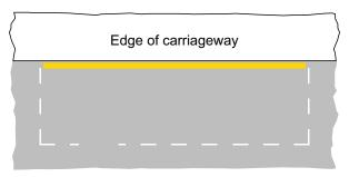
**Figure 13-68** Diagram 1028.6 (S7-4-8) Taxi rank marking where stopping by other vehicles is prohibited at certain times and where it is a controlled parking or loading bay at other times
