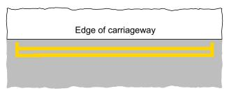
**Figure 13-6** Diagram 1018.1 (S7-4-1) Waiting of vehicles prohibited at all times or stopping of vehicles in a lay-by prohibited except in an emergency
