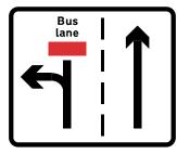
**Figure 9-8** Diagram 877 (S11-2-22) Appropriate traffic lanes for manoeuvres at junction ahead (variant)
