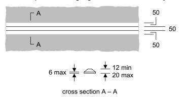
Figure 11-21 Diagram 1049.1 (S9-6-8) Division of route into that part reserved for pedal cycles and that part reserved for pedestrians (Longitudinal marking)
