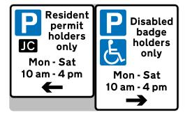
Figure 13-62 Signing arrangement for different parking bays side by side (Alternative types)
