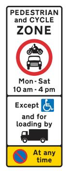
**Figure 6-2** Diagram 618.3C (S8-2-2) Entry to, and waiting in, pedestrian and cycle zone restricted
