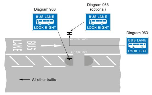
Figure 9-21 Example of the use of pedestrian signs to diagram 963 to indicate a contraflow bus lane
