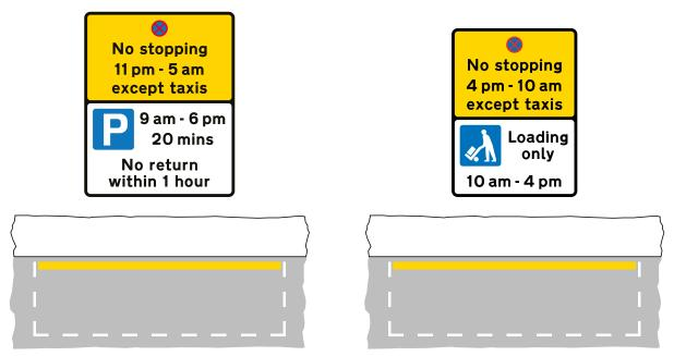
**Figure 13-69** Examples of signs and markings for a part-time "no stopping" taxi rank that is used as a controlled parking or loading bay at other times
