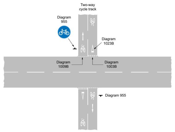
Figure 11-27 Typical layout of a cycle crossing a road where priority is to road traffic
