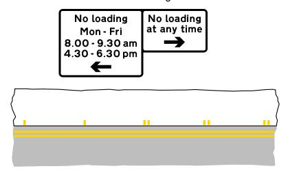
**Figure 13-18** Prohibition of loading changes from peak-hour to at any time, with no change to prohibition of waiting at any time
