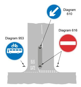
Figure 9-25 One-way bus gate on a two-way road
