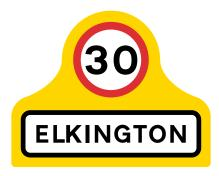
Figure 8-21 Example of a speed limit sign co-located with a boundary sign
