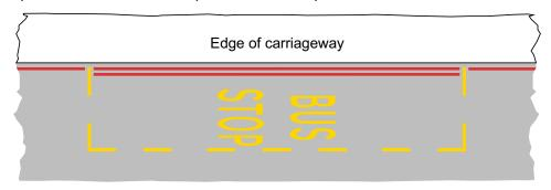
**Figure 16-8** Permitted variant of diagram 1025.1 for a bus stop clearway on red route where taxis may stop to pick up and set down passengers
