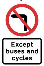
Figure 4-21 Example of a sign to diagram 613 with an exception plate
