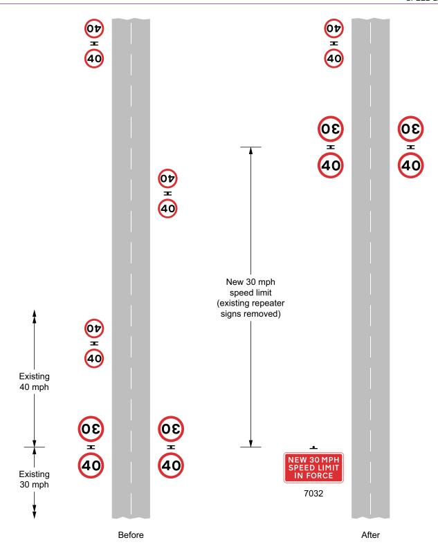
There is no specific requirement to provide two terminal signs for each speed limit. There might be situations where the traffic authority considers that a single terminal is sufficient
