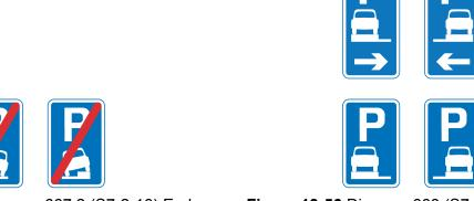
**Figure 13-55** Diagram 667.2 (S7-2-16) End of area where vehicles may be parked partially on the verge or footway (Alternative types)
