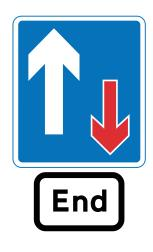
**Figure 4-28** Diagram 811A (S11-2-1) Beginning of section of road where traffic has priority over vehicles from the opposite direction (Alternative types)
