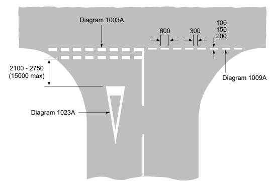
Figure 3-5 Road markings at a junction where vehicles give way
