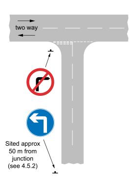
**Figure 4-6** Signing arrangement at unsignalled junction where side road meets two-way road
