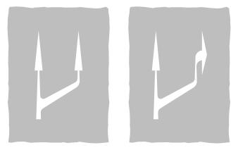
**Figure 9-7** Diagram 1050.1 (S9-6-13) Indication of traffic movements at end of off-side bus lane or intermediate junction (Alternative types)
