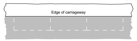
Figure 13-26 Example of a parking bay parallel to the edge of the carriageway and divided into individual spaces
