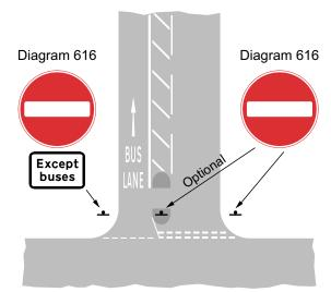
**Figure 9-15** Start of contraflow bus-only lane indicated by signs to diagram 616
