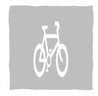
**Figure 11-1** Diagram 1057 (S11-4-28) Road marking indicating a cycle lane, track or route (Alternative types)
