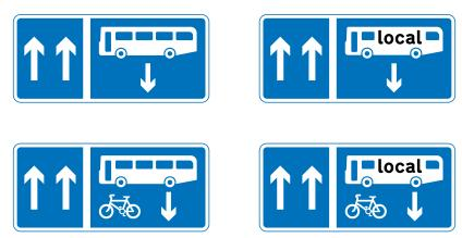
Figure 9-11 Diagram 960 (S9-4-8) One-way road with contraflow bus lane (Alternative types)
