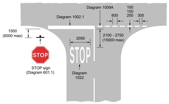
Figure 2-5 Road markings at a junction controlled by a STOP sign
