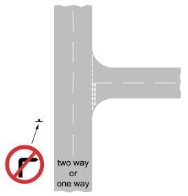
**Figure 4-12** Signing arrangement where traffic is prohibited from turning into side road at unsignalled T-junction
