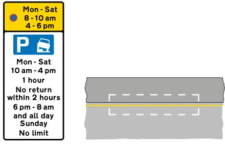
Figure 13-61 Example of an upright sign and road marking indicating footway parking controls
