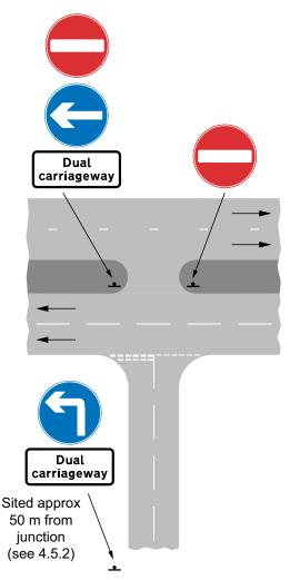
**Figure 4-7** Signing arrangement at unsignalled junction where side road meets a dual carriageway and there is a banned right turn
