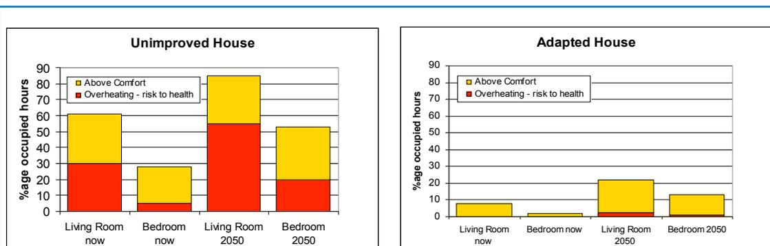
A range of measures are recommended to retrofit homes to ensure that excessive solar gain in the summer is avoided. Some of these measures, including cavity wall and loft insulation, are also of direct benefit now and in 2050 to retain warmth in the home during the cold winter months. Note that adequate ventilation is needed to ensure that heat does not become trapped within the building.
