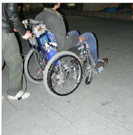
The second work stream focused on wheelchair navigation over a crossfall, or gradient across a footpath. Researchers took a detailed look at how the degree of gradient of the crossfall affects attendant pushing patterns, as well as self-propulsion patterns. Using the PAMELA
