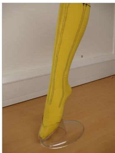
Initial tests showed that the relationship between signals from the sensors and the 3D orientation of the foot was much less predictable than had been expected. However, it proved possible to use the signals to detect significant changes in gait to an average accuracy of between 1% and 3.3% of the gait cycle, which is comparable with other currently used measurement approaches. The questionnaire results showed that people found the sock comfortable and easy to get on and off.
