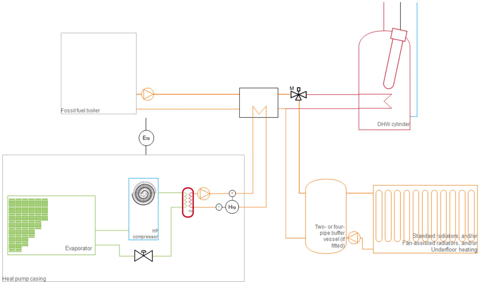
**Figure 5: Air-source heat pump with back-up fossil fuel boiler showing metering option 2: 1 heat meter (integrated) and 1 electricity meter**
