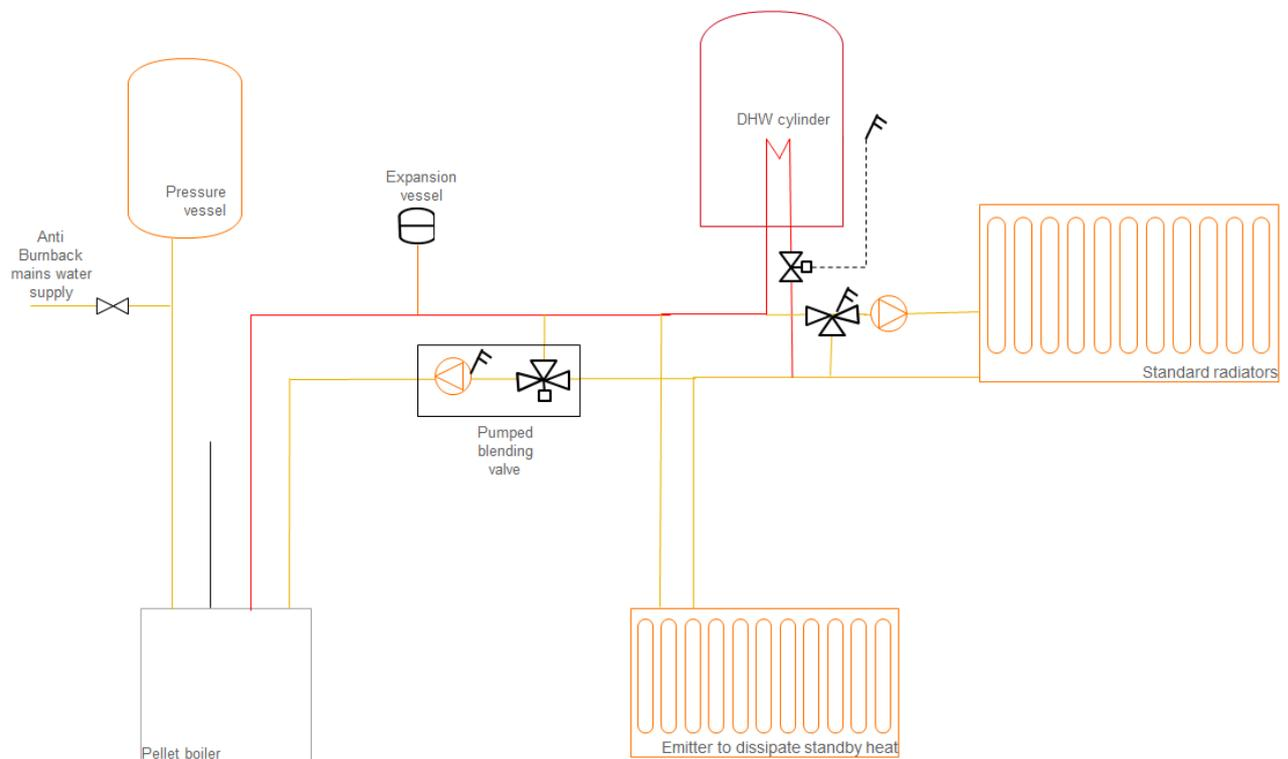
**Figure 1: Pellet biomass boiler**
