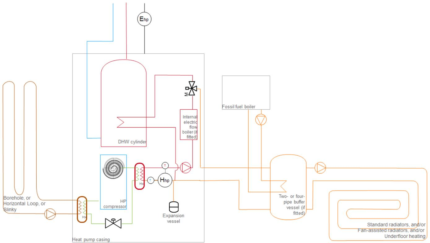
**Figure 8: Ground-source heat pump with integrated domestic hot water cylinder and metering option 2: 1 heat meter (integrated), 1 electricity meter**
