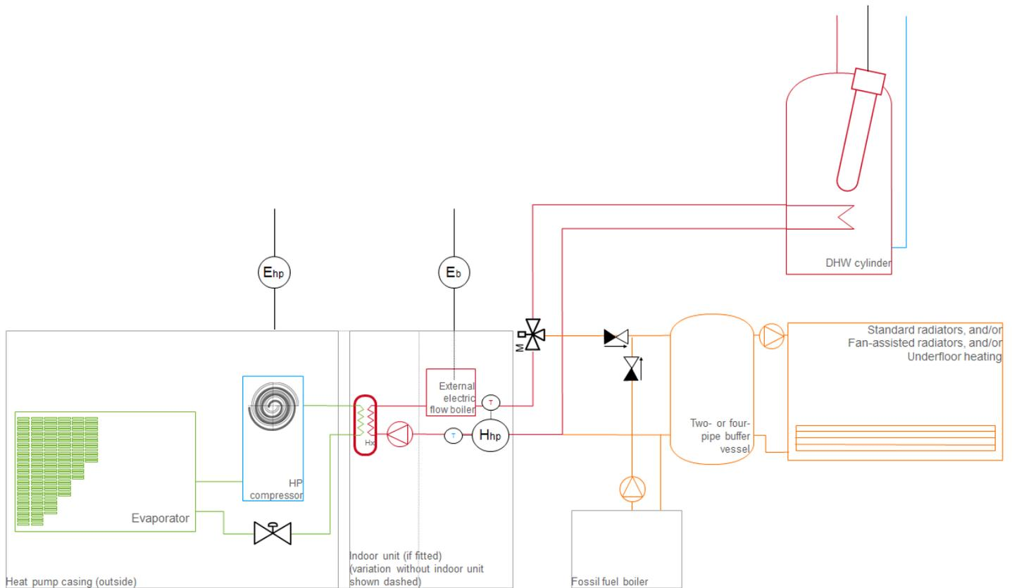
**Figure 11: Split-system air-source heat pump with metering option 2: 1 heat meter (integrated), 2 electricity meters**
