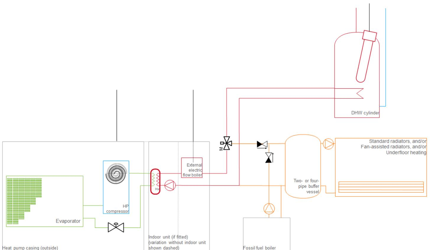
**Figure 9: Split-system air-source heat pump providing space heating and hot water**
