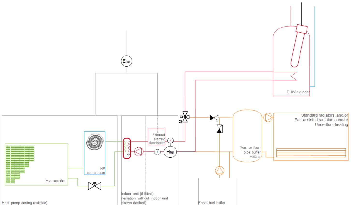
**Figure 12: Split-system air-source heat pump with metering option 3: 1 heat meter (integrated), 1 electricity meter**
