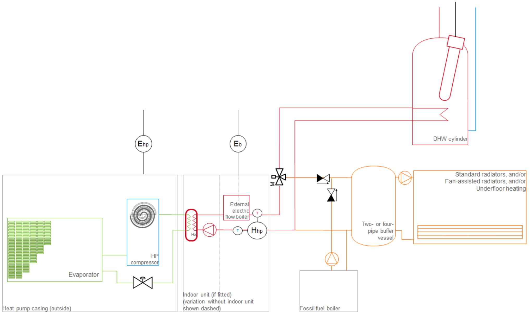
**Figure 11: Split-system air-source heat pump with metering option 1: 1 heat meter (integrated), 2 electricity meters**
