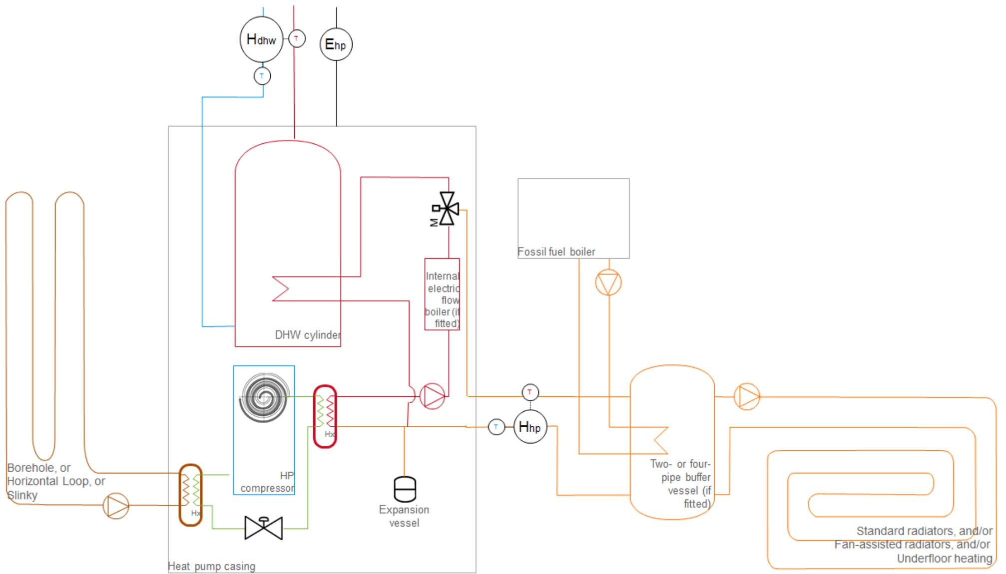
**Figure 7: Ground-source heat pump with integrated domestic hot water cylinder and metering option 1: 2 heat meters, 1 electricity meter**
