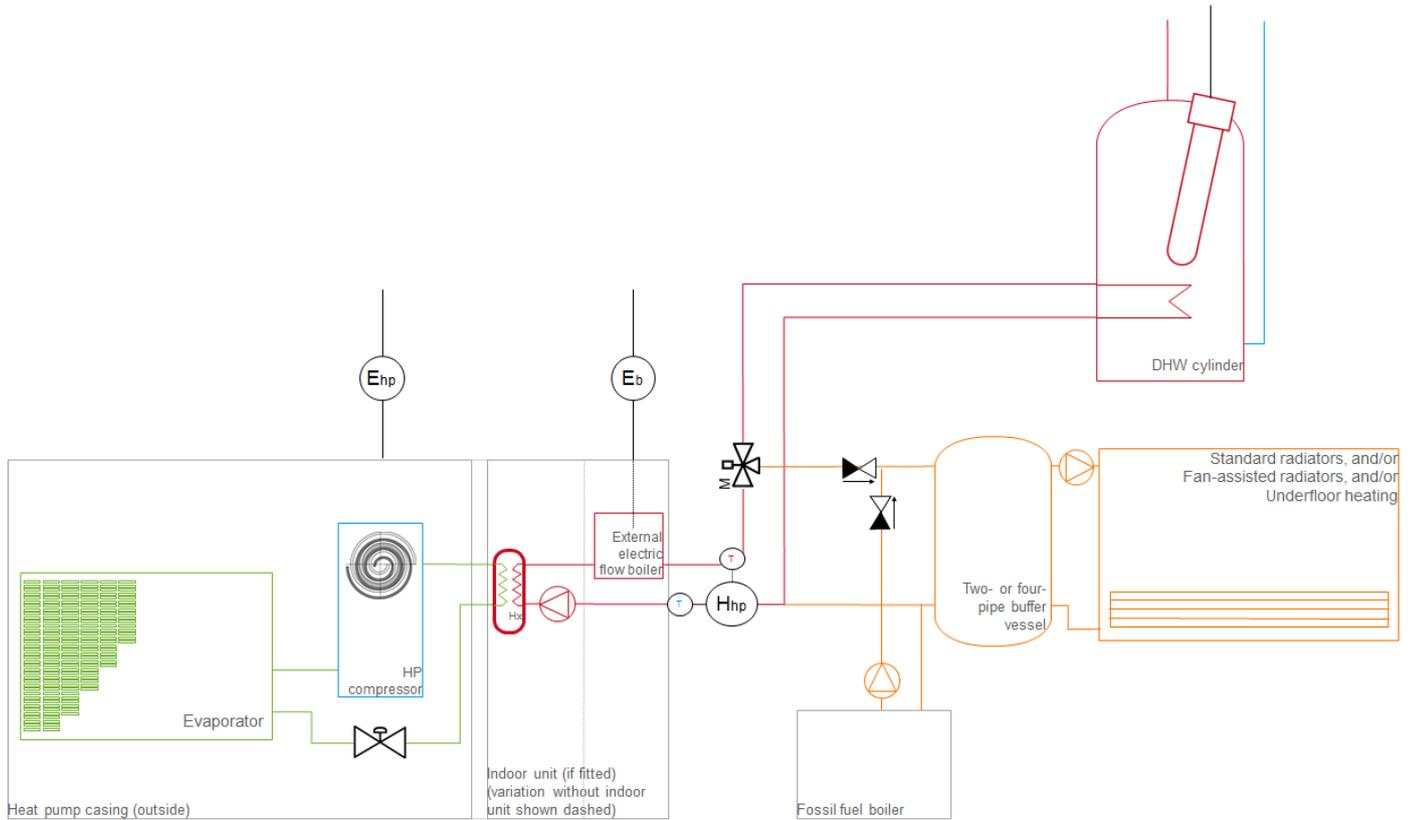
**Figure 10: Split-system air-source heat pump with metering option 1: 1 heat meter, 2 electricity meters**
