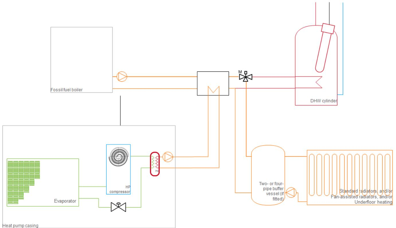
**Figure 3: Air-source heat pump with back-up fossil fuel boiler**
