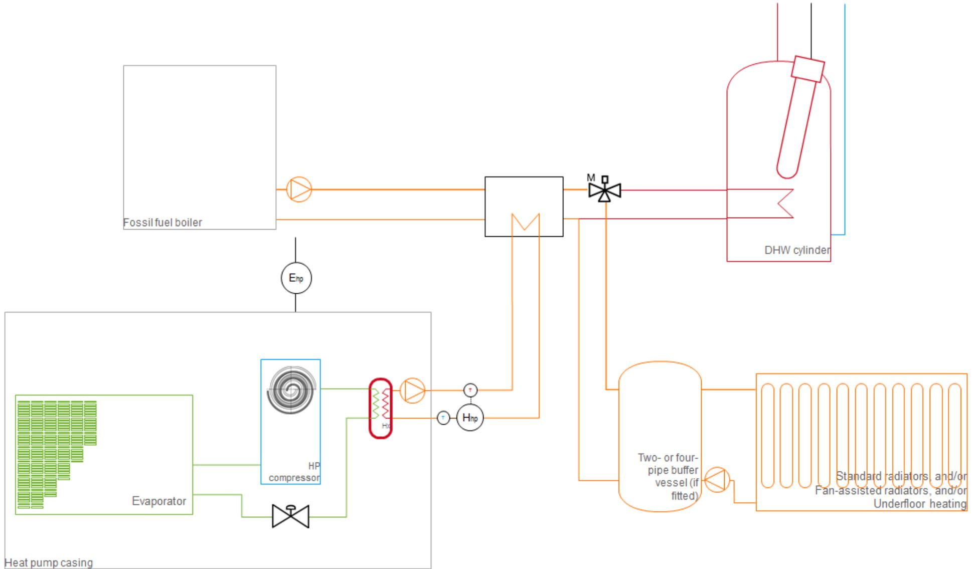
**Figure 4: Air-source heat pump with back-up fossil fuel boiler showing metering option 1: 1 heat meter and 1 electricity meter**
