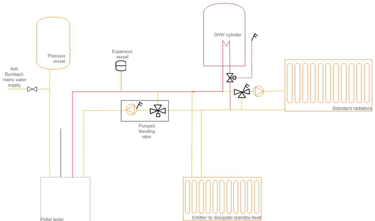
**Figure 1: Pellet biomass boiler**
