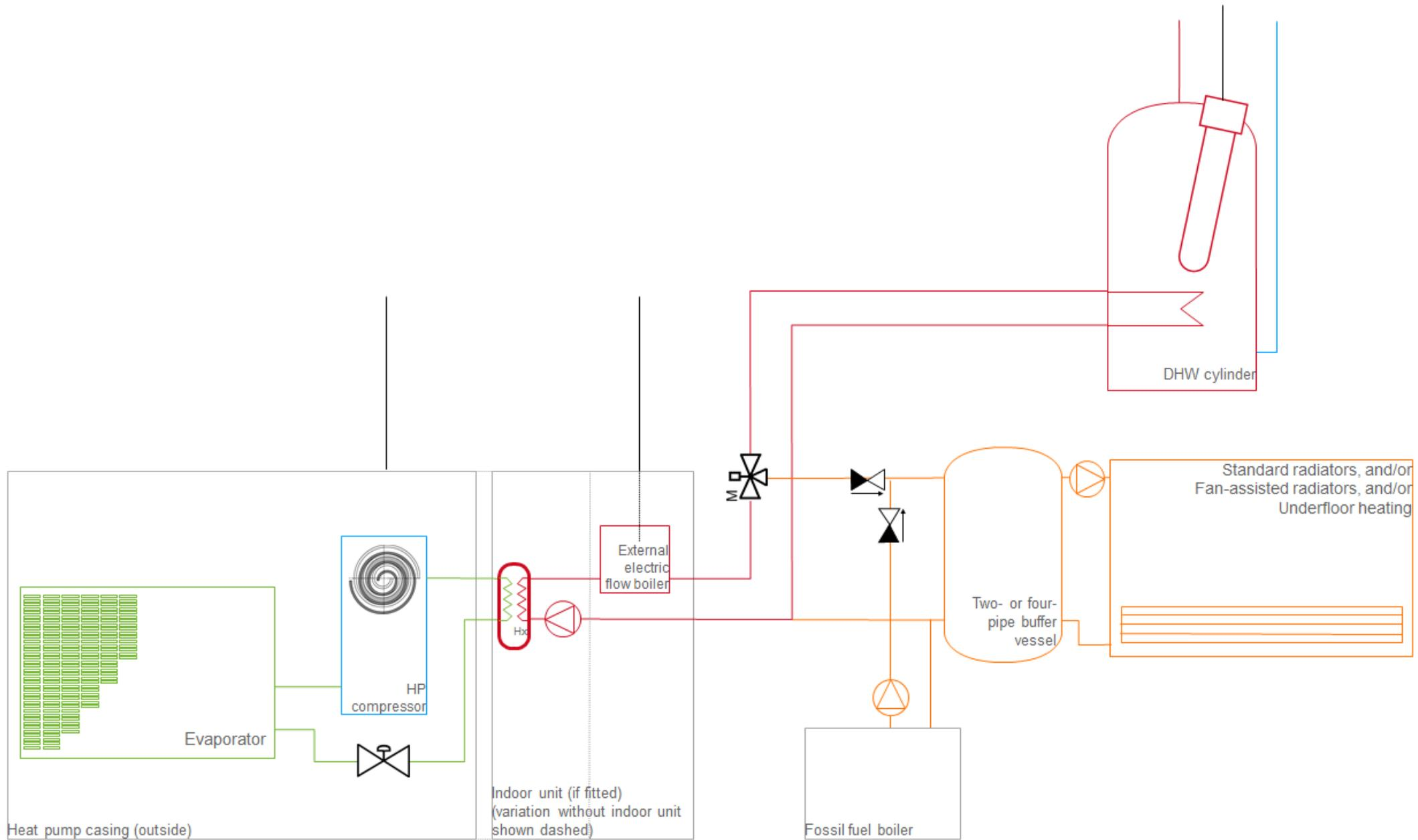
**Figure 9: Split-system air-source heat pump providing space heating and hot water**
