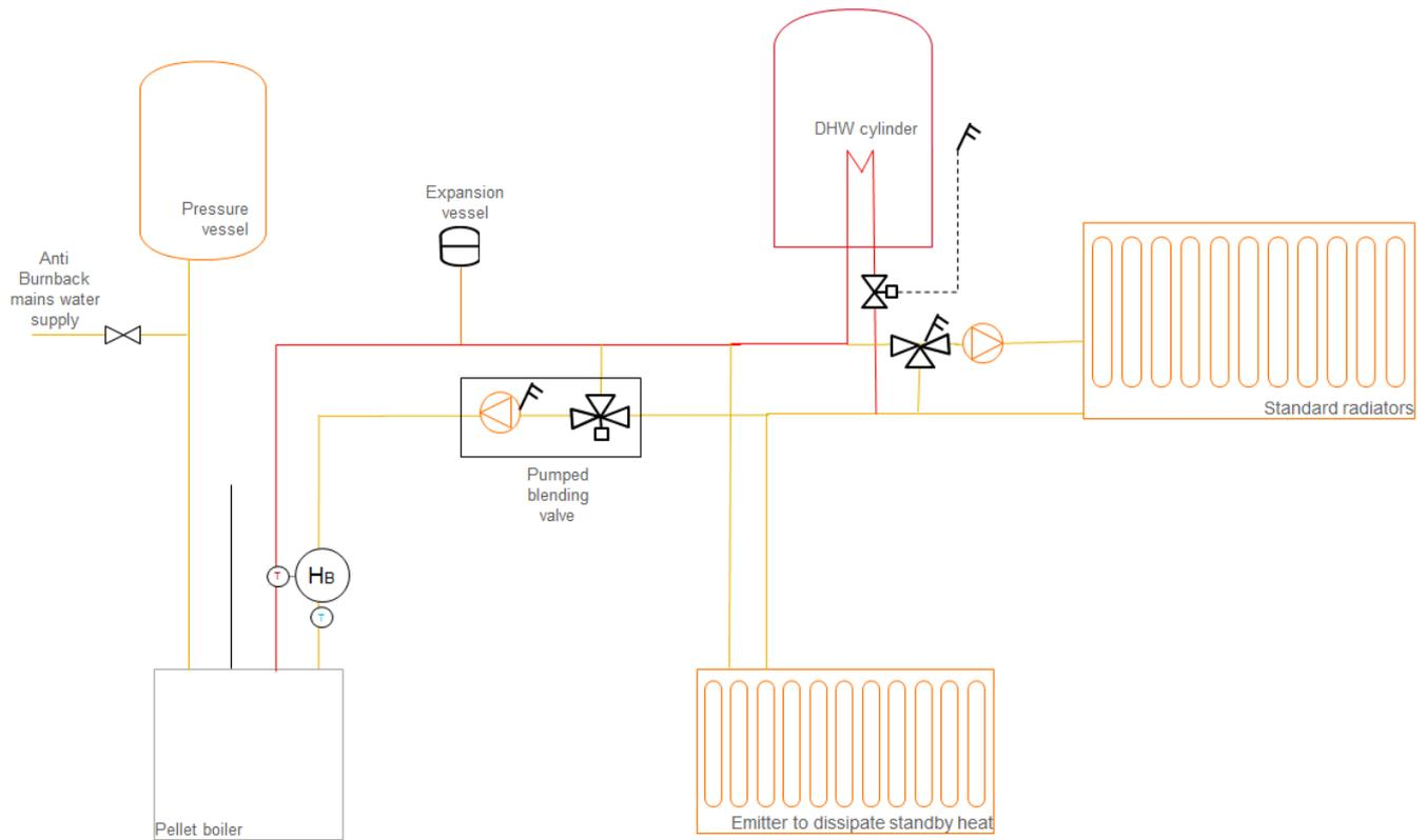
**Figure 2: Pellet biomass boiler with metering option 1: 1 heat meter**
