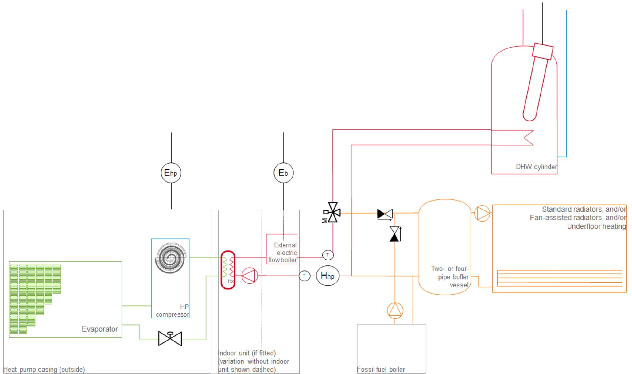
**Figure 10: Split-system air-source heat pump with metering option 1: 1 heat meter, 2 electricity meters**
