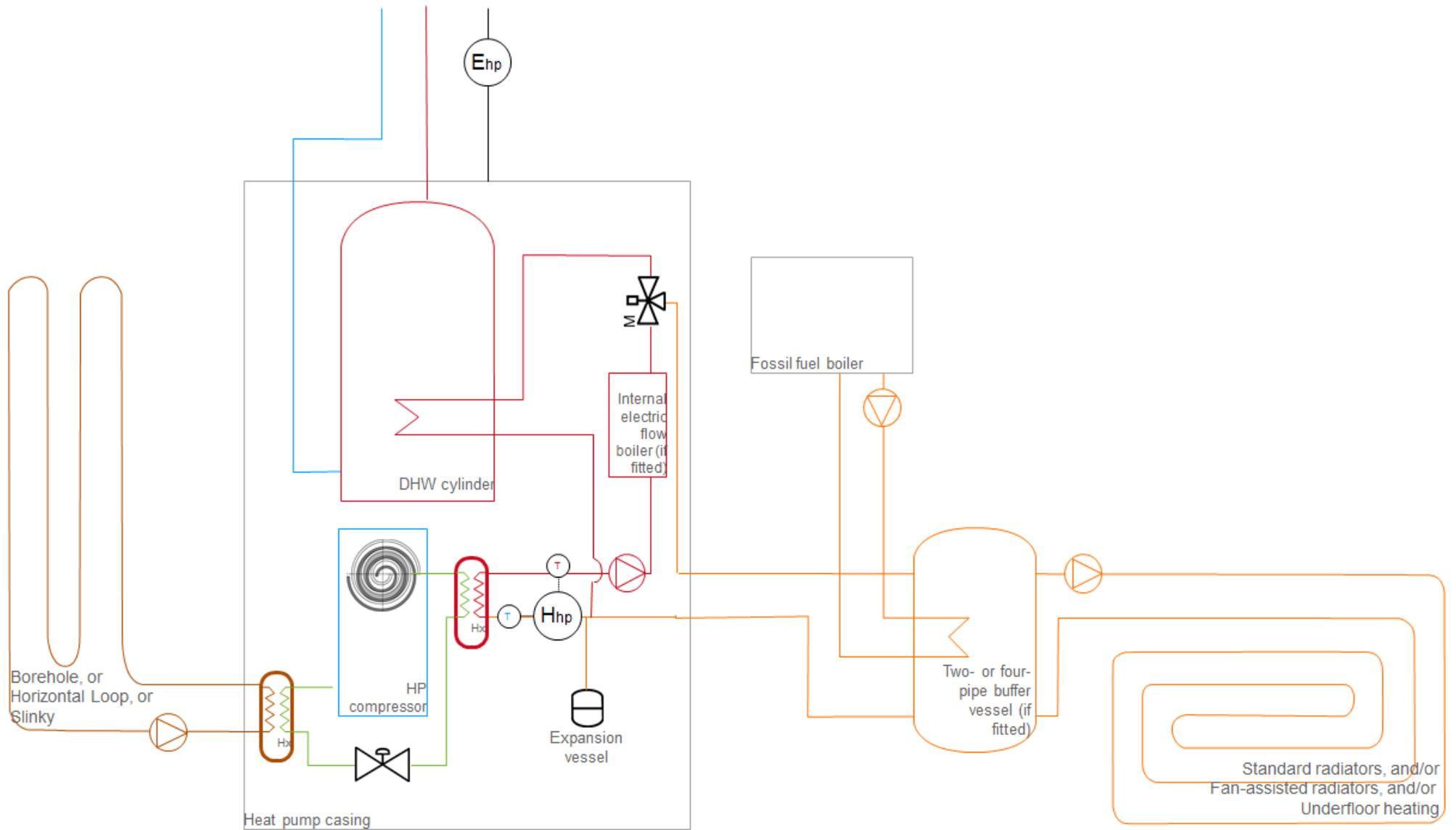
**Figure 8: Ground-source heat pump with integrated domestic hot water cylinder and metering option 2: 1 heat meter, 1 electricity meter**
