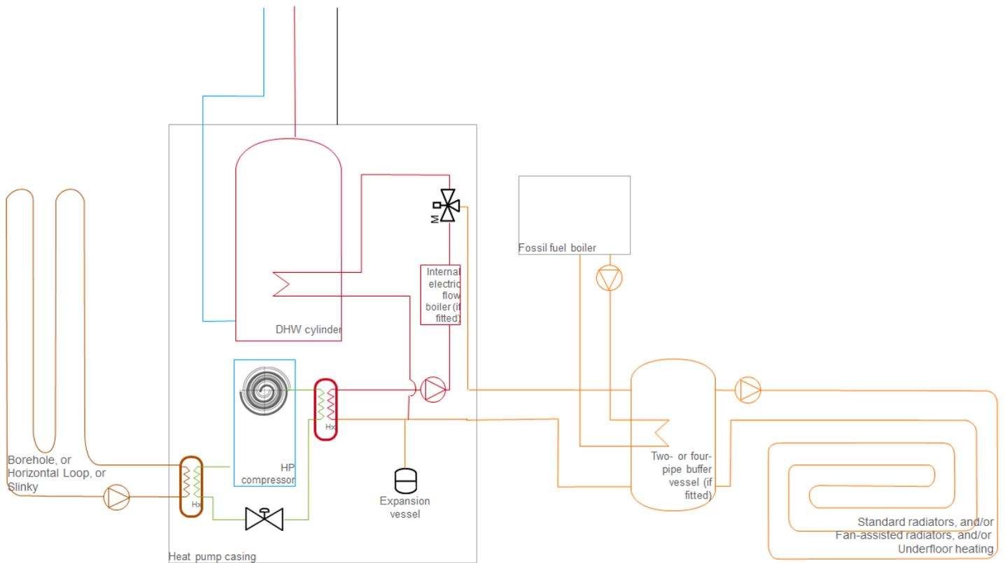
**Figure 6: Ground-source heat pump with integrated domestic hot water cylinder**
