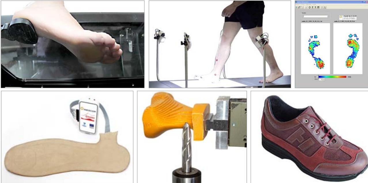
The scanner, gait analysis system, sensor system, machining process and finished bespoke Sshoe.
