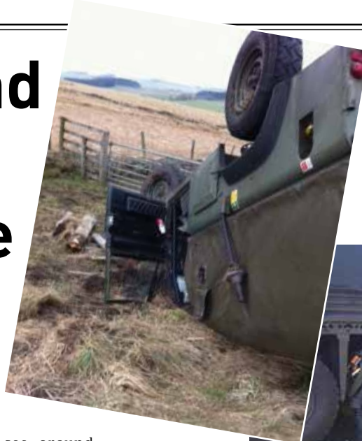
Left and below: roll-over protection in action – personnel escaped serious injury after their vehicles were involved in road accidents, thanks to Remus-fitted protection (High Specification) Truck
