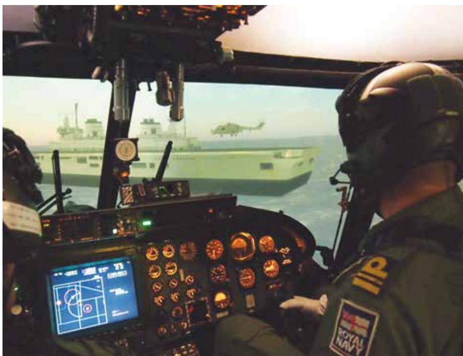
Touchdown: a Royal Navy crew brings a Lynx towards a carrier while operating the new Medallion 6000 simulator at RNAS Yeovilton
