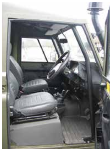
Above: Front Roll Over Protection System and acoustic matting fitted in the front compartment
