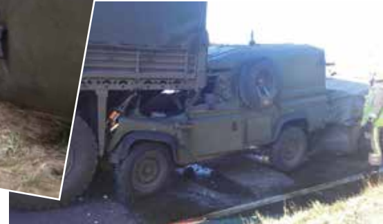
Left and below: roll-over protection in action – personnel escaped serious injury after their vehicles were involved in road accidents, thanks to Remus-fitted protection (High Specification) Truck
