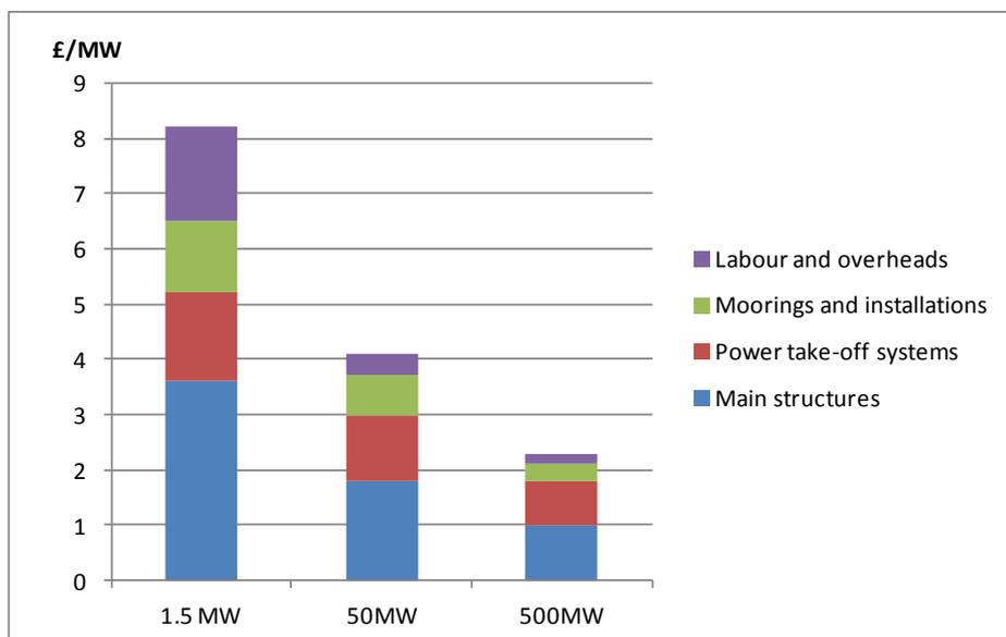
Figure 21 - Cost Reduction Profile for Pelamis Wave Device
