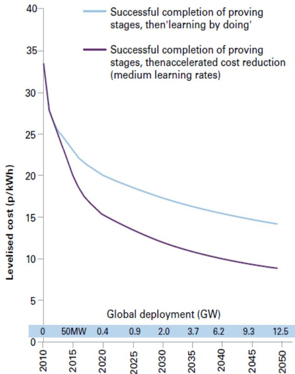
Figure 20 - Predicted levelised cost reduction for tidal energy<sup>69</sup>
