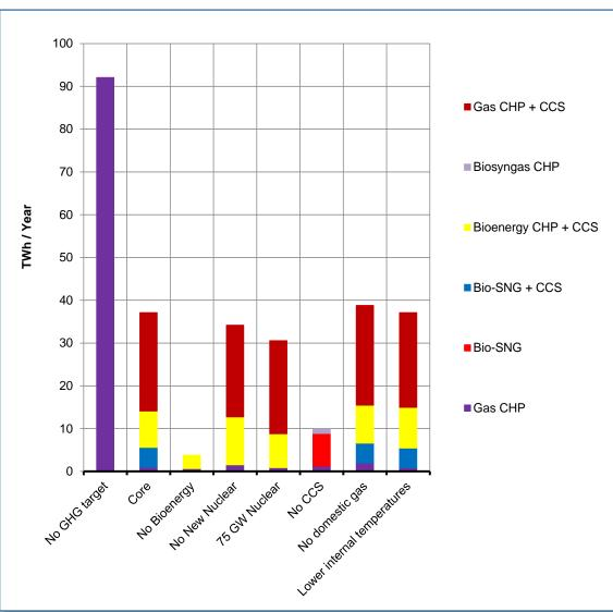
The mix of industry heat network supply options in 2050 does not change significantly across the sensitivities, focusing primarily on gas CHP with CCS, and to a lesser extent bioenergy and CCS routes. The key exceptions are the no CCS and no bioenergy sensitivities.
