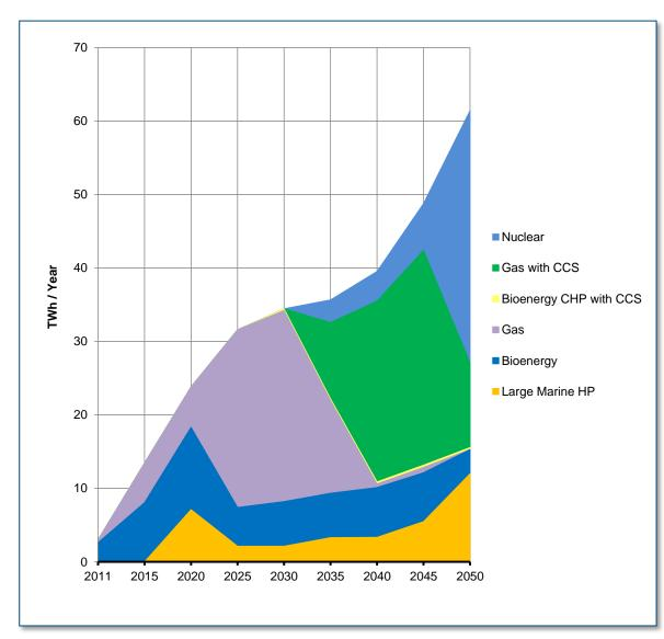
The core scenario shows heat networks supplying around 60 TWh of heat to buildings by 2050. Heat networks grow rapidly to 2030, with the majority of heat being supplied by gas sources through large scale CHP, but complemented with around a quarter of heat from biomass.
