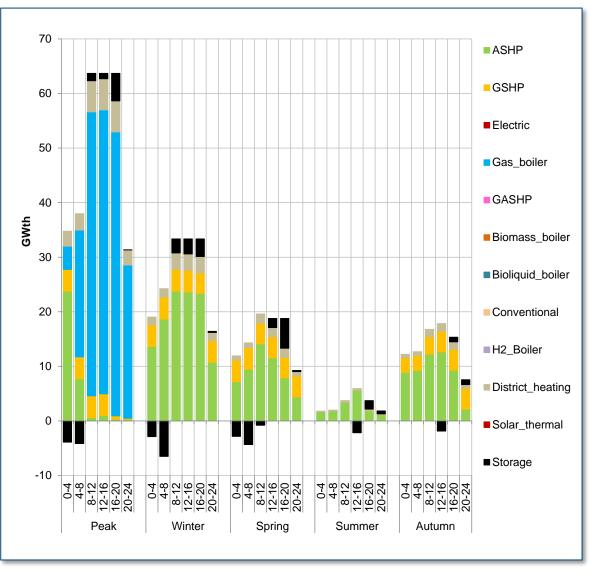
In a similar manner to the domestic sector, this chart shows the profile of the supply of heat demand (for space heat and hot water) in 2050 for each characteristic day modelled.
