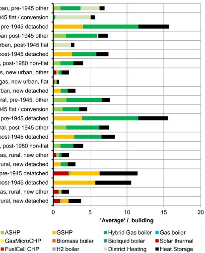
The chart shows the average mix of installed heating capacity by dwelling type. It is important to note that this does not imply that each individual building within each characteristic segment has this mix of technologies, but is illustrative of the broad preference for technology types by segment.
