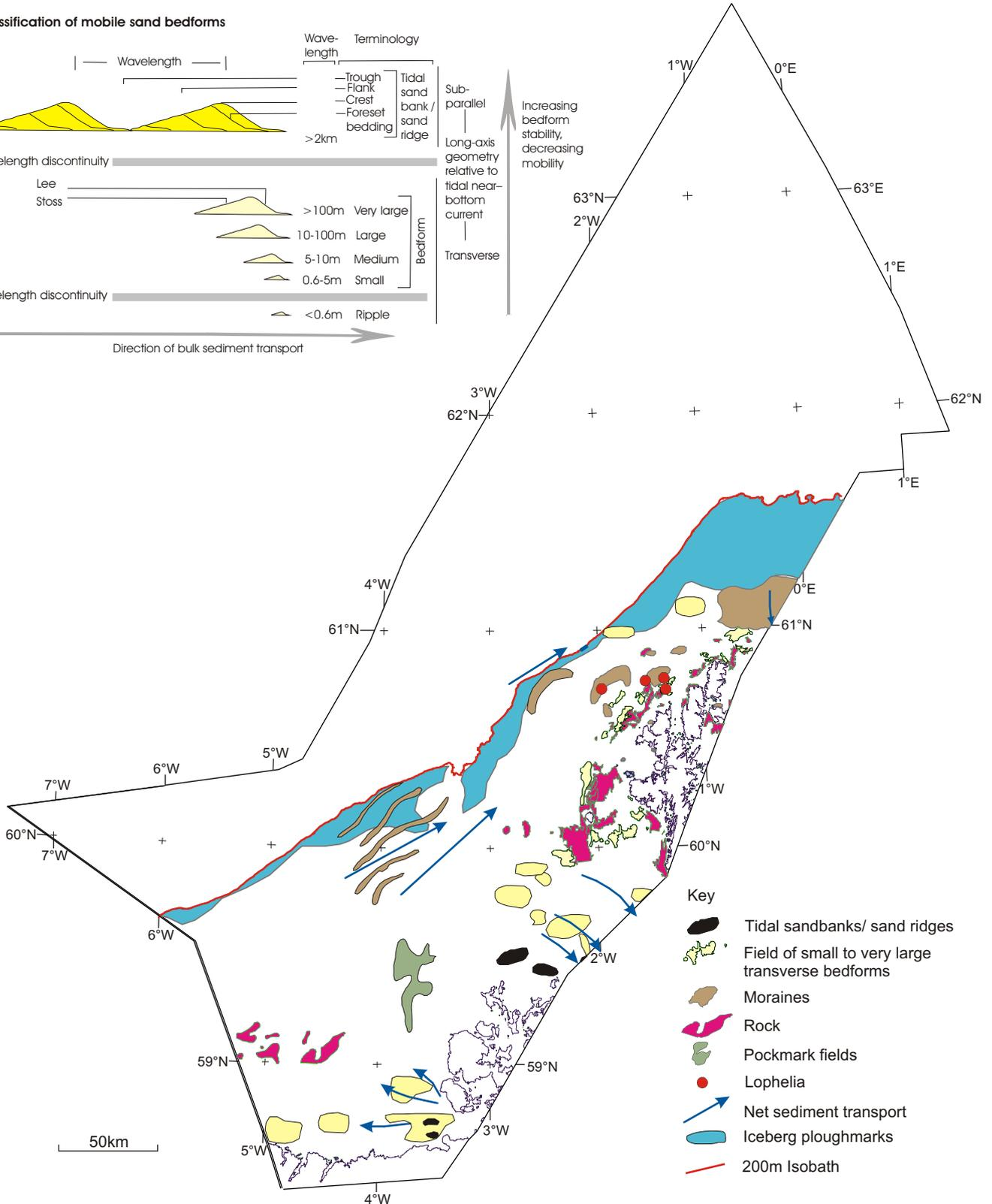
**Figure 6 Seabed bedforms and net sand transport directions**
