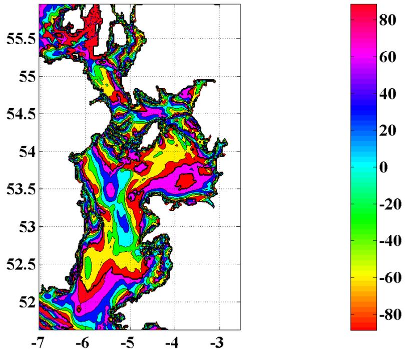
Figure 5. Phase difference between  $M_2$  currents and elevations (degrees).
