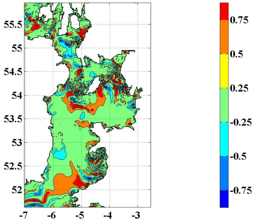
Figure 6.  $M_2$  tidal current ellipse eccentricity (ratio of minimum to maximum amplitude).
