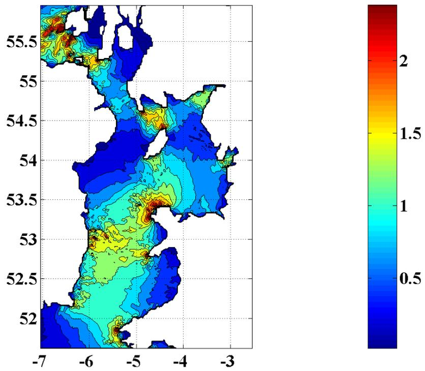
Figure 4. Maximum amplitude of the depth-averaged current for a mean spring tide ( $\text{m s}^{-1}$ ).
