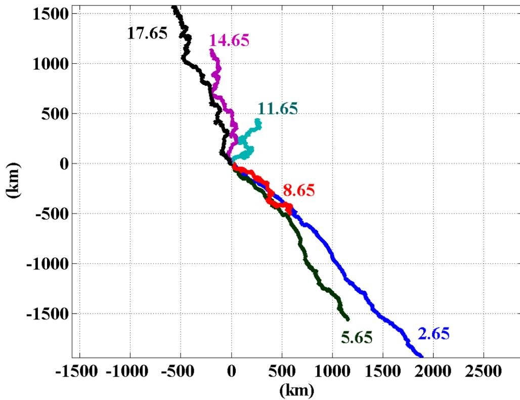
Figure 20. Progressive vector diagram showing mean currents from a 2-year record by the Mersey Bar Light. The figures denote measurement height (m) above the bed. The water depth at the site varies between 18.5 and 28.5 m, depending on the tide. (In one year water moving at  $0.01 \text{ m s}^{-1}$  will travel 315 km.)
