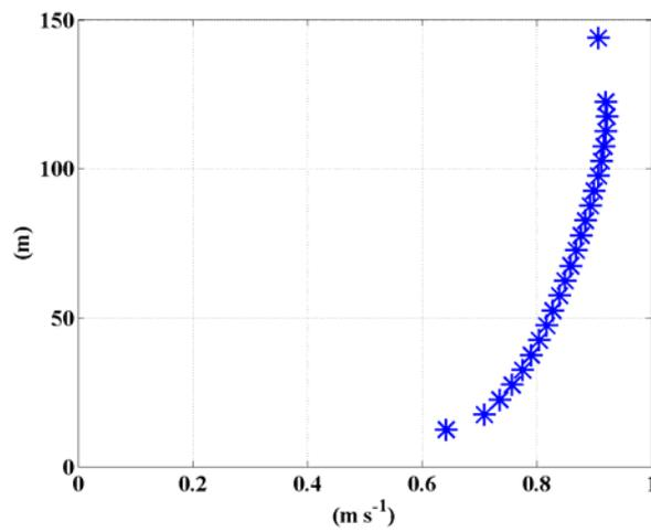
Figure 9. Variation with height above the bed of the maximum  $M_2$  current amplitude ( $\text{m s}^{-1}$ ) in the North Channel,  $54^\circ 46' \text{N}$   $5^\circ 24' \text{W}$  in 142 m of water.
