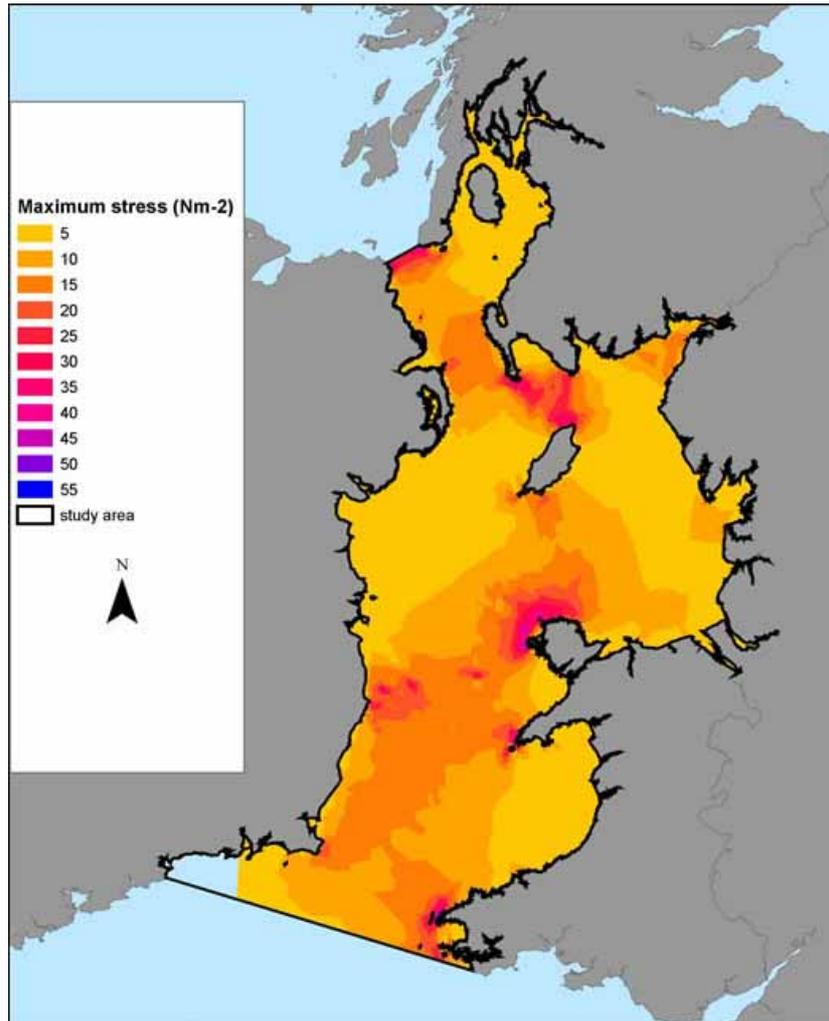
Figure 7. Maximum bed stress in Pa from a numerical model run for the years 1995 to 1997 forced both by tides and winds, but with no wave contribution (JNCC, 2004).
