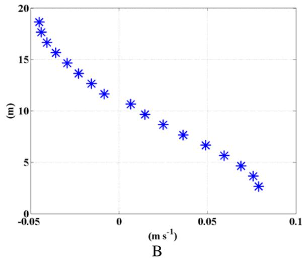
Figure 8. Variation with height above the bed of the  $M_2$  current amplitude ( $\text{m s}^{-1}$ ) at the Mersey Bar Light a) Maximum b) Minimum, positive anti-clockwise.
