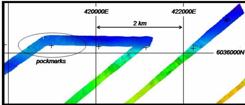
Figure 11: Pockmarks on Cruise A MBES data. The location is indicated on Fig. 10.
