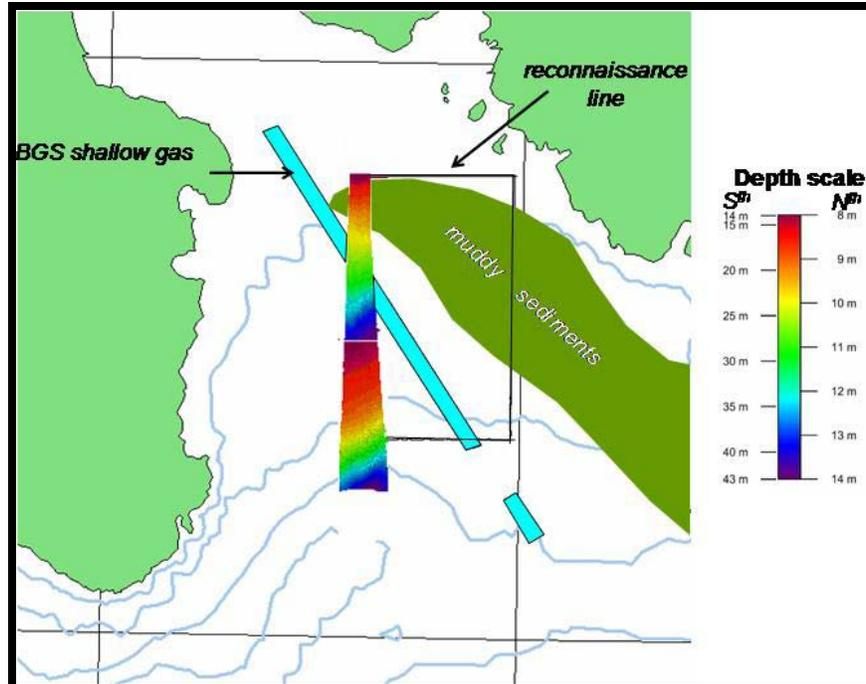
Figure 12: Wigtown Bay survey area showing MBES bathymetry. Weather and sea conditions permitted no coverage of the area with muddy sediments (muds, sandy muds, and muddy sands) other than the reconnaissance lines indicated.
