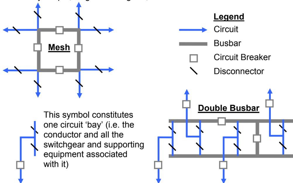
Figure A1-7: Mesh and Double Busbar Configurations
