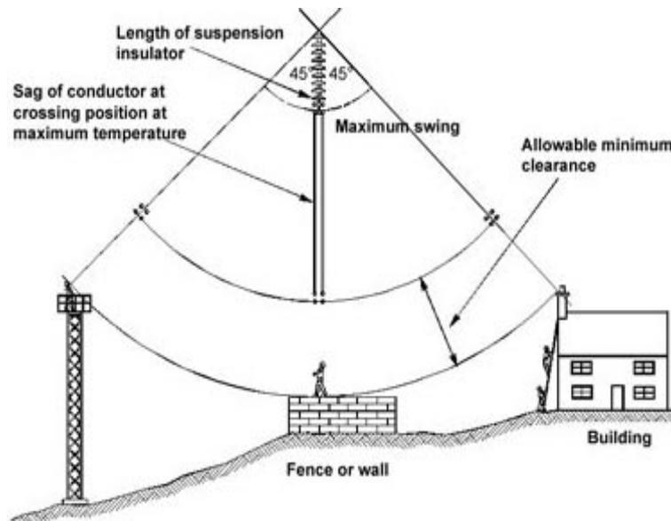
Figure A1-28 Safety Clearance to Objects (on which a person can stand)
