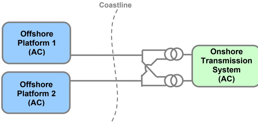
Figure A1-16: Assumed Sharing of Assets forming part of the Offshore Transmission System
