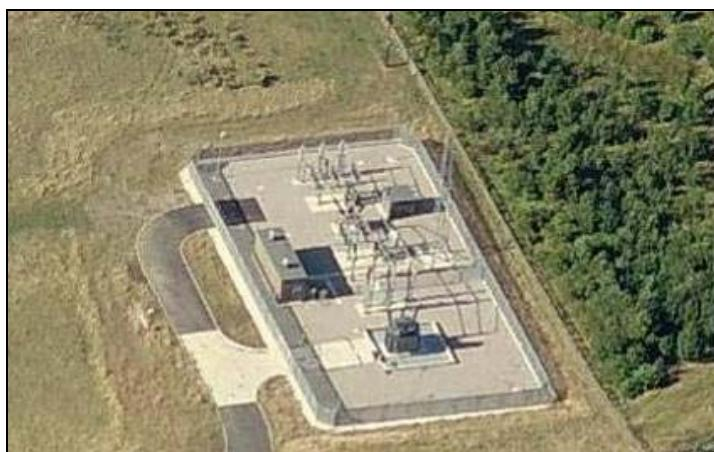
Figure A1-15: Round 1 Offshore Wind Generation 132kV Cable Termination Compound (no transformers required)
