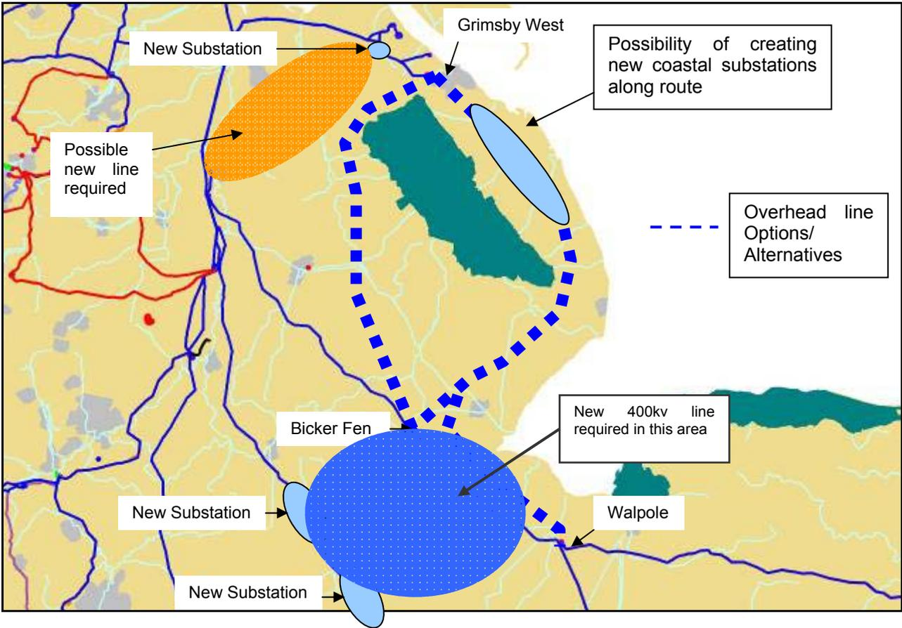
Figure 16 – Potential New Overhead Line Requirements in Lincolnshire
