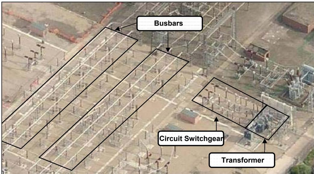
Figure A1-1: Busbars, Switchgear and Transformers
