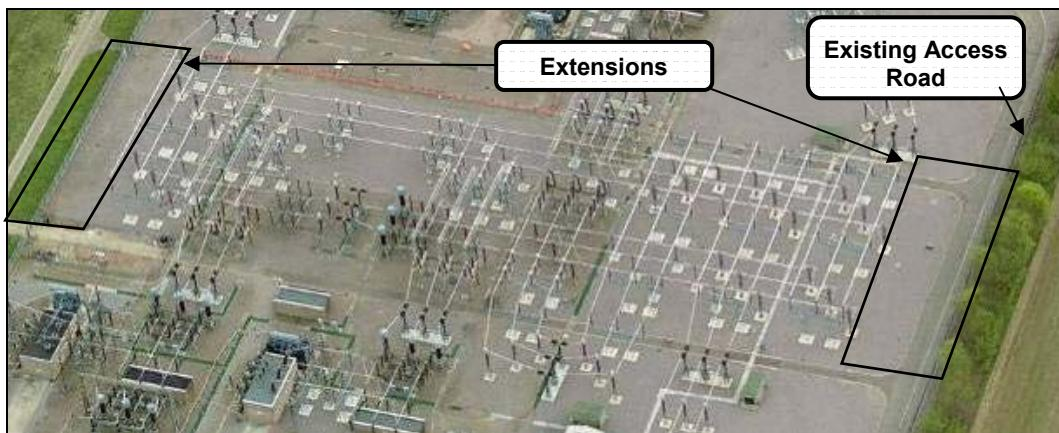
Figure A1-8: Location of Substation Extensions
