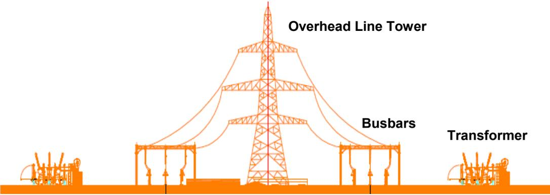
Figure A1-26 Relative Size of Substation Equipment and Overhead Line Towers
