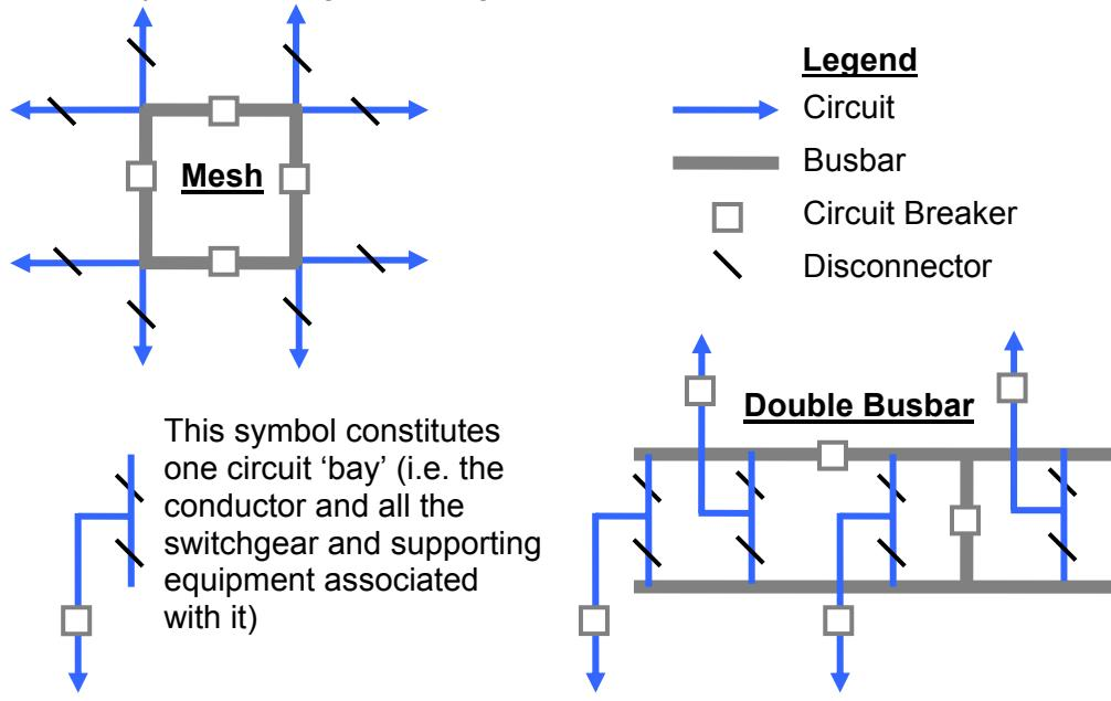
Figure A1-7: Mesh and Double Busbar Configurations
