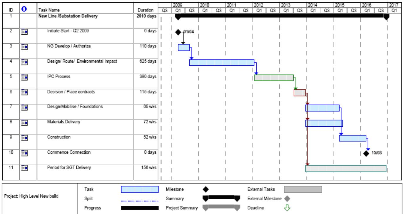
Figure A3-1 – Overview of Programme for New Overhead Line and Substation Deliver with IPC
