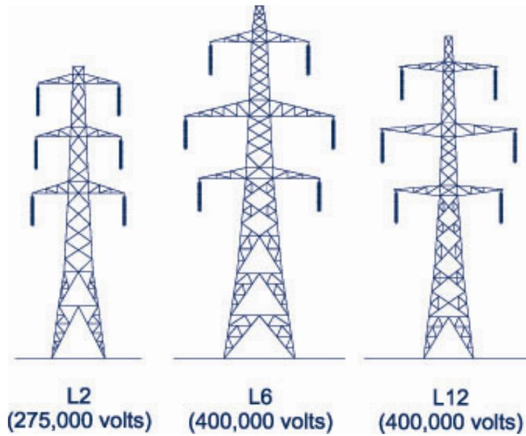
Figure A1-23: Typical Suspension Towers
