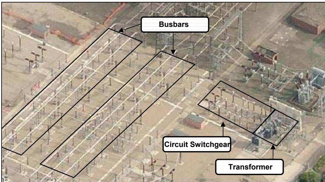
Figure A1-1: Busbars, Switchgear and Transformers
