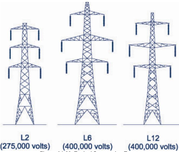
Figure A1-23: Typical Suspension Towers
