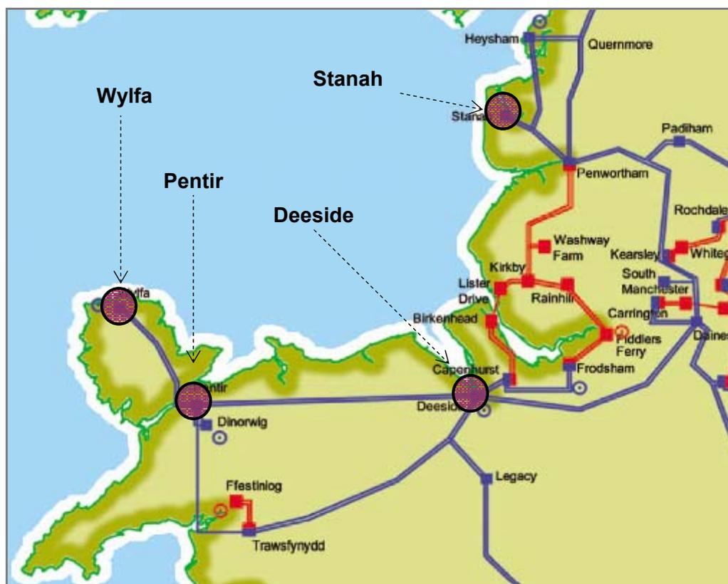
Figure 22 – Onshore Transmission System in North Wales and the North West
