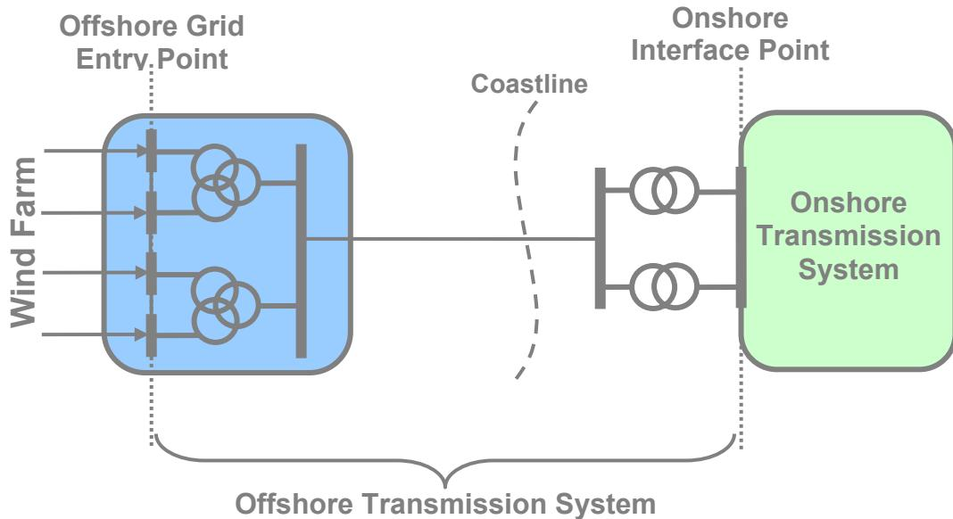
**Figure 8 – Extent of an Offshore Transmission System**
