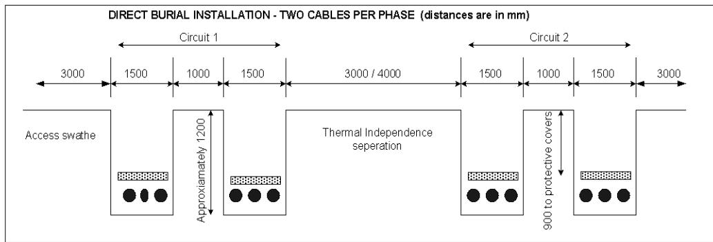
Figure A1-20: Example of Separation Distances Required for Underground Cable
