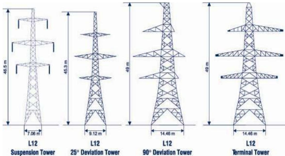
Figure A1-24: Typical Towers in a 400kV Route (L12 example)
