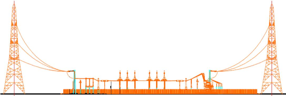
Figure A1-25 Relative Size of Substation Equipment and Overhead Line Towers
