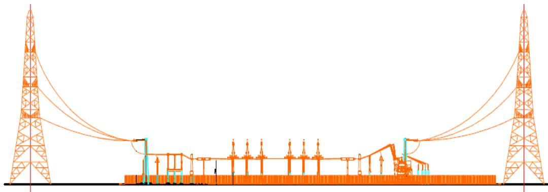
Figure A1-25 Relative Size of Substation Equipment and Overhead Line Towers
