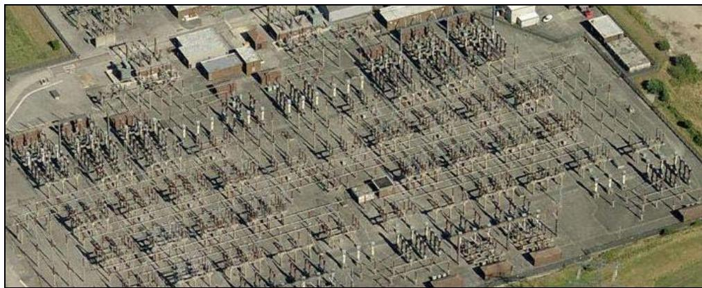
Figure A1-2: Aerial view of typical outdoor, AIS substation
