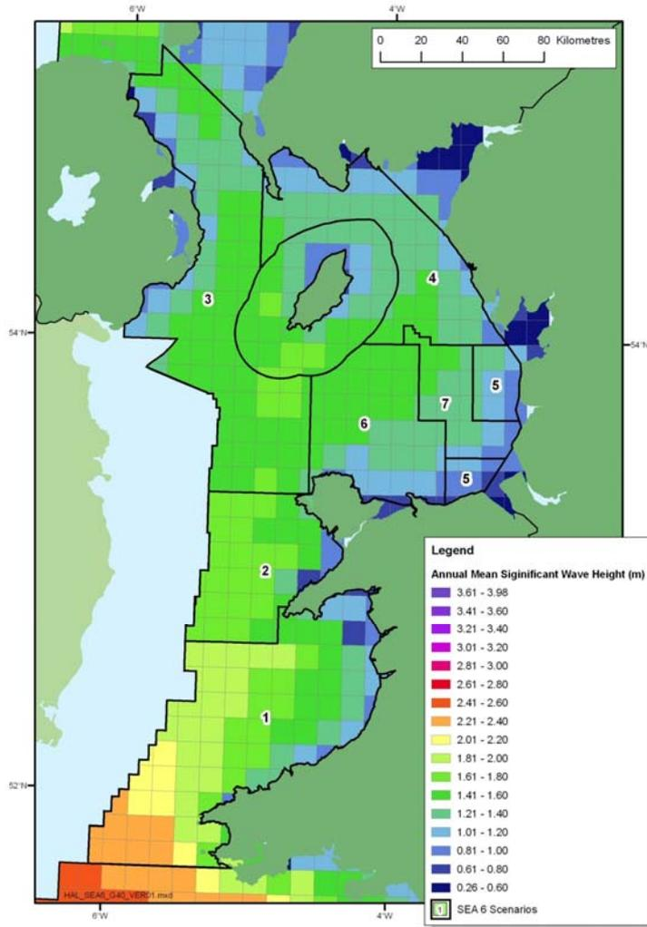
Figure 5.20 – Annual mean significant wave height
