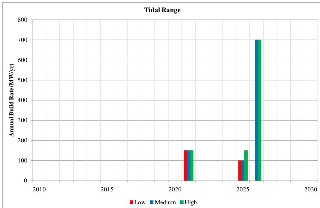
**Figure 44: UK Tidal Range Annual Build Rate (MW/yr)**
