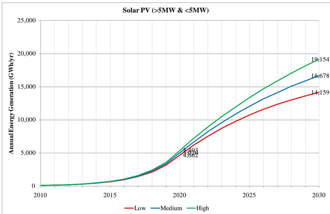
**Figure 56: UK PV Annual Energy Generation >5MW & <5MW (GWh/yr)**
