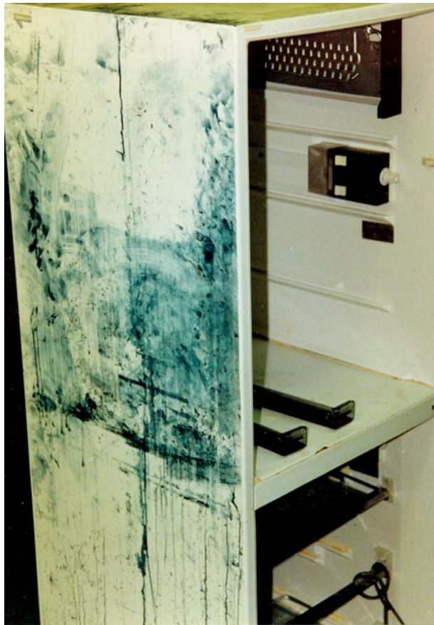
Contaminated fridge treated using iodine fuming followed by fixing with \alpha -naphthoflavone.
