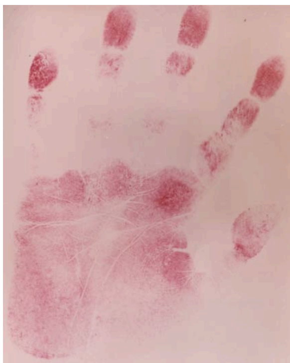
Palm print developed using 4-dimethylaminocinnamaldehyde solution.
