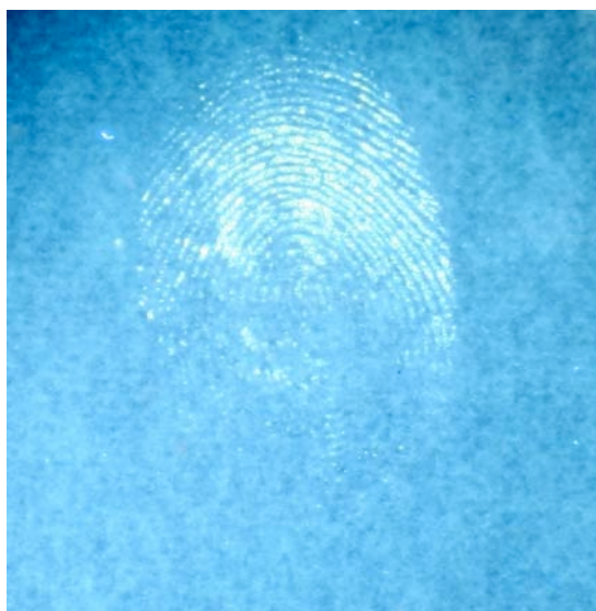
Fingerprint developed on filter paper using o-phthaldialdehyde.
