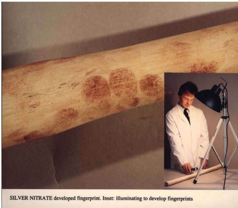
Development of fingerprints using silver nitrate.
