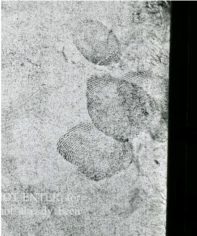
Fingerprints developed by electrostatic detection apparatus while processing a document.
