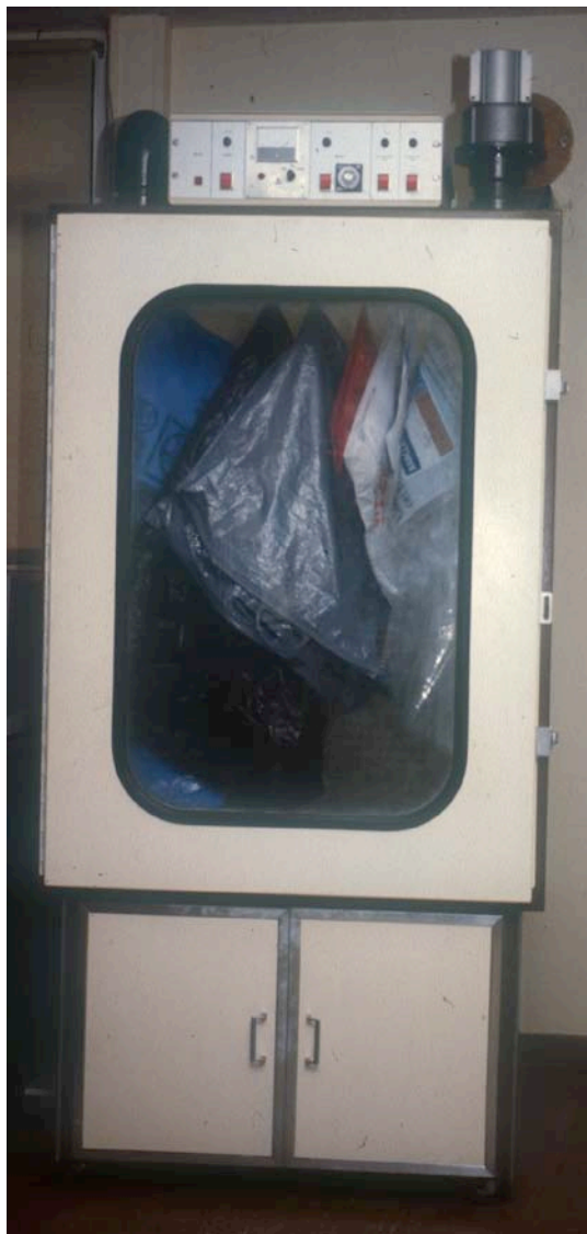
The prototype 'Sandridge' controlled-humidity superglue cabinet developed by the Police Scientific Development Branch.
