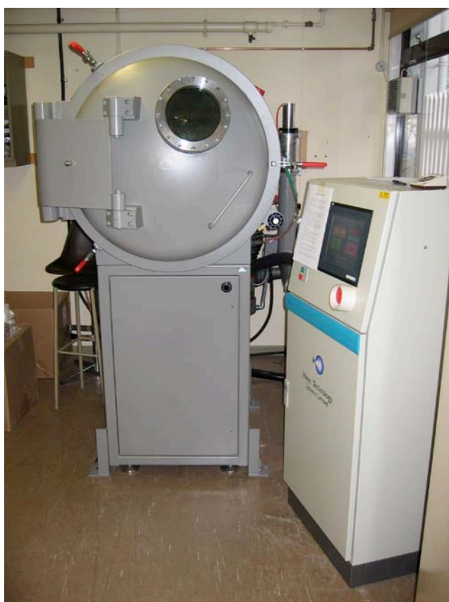
Typical vacuum metal deposition equipment.
