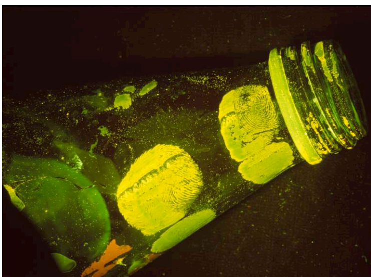
Fingerprints in blood on a dark glass bottle enhanced using acid yellow 7.
