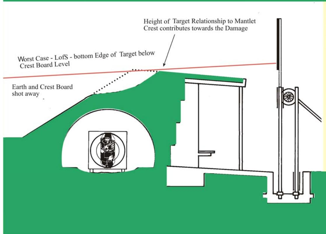
Figure 15-10. Crest Board Clearance and Mantlet Damage
