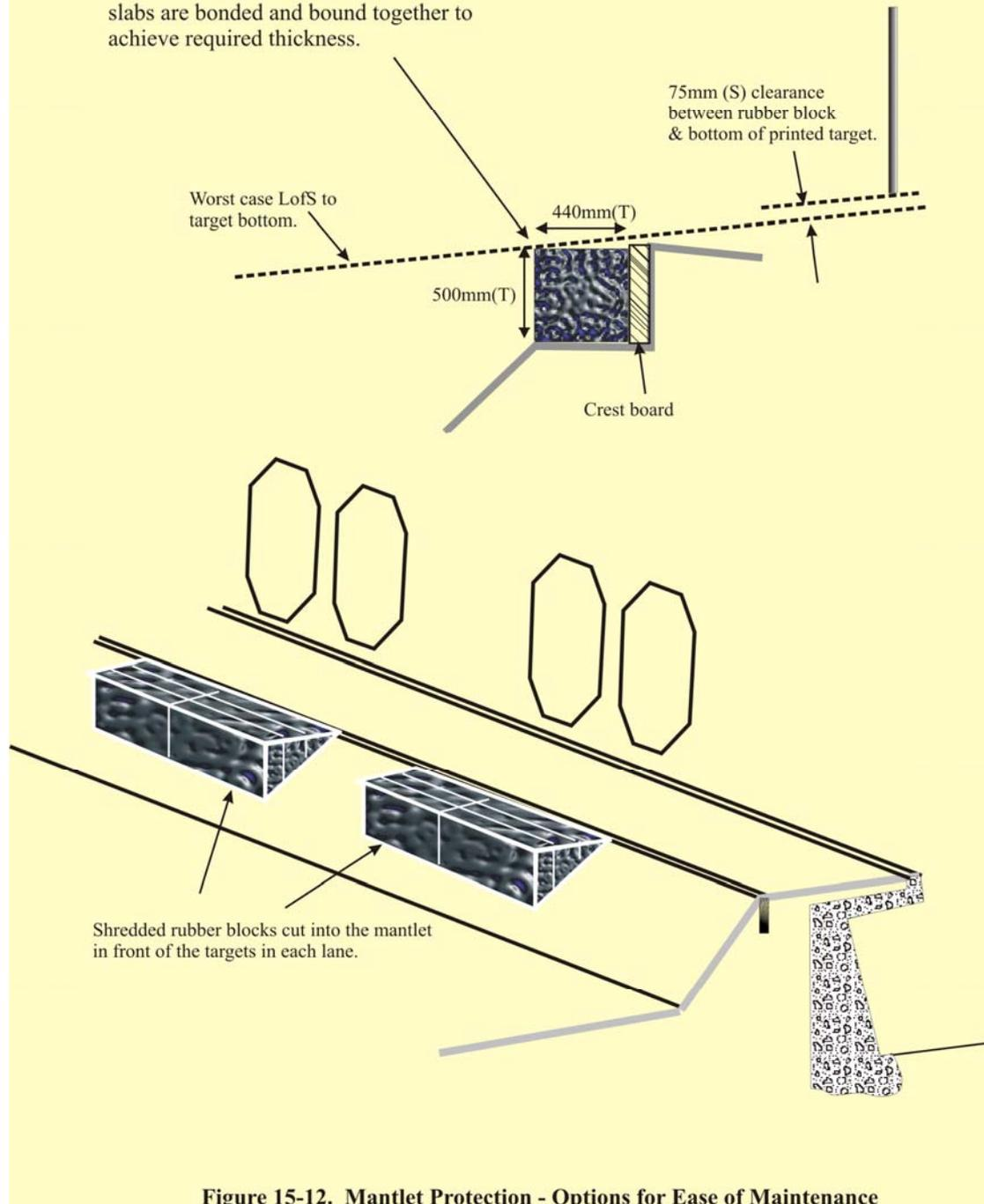
Figure 15-12. Mantlet Protection - Options for Ease of Maintenance
