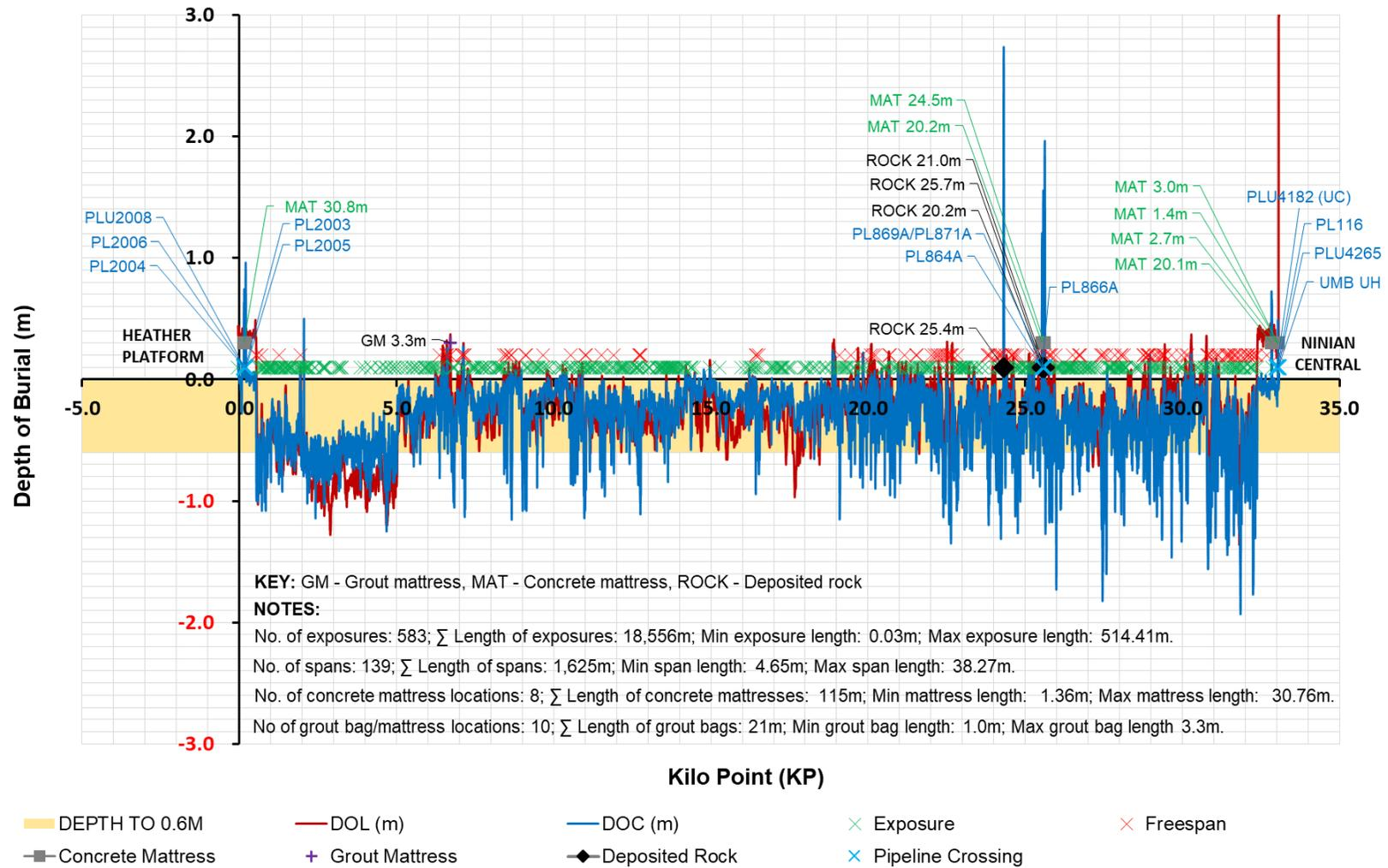
Figure 4.2.3: PL9 pipeline depth of burial profile (2010)<sup>4</sup>
