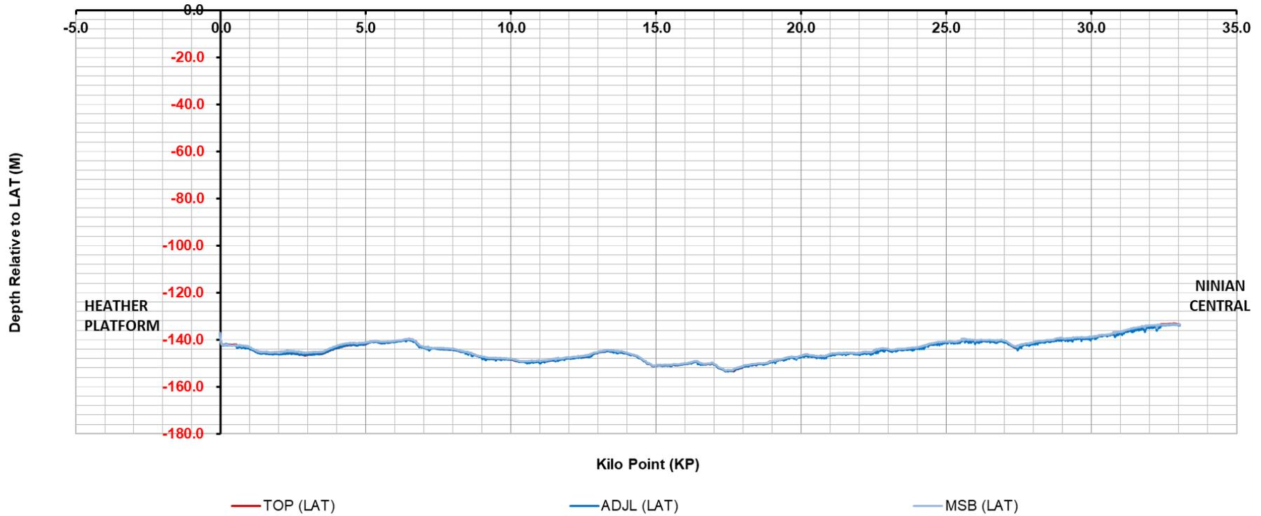
Figure 4.2.1: PL9 seabed & pipeline profile (2008)
