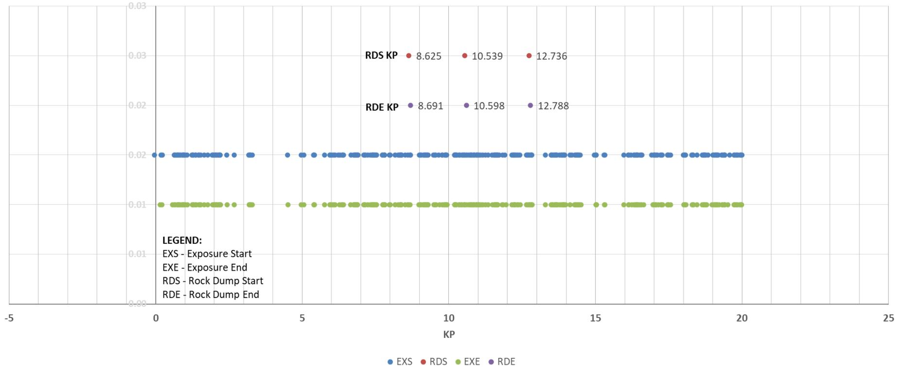
Figure B.1.1: PL9 rock vs. exposures plot KP0.0 to KP20.0 (2018 data)
