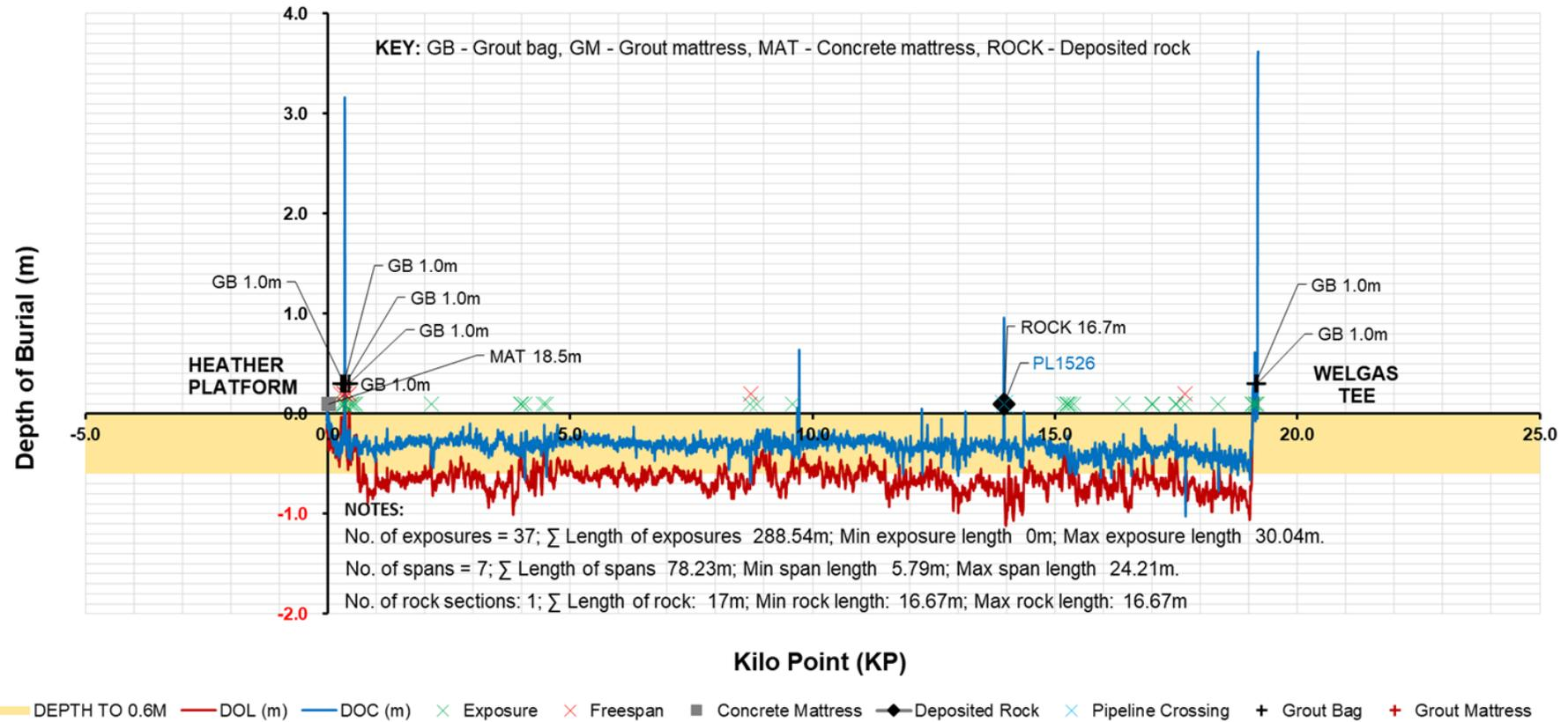
Figure 4.2.11: PL352 pipeline depth of burial profile (2010)
