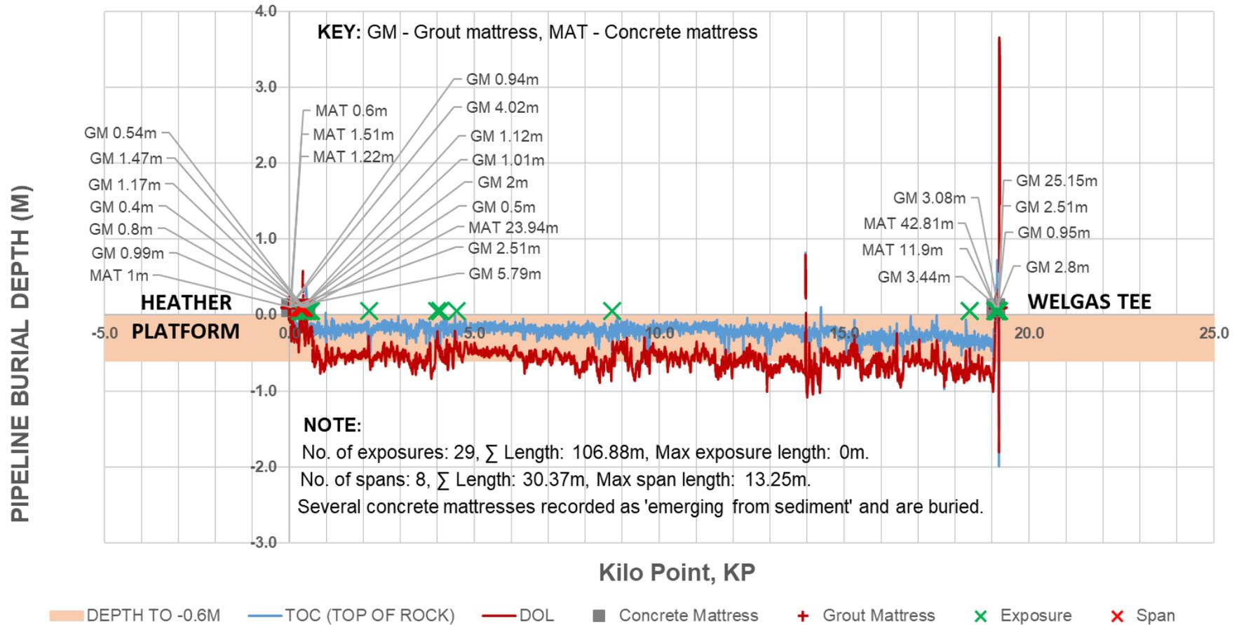
Figure 4.2.13: PL352 pipeline depth of burial profile (2018)
