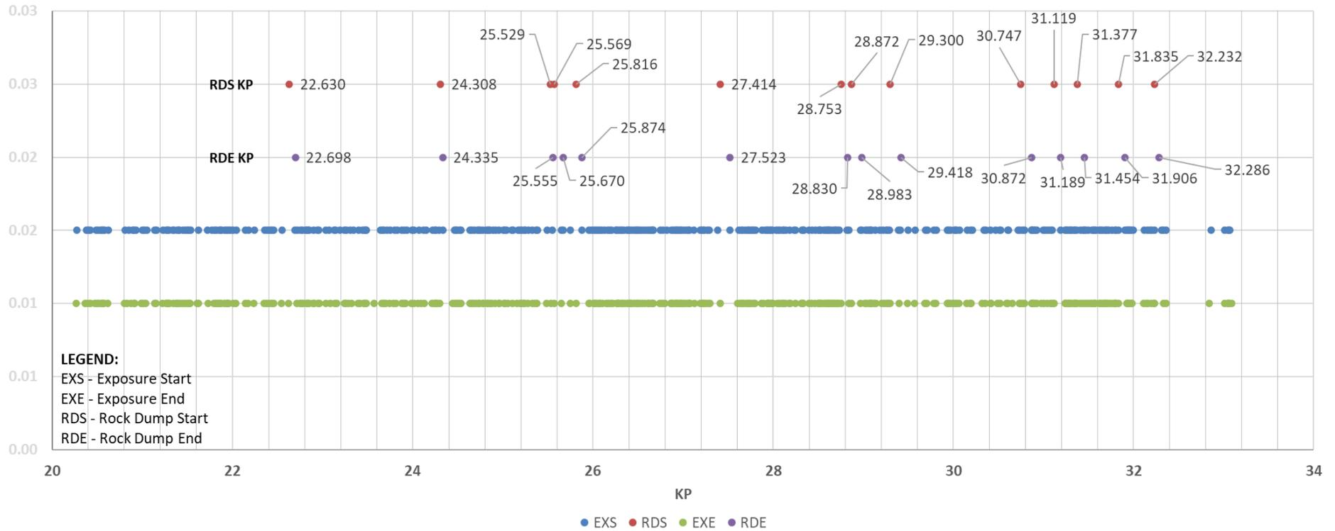
Figure B.1.1: PL9 rock vs. exposures plot KP20.0 to KP33.100 (2018 data)
