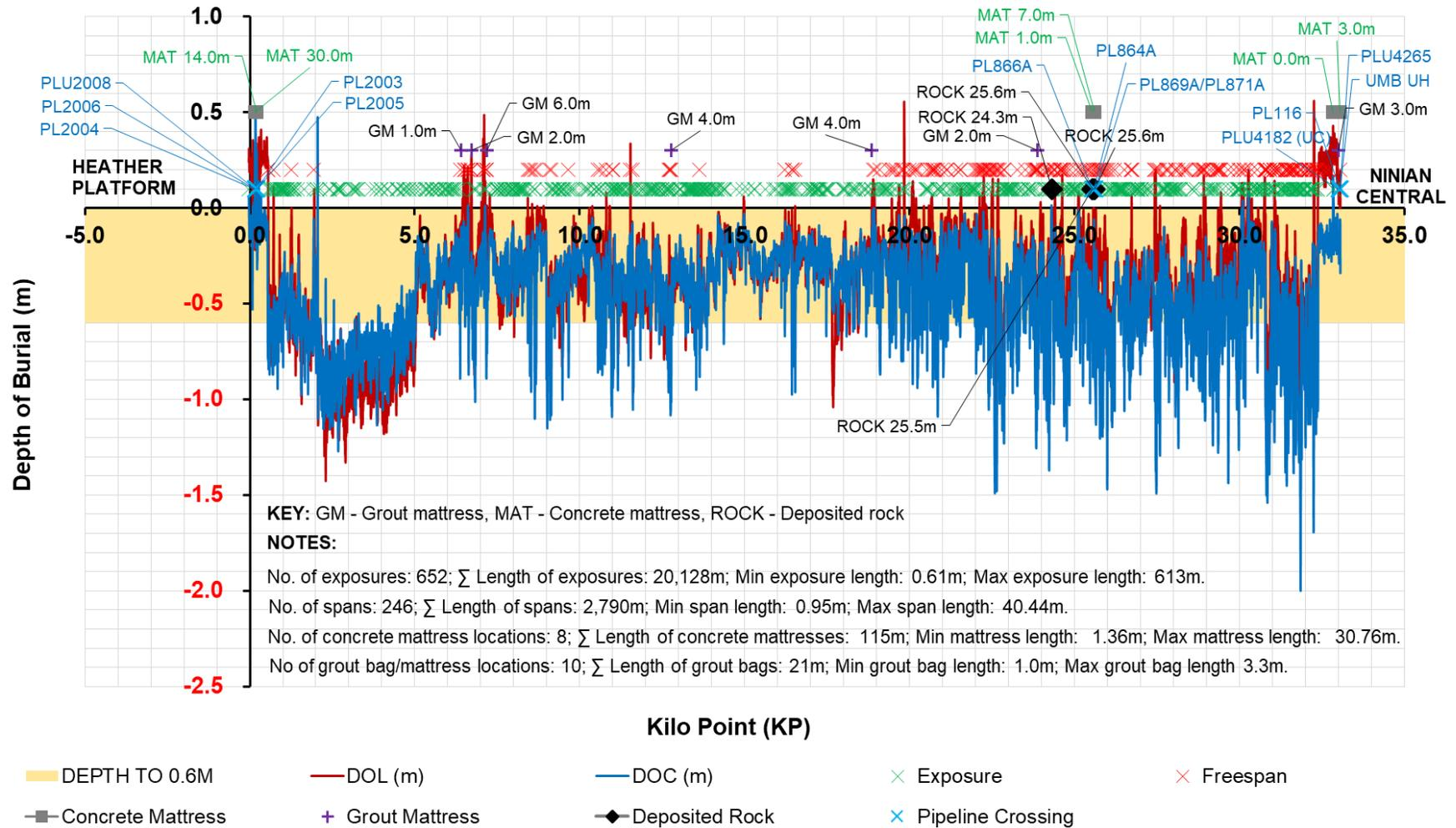
Figure 4.2.2: PL9 pipeline depth of burial profile (2008)<sup>4</sup>
