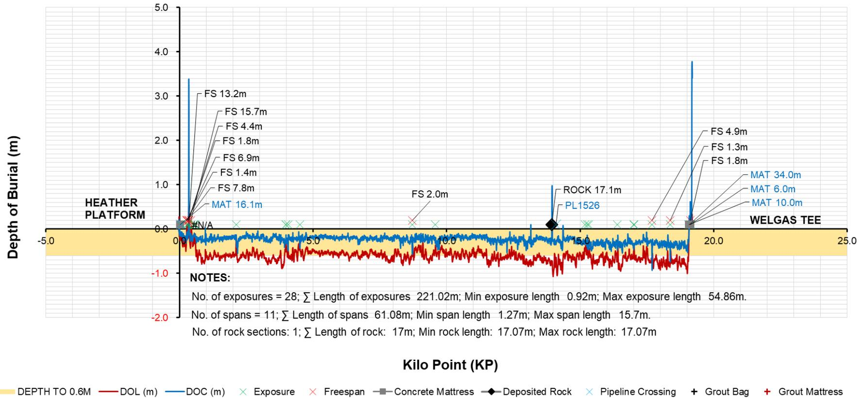
Figure 4.2.12: PL352 pipeline depth of burial profile (2014)
