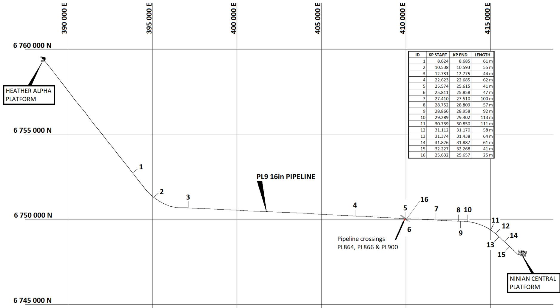
Figure 4.2.4: PL9 deposited rock for remediation of spans in 2010<sup>4</sup>
