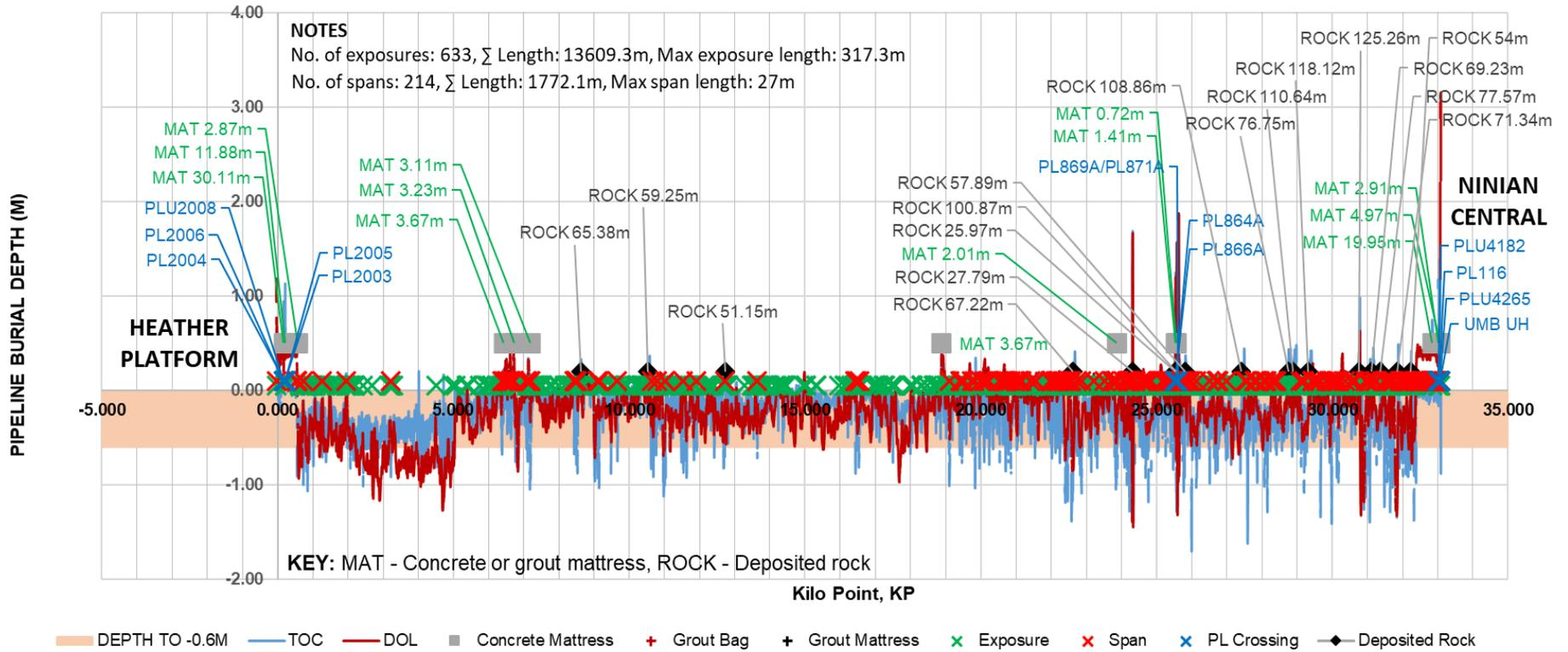
Figure 4.2.6: PL9 pipeline depth of burial profile (2018)<sup>4,5</sup>
