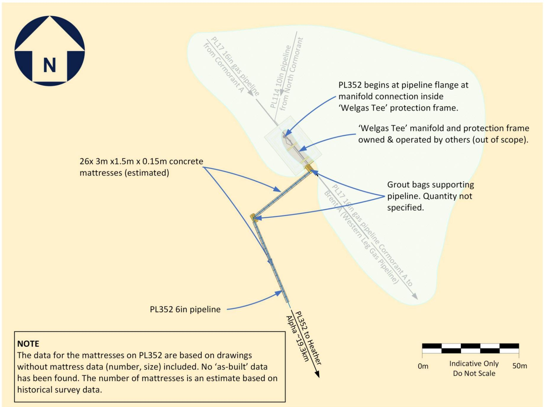
Figure B.2.1: Welgas tee / manifold approaches
