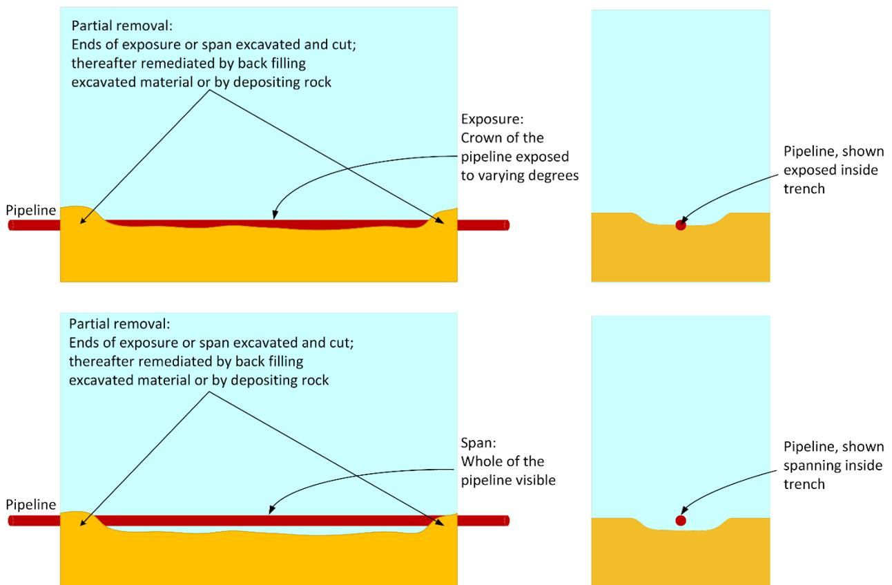
Figure 5.1.1: Exposures, spans & partial removal
