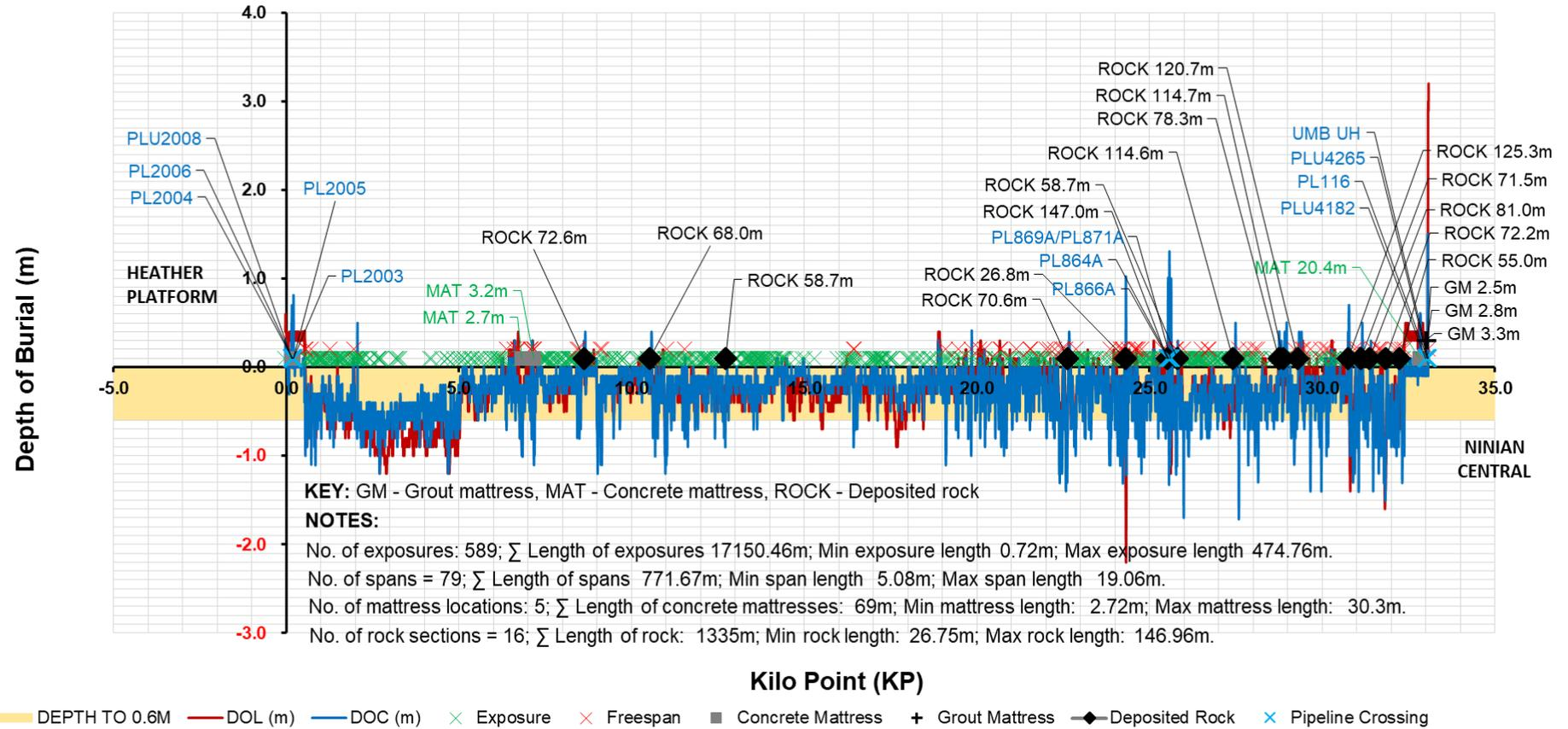
Figure 4.2.5: PL9 pipeline depth of burial profile (2012)<sup>4</sup>
