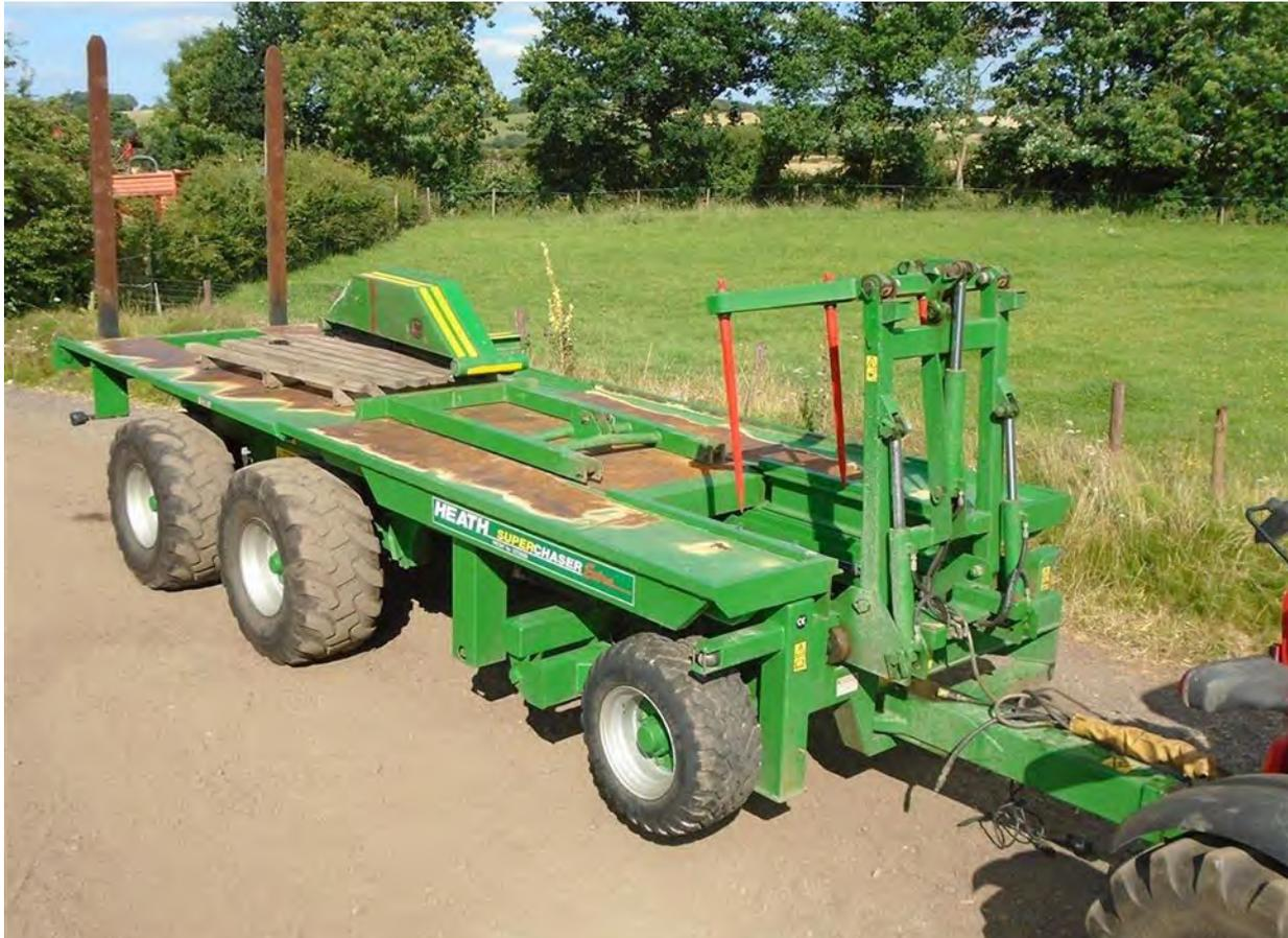
Figure 6: A bale chaser similar to that involved in the collision (courtesy of Heath Engineering).
