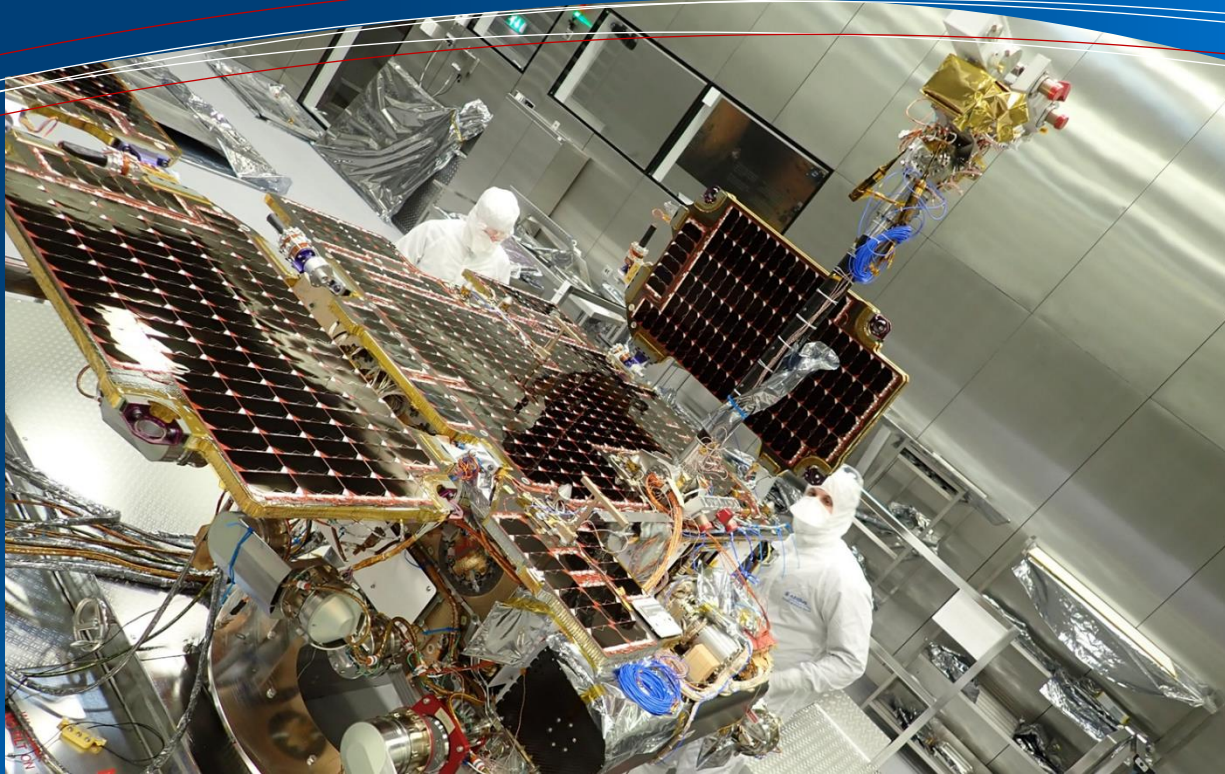
Rosalind Franklin being integrated in the Bio-Clean Facility at Airbus in Stevenage
