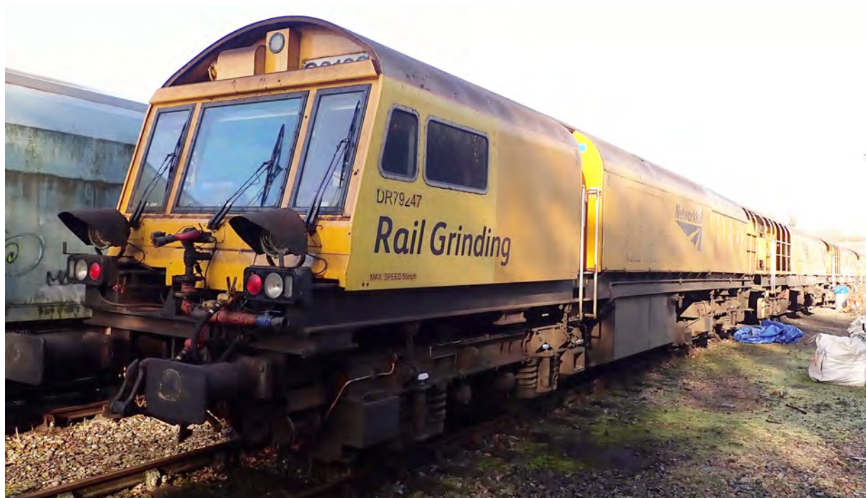
Figure 4: Rail grinding train similar to C2101
