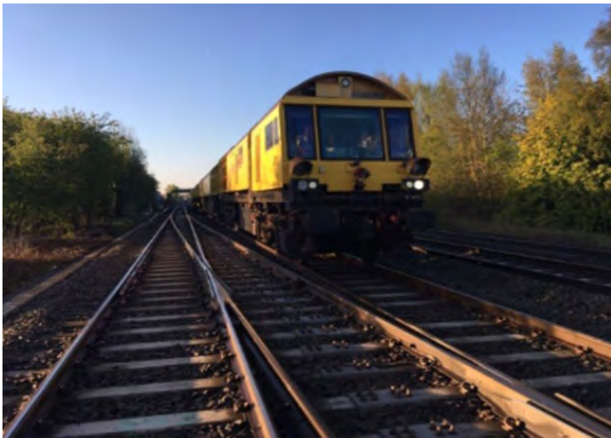
Figure 7: Stopping point of the train after the incident, showing the crossover used by train 5P01 from the down slow to the up slow line (Network Rail)
