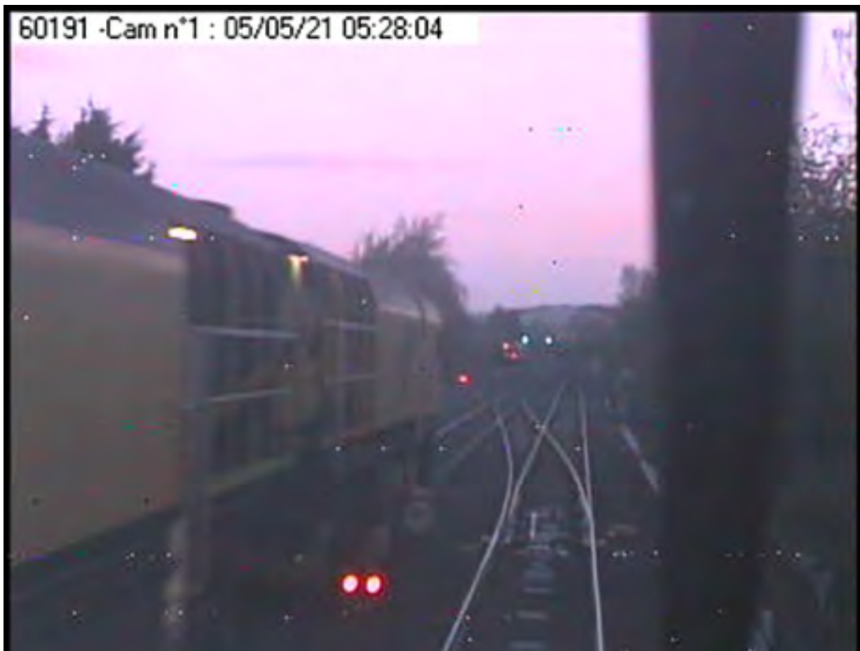
Figure 2: Still image from the rearward facing closed-circuit television (CCTV) of train 5P01 having just crossed over from the up fast line to the up slow line, across the path of train 6Z08; image shows the leading end of rail grinding train 6Z08 (left) shortly before it came to a stop on the down slow line (East Midlands Railway)
