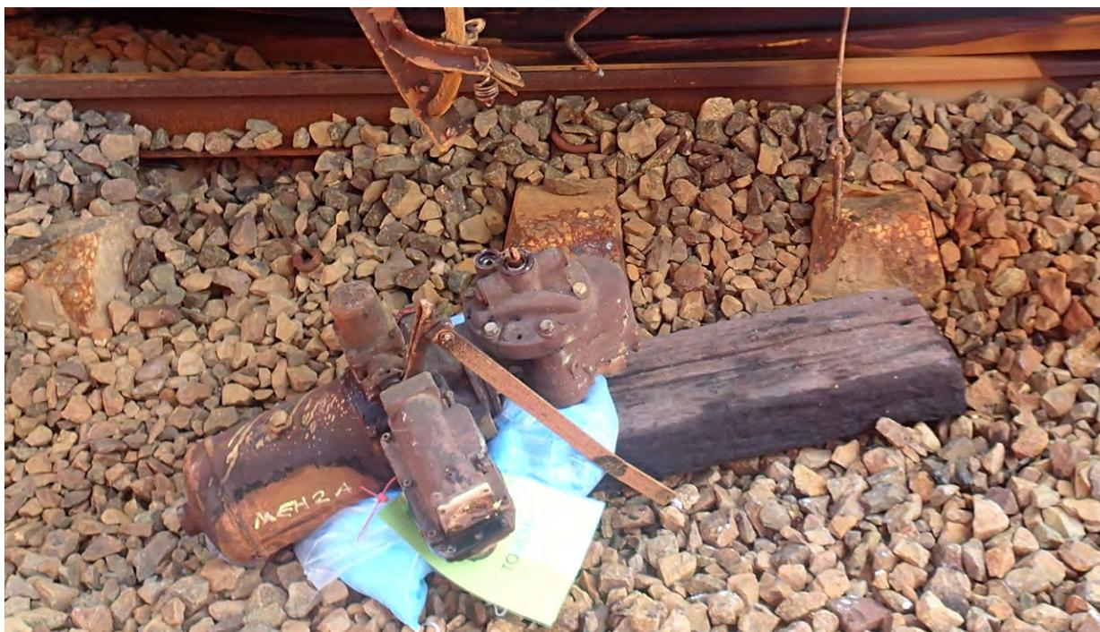
Figure 20: The brake group from Wagon GERS 89005 as found after the accident
