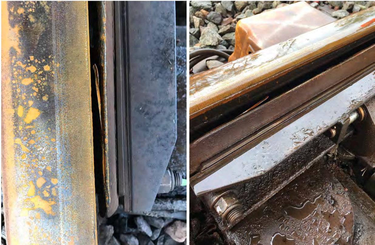
Figure 17: Damage to the switch tip of points 997A
