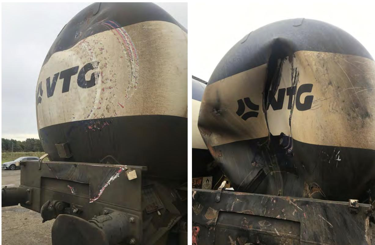
Figure 31: (left) VTG wagon (incident wagon 7) with raised buffer override protection beams which mitigated against further damage occurring and (right) wagon (incident wagon 6) that derailed, showing impact damage at high level where override protection could not prevent override and puncturing.
