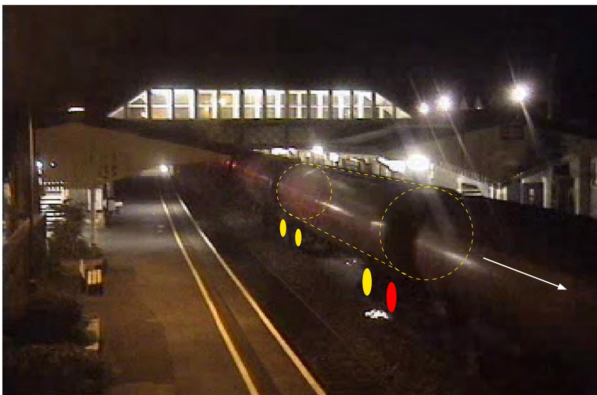
Figure 7: Station CCTV image showing train 6A11 passing through Llanelli station with sparks emanating from the front axle of wagon GERS 89005
