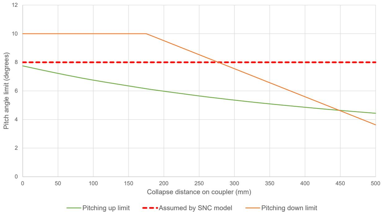
Figure 12: Graph showing how the pitch limits change as the inter-vehicle coupler collapses<sup>12</sup>
