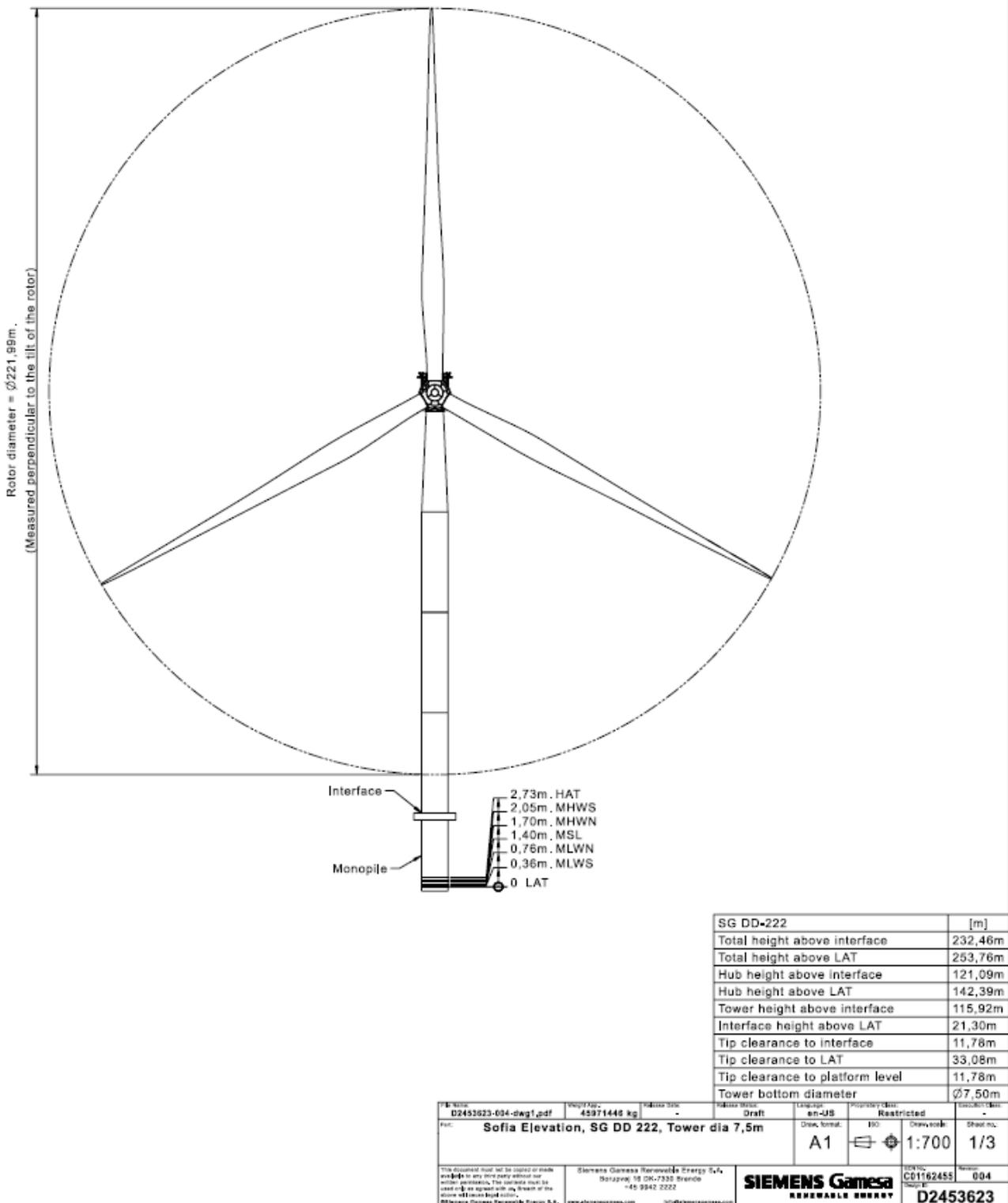
Figure 3.1: WTG Schematic
