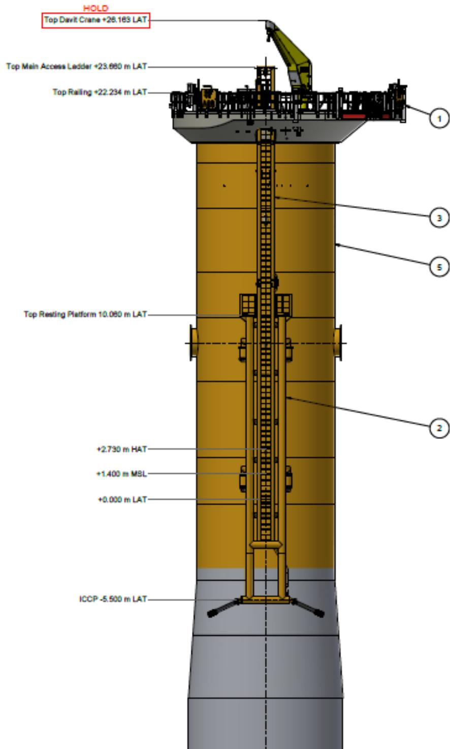
Figure 3.2: Indicative Foundation Schematic
