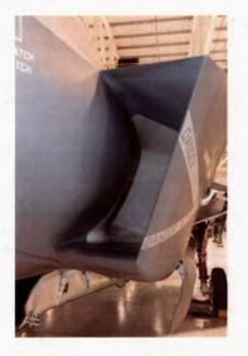
Figure 1.4.9 – Intake blank positioned in the intake, but not externally visible.
