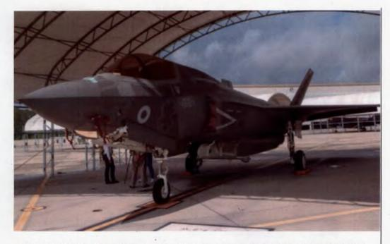
Figure 1.3.8 – Locally acquired intake plugs in a UK F-35B at MCAS Beaufort.
