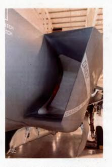
Figure 1.4.8 – Intake blank positioned in the intake.
