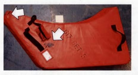
Figure 1.4.22 – BK-18 left intake blank. Arrows show black marks which were subject to chemical analysis.
