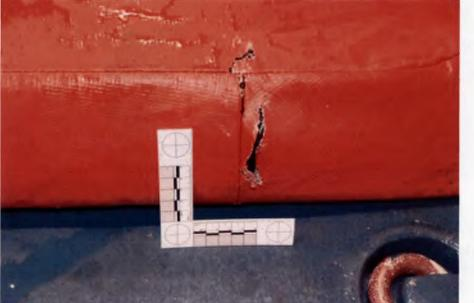
Figure 1.4.24 – Close up view of damage to BK-18 left intake blank top edge.
