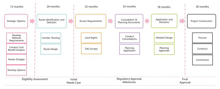
Figure 4.5 End-to-end process diagram with minimum project construction time
