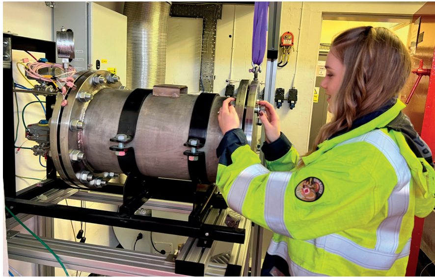
HSE scientist Gemma Howard with the equipment she designed for experiments to drive a nail into a battery sealed inside a gas-tight pressure vessel
