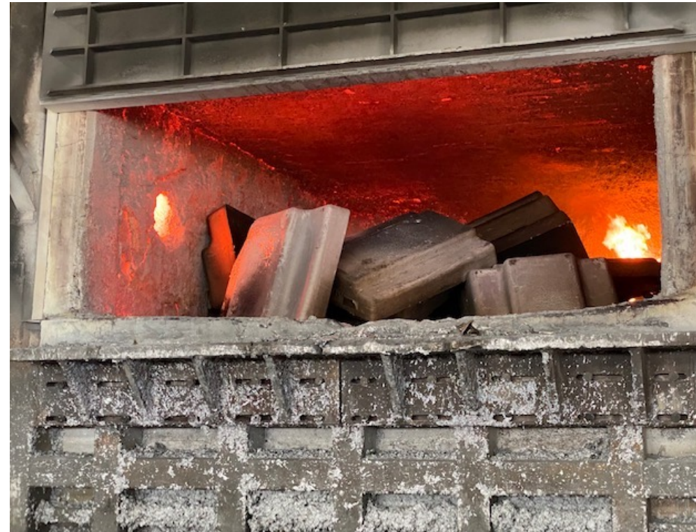
Figure 4 1: A typical solid aluminium charge for GPP Melter 3
