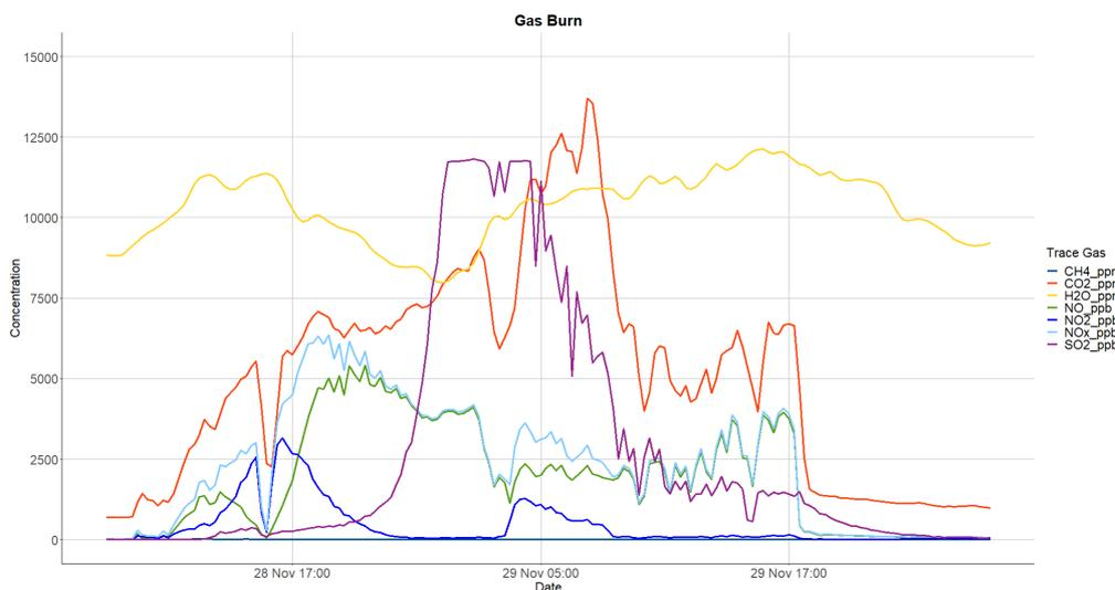
Figure 29: The emissions profiles of the natural gas trial (temperature not shown)
