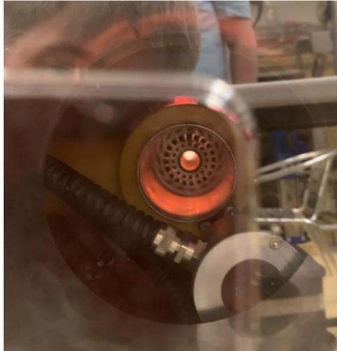
Figure 4: Hydrogen burner undergoing test firing with hydrogen in Limpsfield Lab
