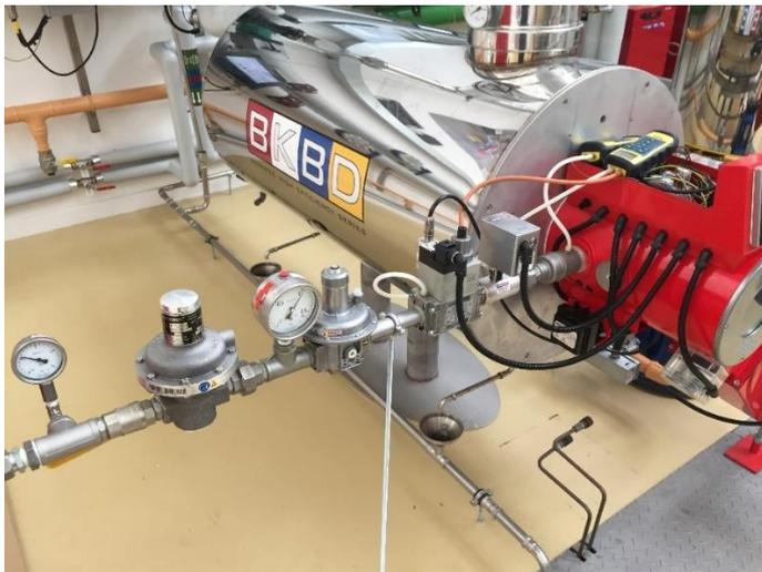
*Figure 30: Test setup for hydrogen firing (Limpsfield Lab)*
