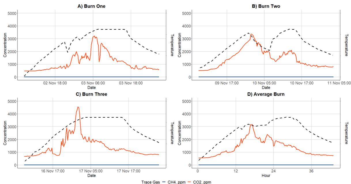
Figure 27: The CO<sub>2</sub> and CH<sub>4</sub> emissions profiles of Burn One (a), Burn Two (b), Burn Three (c) and the average Hydrogen burn (d). Temperature denoted by dashed black line
