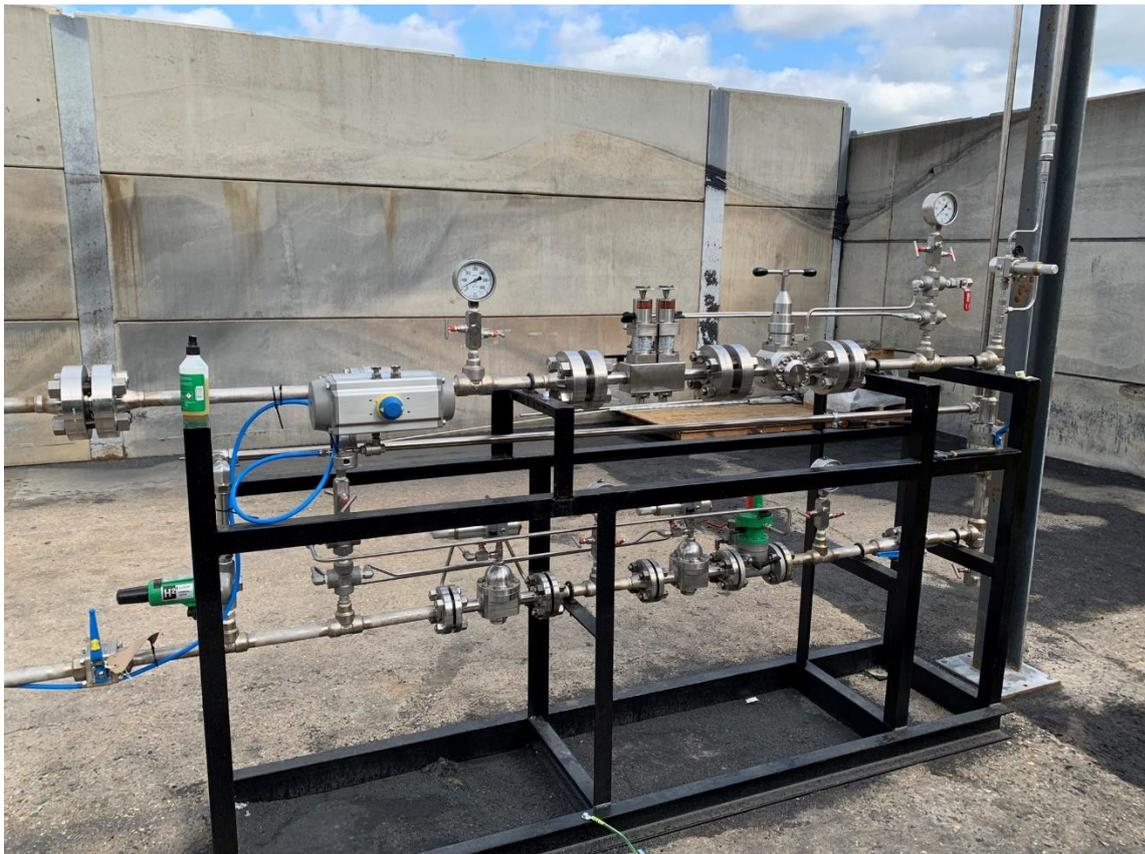
Figure 6: Hydrogen Pressure Reducing Skid
