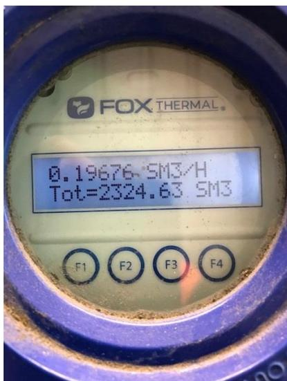
Figure 21: Close up of Fox Thermal Flow Meter (H<sub>2</sub> reading)
