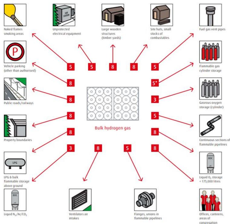
Figure 12: Minimum recommended horizontal distances for hydrogen bulk gas systems (distance in metres)
