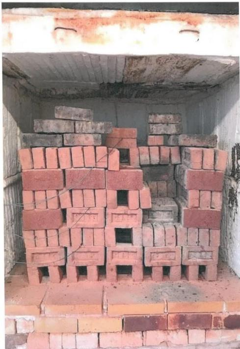
Figure 19: Hydrogen Burn 3 Bricks in Kiln
