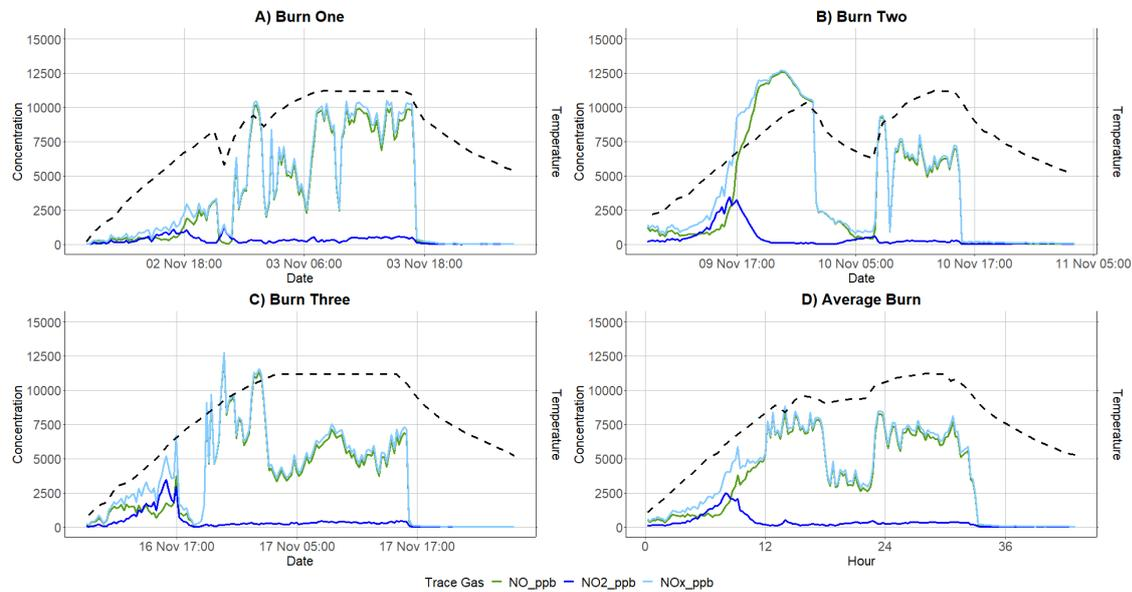
Figure 25: The NO, NO<sub>2</sub> and NO<sub>x</sub> emissions profiles of Burn One (a), Burn Two (b), Burn Three (c) and the average Hydrogen burn (d). Temperature denoted by dashed black line
