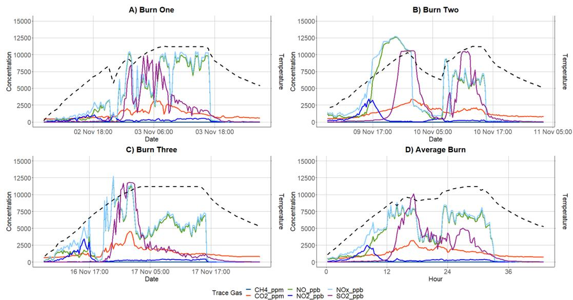
Figure 24: The emissions profiles of Burn One (a), Burn Two (b), Burn Three (c) and the average Hydrogen burn (d). Temperature denoted by dashed black line
