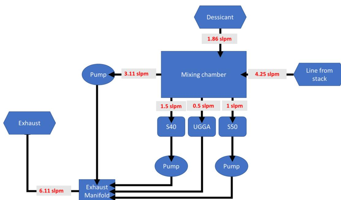
Figure 22: Diagram of sampling set up and flow rates (arrows indicate direction of flow)
