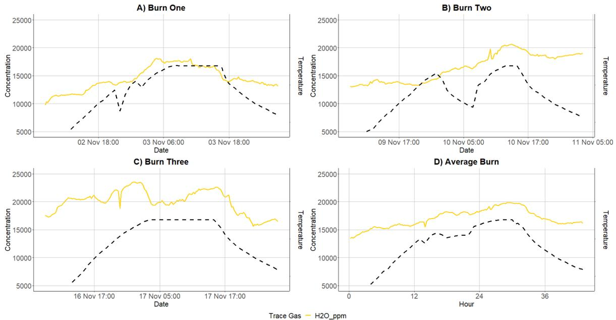
Figure 28: The H<sub>2</sub>O emissions profiles of Burn One (a), Burn Two (b), Burn Three (c) and the average Hydrogen burn (d). Temperature denoted by dashed black line
