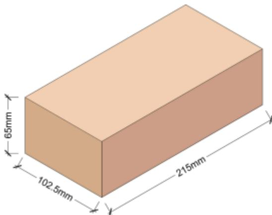
Figure 13: The most widely used work size for UK Clay bricks
