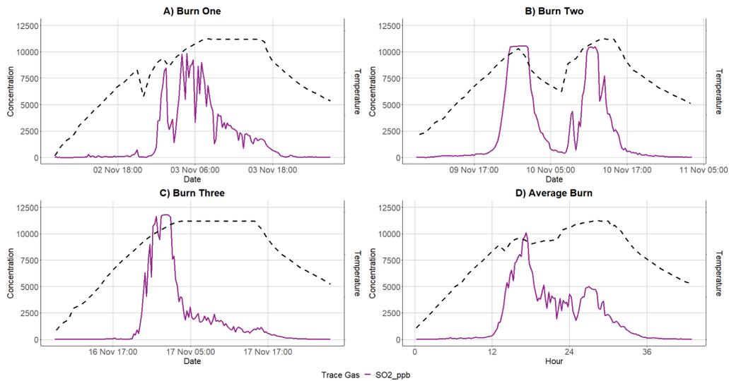
Figure 26: The SO<sub>2</sub> emissions profiles of Burn One (a), Burn Two (b), Burn Three (c) and the average Hydrogen burn (d). Temperature denoted by dashed black line
