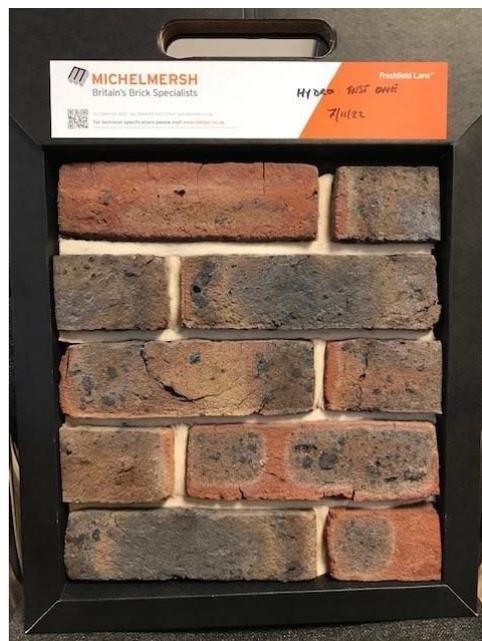
Figure 16: Hydrogen Burn 1 Test Panel
