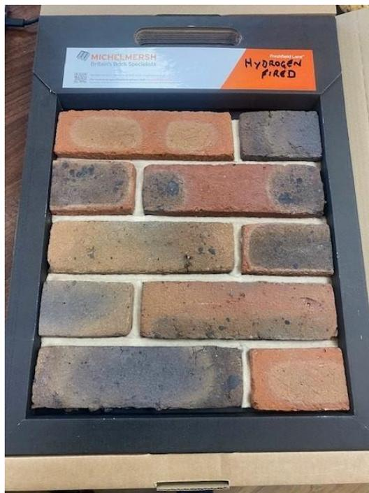
Figure 20: Hydrogen Trial 3 Test Panel
