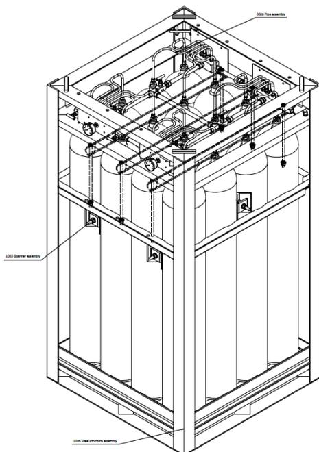
Figure 8: Hydrogen Manifold Cylinder Pack (MCP)
