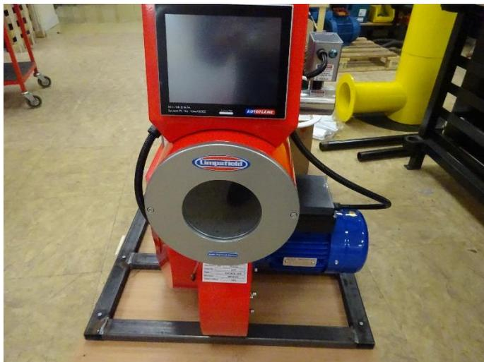
Figure 32: Limpsfield Hydrogen Ready Burner
