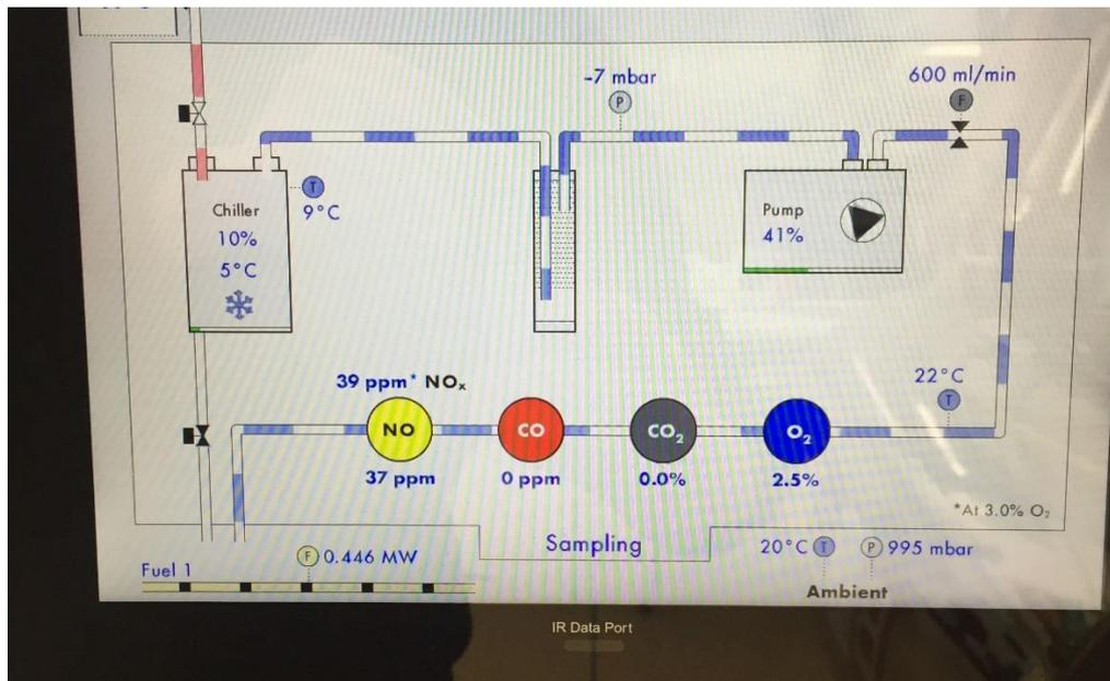
Figure 31: Low NO<sub>x</sub> achieved during bench tests
