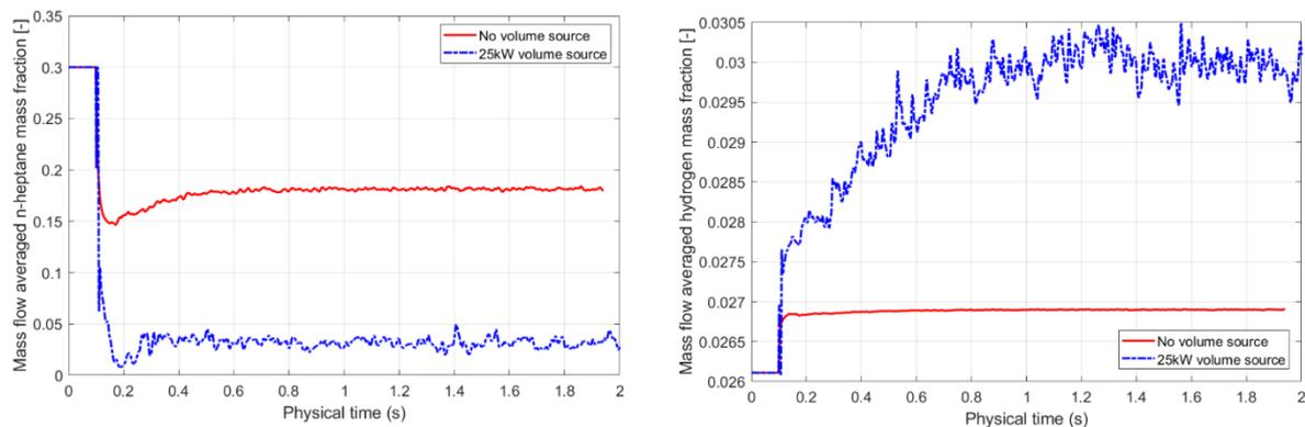
Figure 2: The distribution of key mass flow averaged quantities across all syngas flow outlets with and without the triboplasma volume source: *n*-heptane mass fraction, which represented tars in the simulation (left) and hydrogen mass fraction (right).
