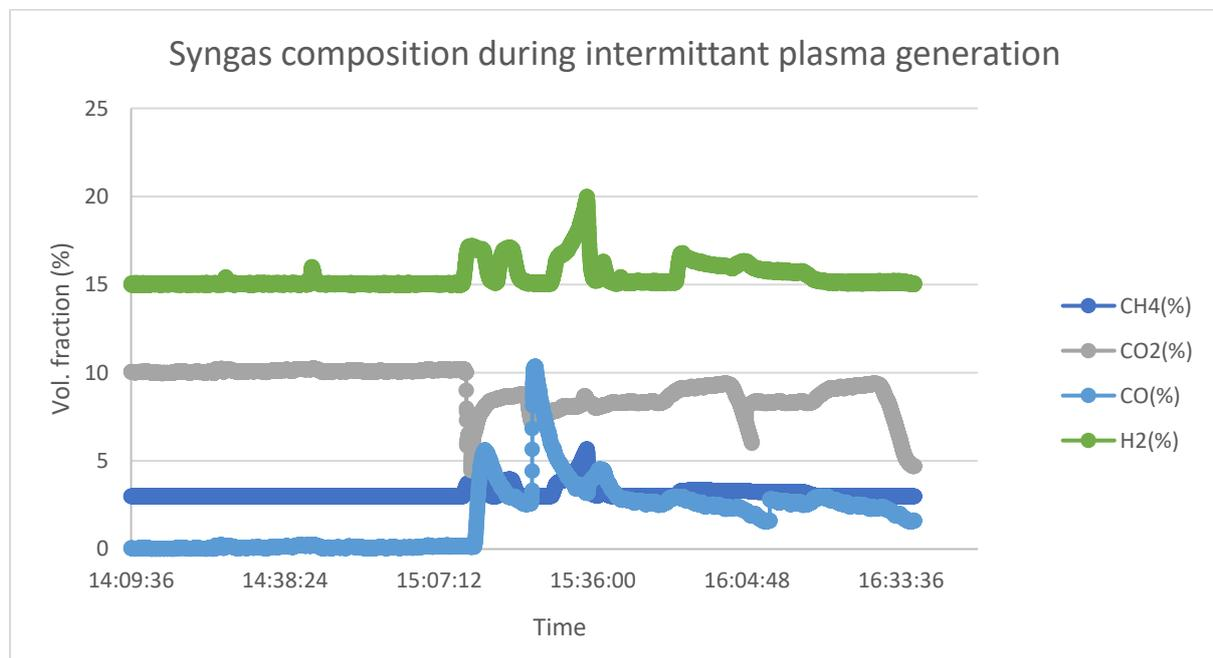
Figure 3: Syngas analysis from tests at UCL, in which a gas mixture of H<sub>2</sub>, CO<sub>2</sub>, Steam, CH<sub>4</sub> and vaporised C<sub>12</sub> hydrocarbons are exposed to intermittent plasma discharges
