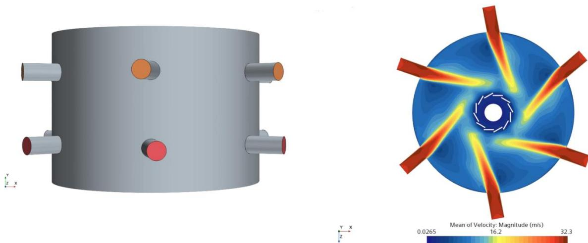
Figure 1: Schematic of reformer vessel used in the full-scale reacting flow calculations, where inlets are highlighted in red and outlets are highlighted in orange (left) and the CFD solution of in the reformer inlet plane coloured by mean velocity magnitude (right).
