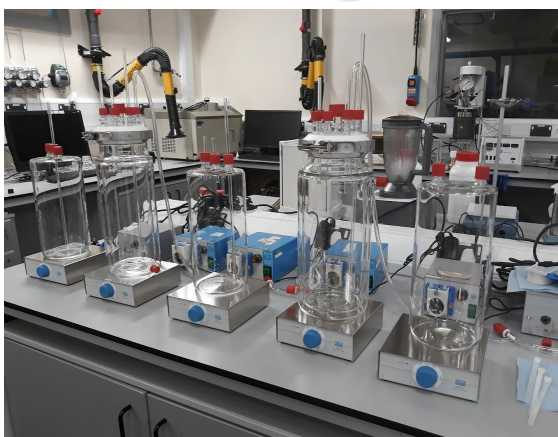
Figure C.1 DF and AD stages: Experimental set-up for the lab-prototype.
