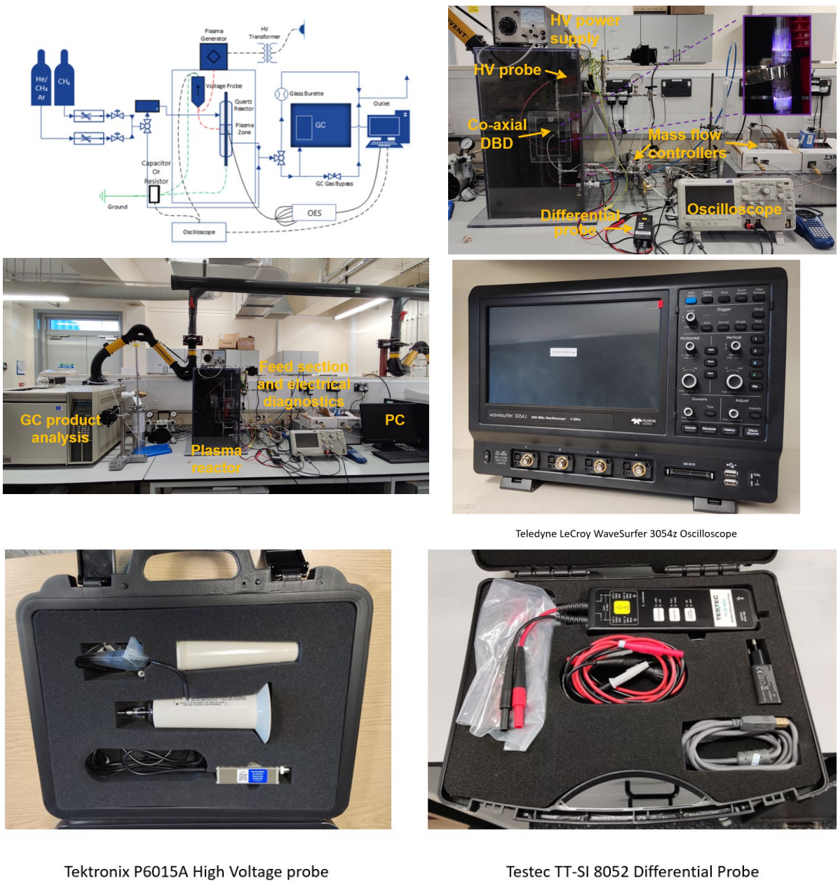
Figure C.3. PR stage: Experimental set-up of the lab prototype
