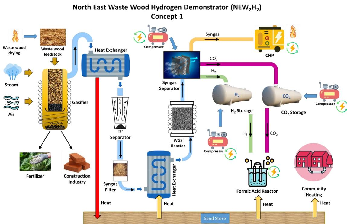
Figure 3: Concept 1 Pictorial Diagram
