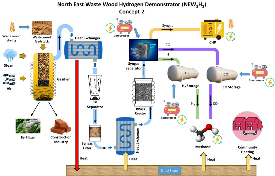
Figure 4: Concept 2 Pictorial Diagram
