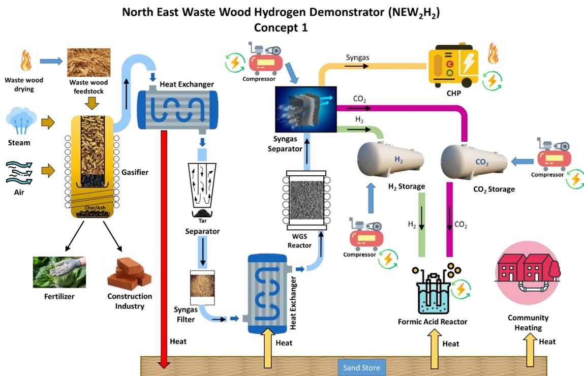
Figure 3: Concept 1 Pictorial Diagram
