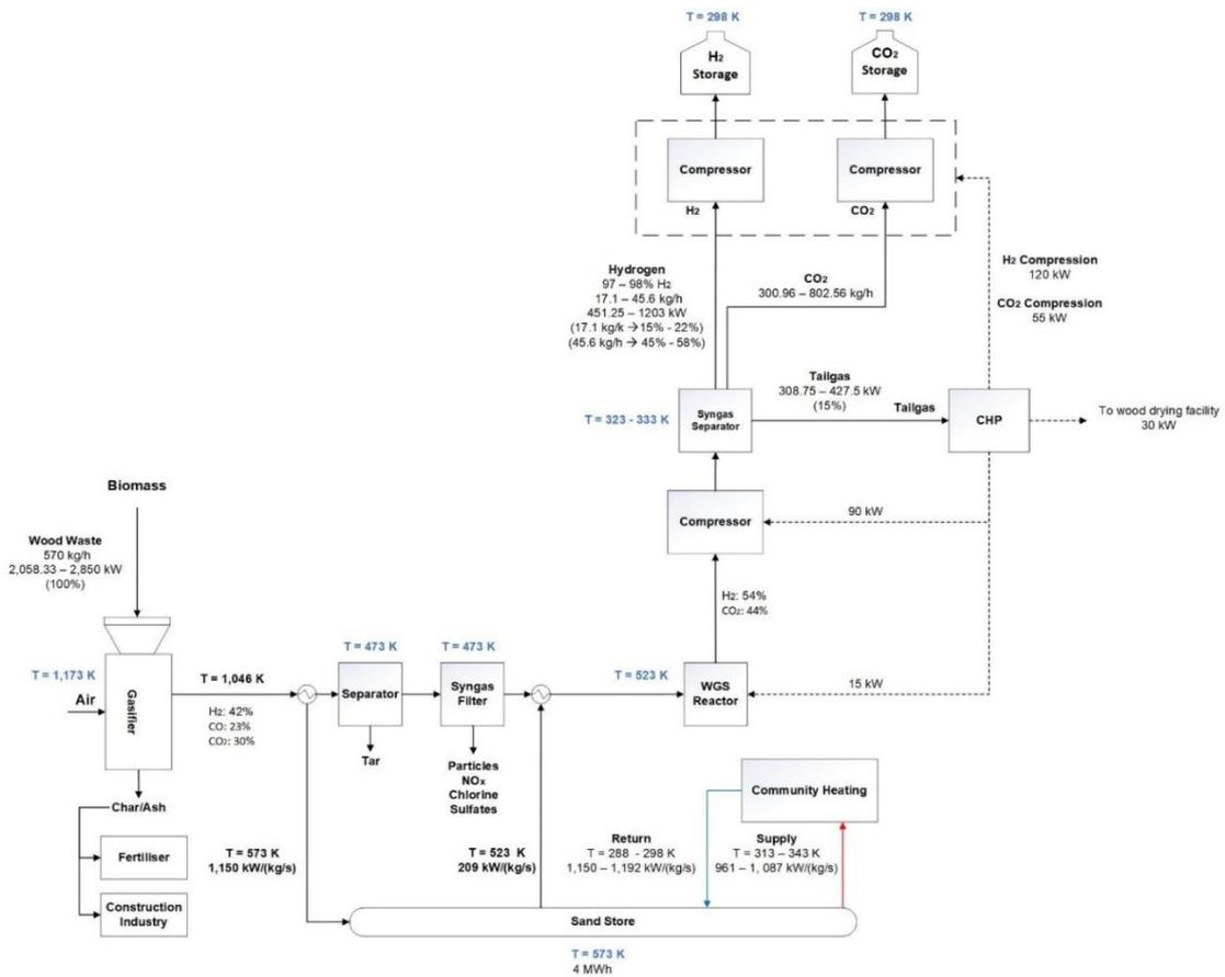
Figure 7: Heat and Mass Balance Diagram for the Proposed NEW<sub>2</sub>H<sub>2</sub> Concept 3 Installation
