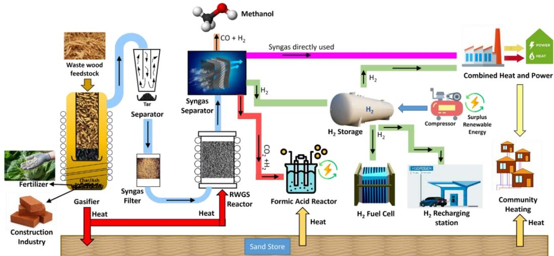
Figure 1: Pictorial Diagram of Original Concept as Presented in the Proposal
