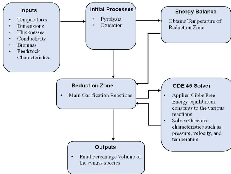
Figure 10: Schematic Diagram of the Gasification Code Structure
