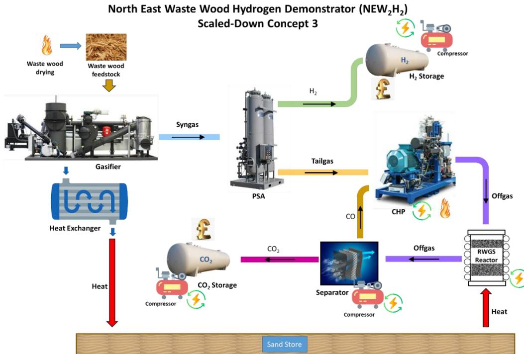
Figure 12: Scaled-Down Concept 3 Pictorial Diagram
