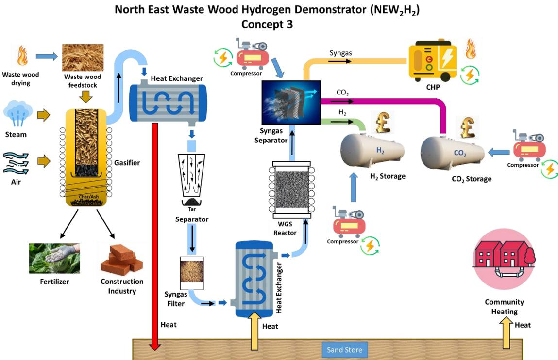
Figure 5: Concept 3 Pictorial Diagram
