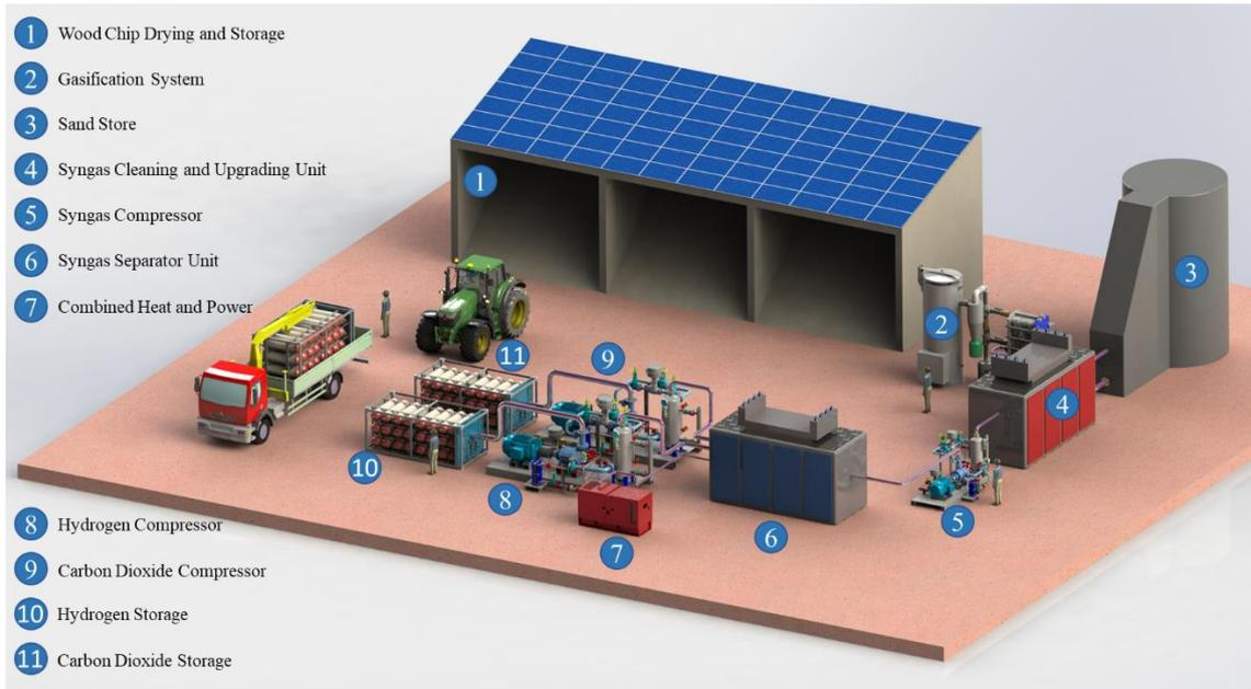
Figure 6: Digital Representation of the Layout for NEW<sub>2</sub>H<sub>2</sub> Concept 3
