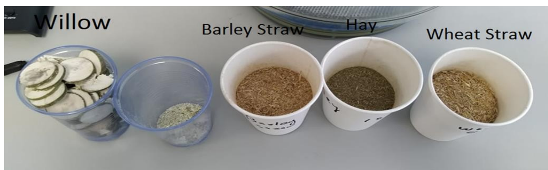
Figure 2 The samples of feedstocks oven dried and ground in the Newcastle University laboratory sourced from Cockle Park Farm, Morpeth
