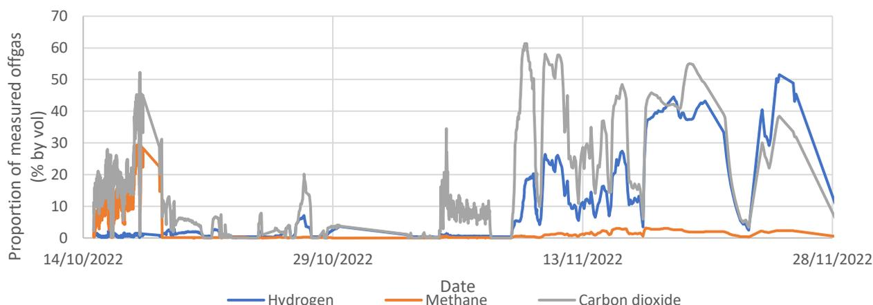
Figure 11: Hydrogen % in off gas during the test period.
