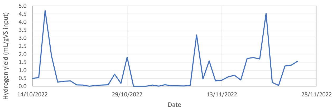
Figure 10: Hydrogen production during the test period - yield per g of volatile solids (VS).
