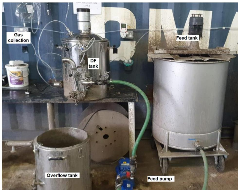
Figure 8: The dark fermentation process in 'continuous' setup mode.
