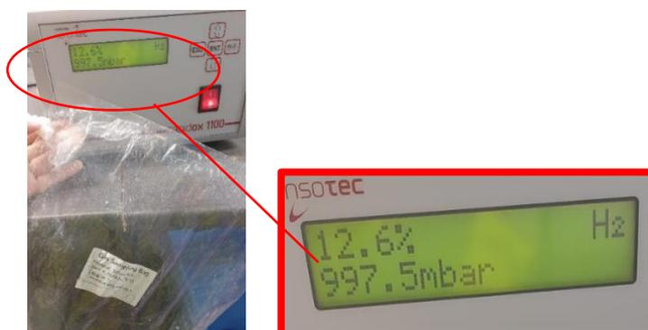
Figure 3: Gas analysis during the functional test.
