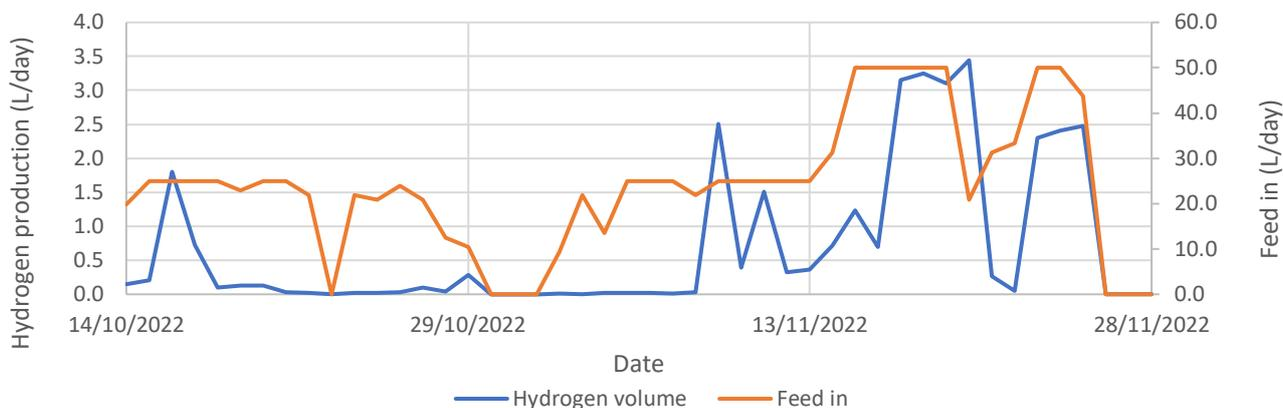
Figure 9: Hydrogen production during the test period - comparison of production rate vs feed rate.
