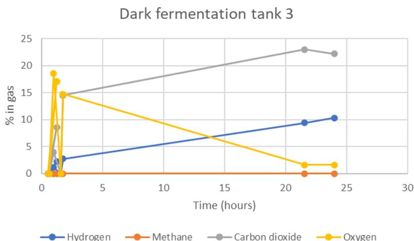
Figure 14: Hydrogen production in run 2, fermenter 3.
