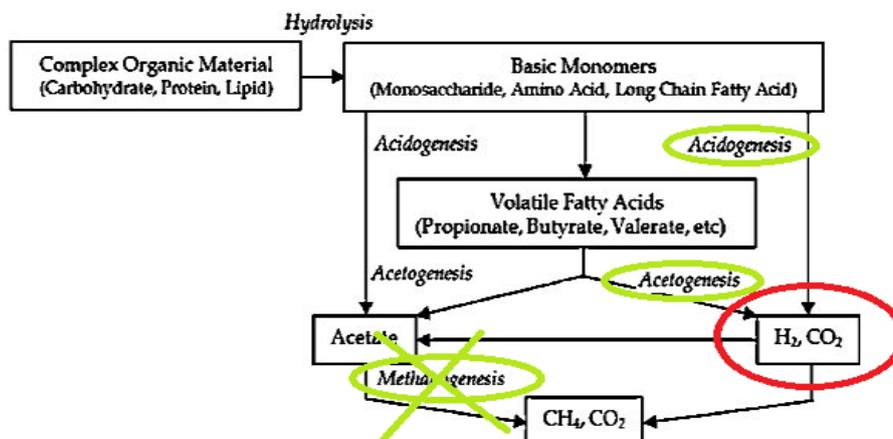
Figure 1: The process of anaerobic digestion with process adjustments to favour dark fermentation.
