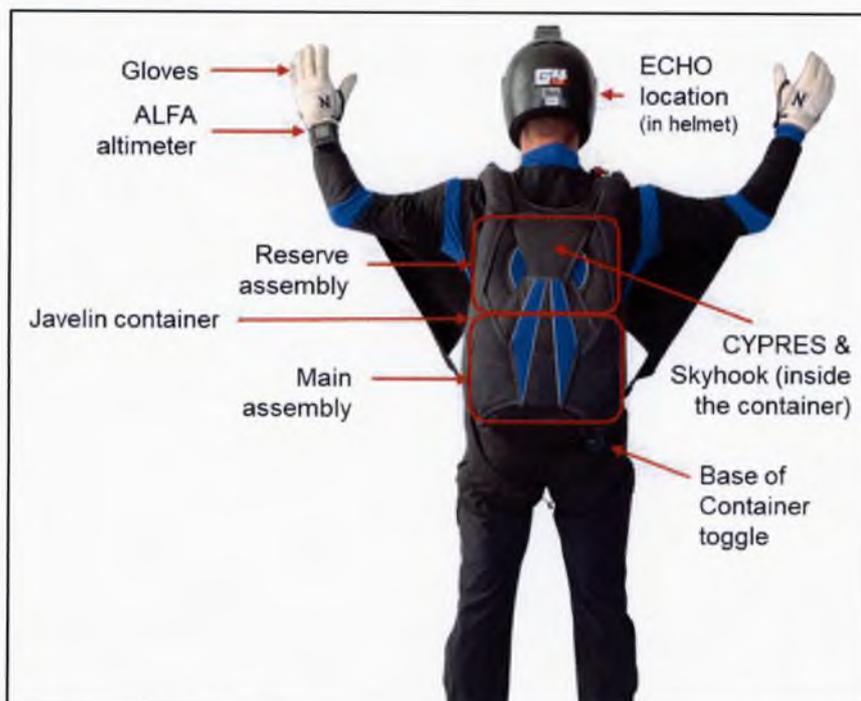
Figure 1.3.A.2 – Equipment and ancillaries, rear view.
