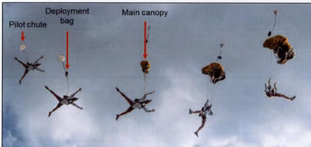
Figure 1.3.A.10 – Main canopy deployment.<sup>38</sup>
