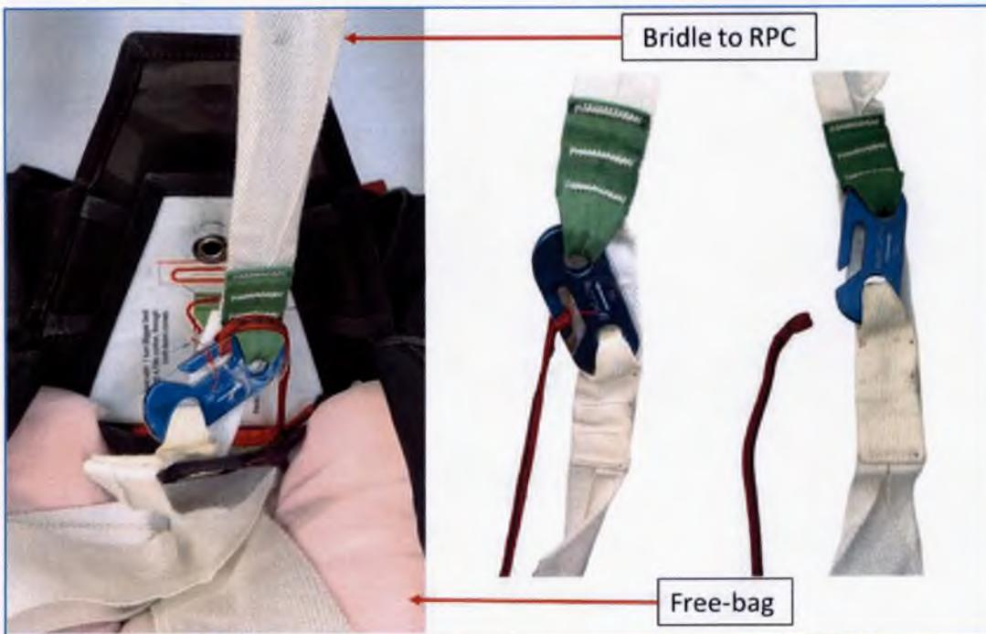
Figure 1.3.A.33 – Skyhook operation for non-main canopy malfunction.<sup>62</sup>
