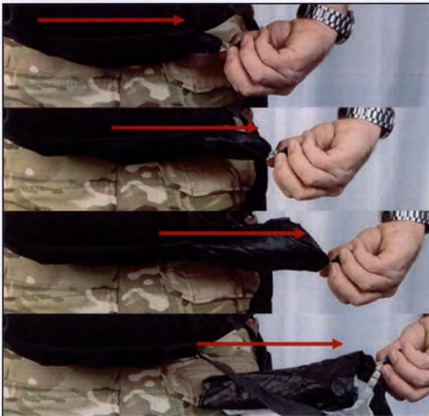
Figure 1.3.A.8 – Main pilot chute deployment.
