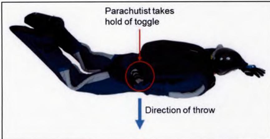
Figure 1.3.A.7 – Main pilot chute deployment position.<sup>37</sup>
