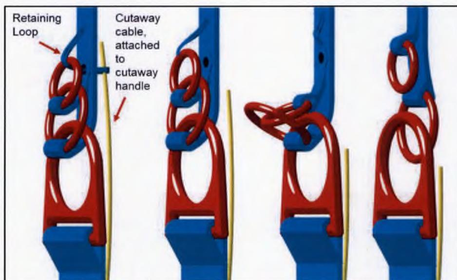
Figure 1.3.A.12 – 3-ring release operation.<sup>39</sup>
