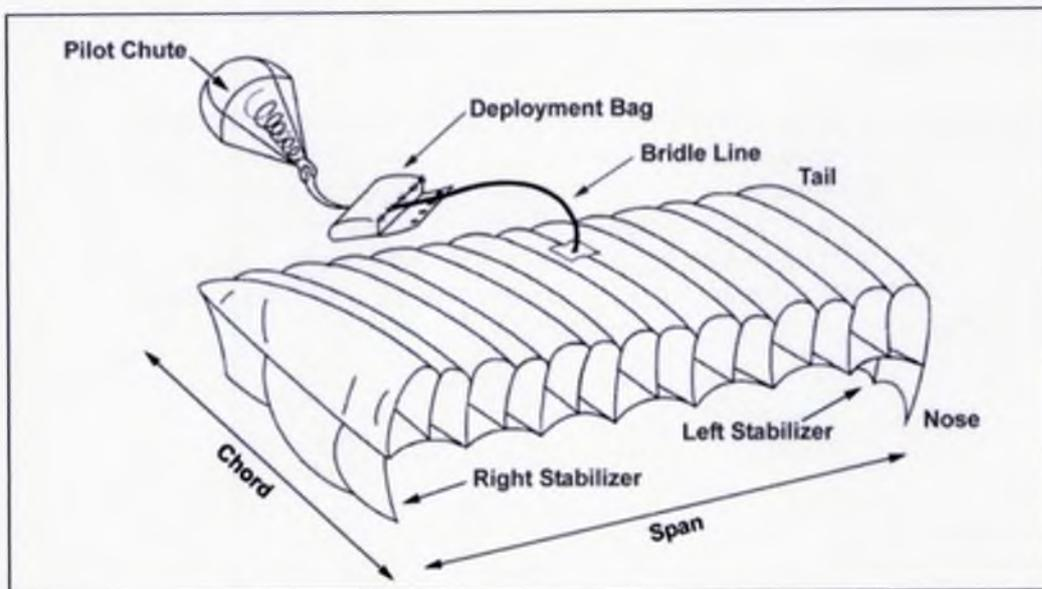
Figure 1.3.A.26 – Ram-air external design.<sup>52</sup>
