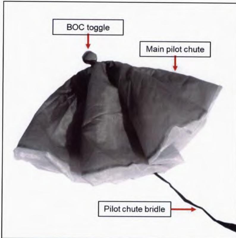
Figure 1.3.A.5 – Main pilot chute.<sup>36</sup>
