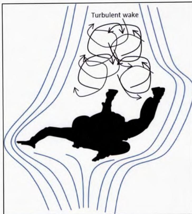
**Figure 1.4.27 – Parachutist turbulent wake.**
