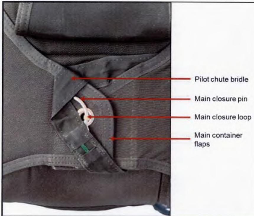
Figure 1.3.A.9 – Main container closure flaps and pin.
