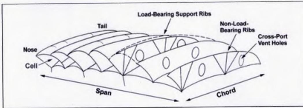
Figure 1.3.A.25 – Ram-air canopy internal design.<sup>51</sup>
