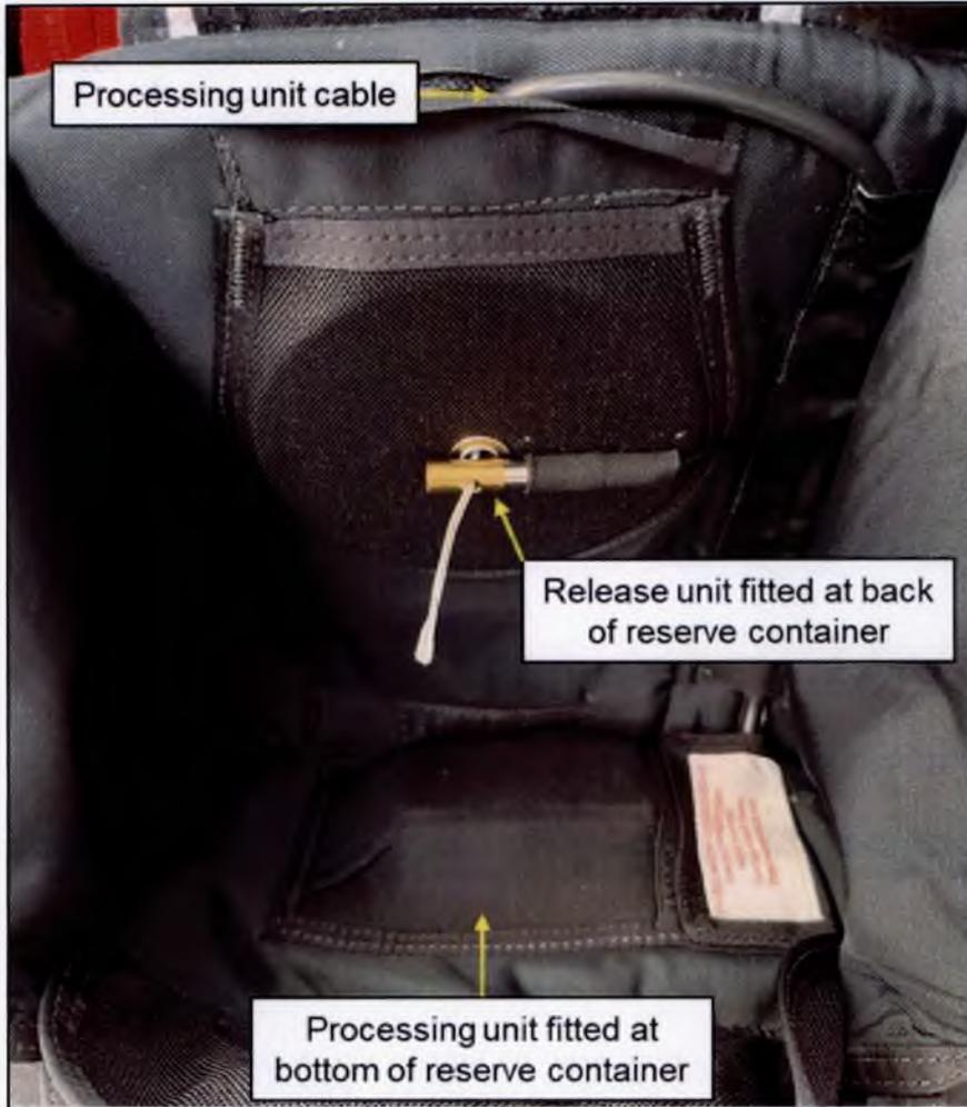
Figure 1.3.A.38 – CYPRES release and processing units.
