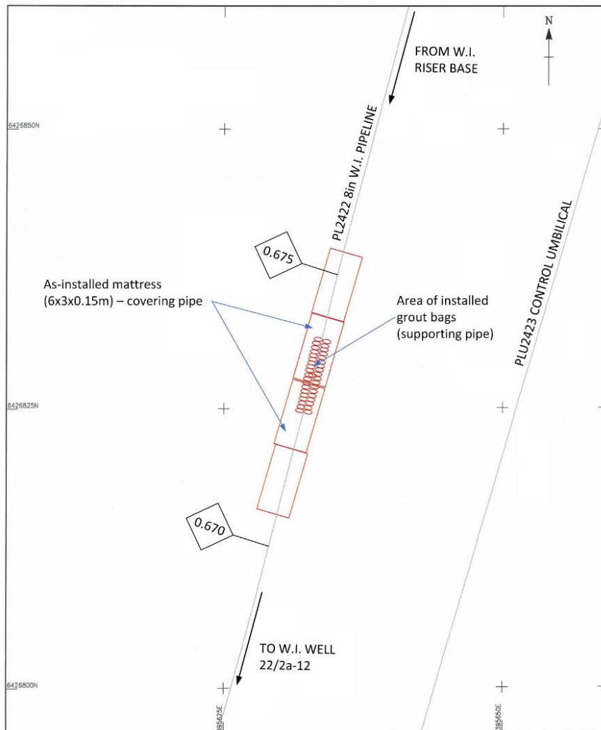
Figure 2.4.5: Span rectification work on PL2422 in 2010
