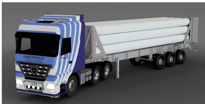
Figure 3: Example of hydrogen tube trailer.
